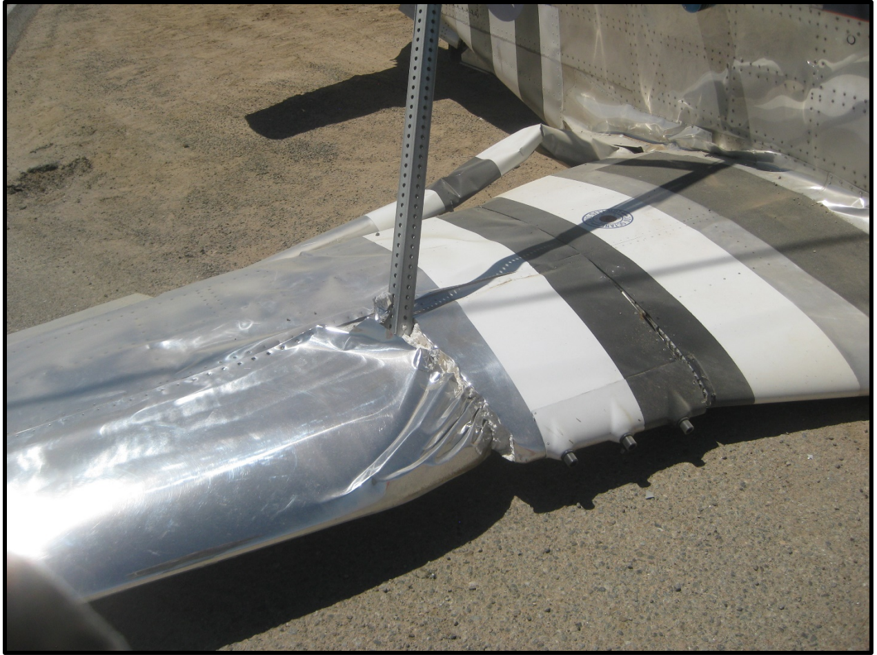
Figure 2: Right Wing Damage.
