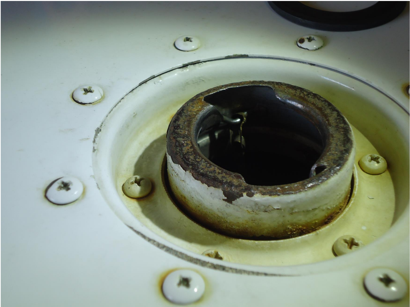
FAA Photo 4 – Right Wing Fuel Tank Filler Neck
