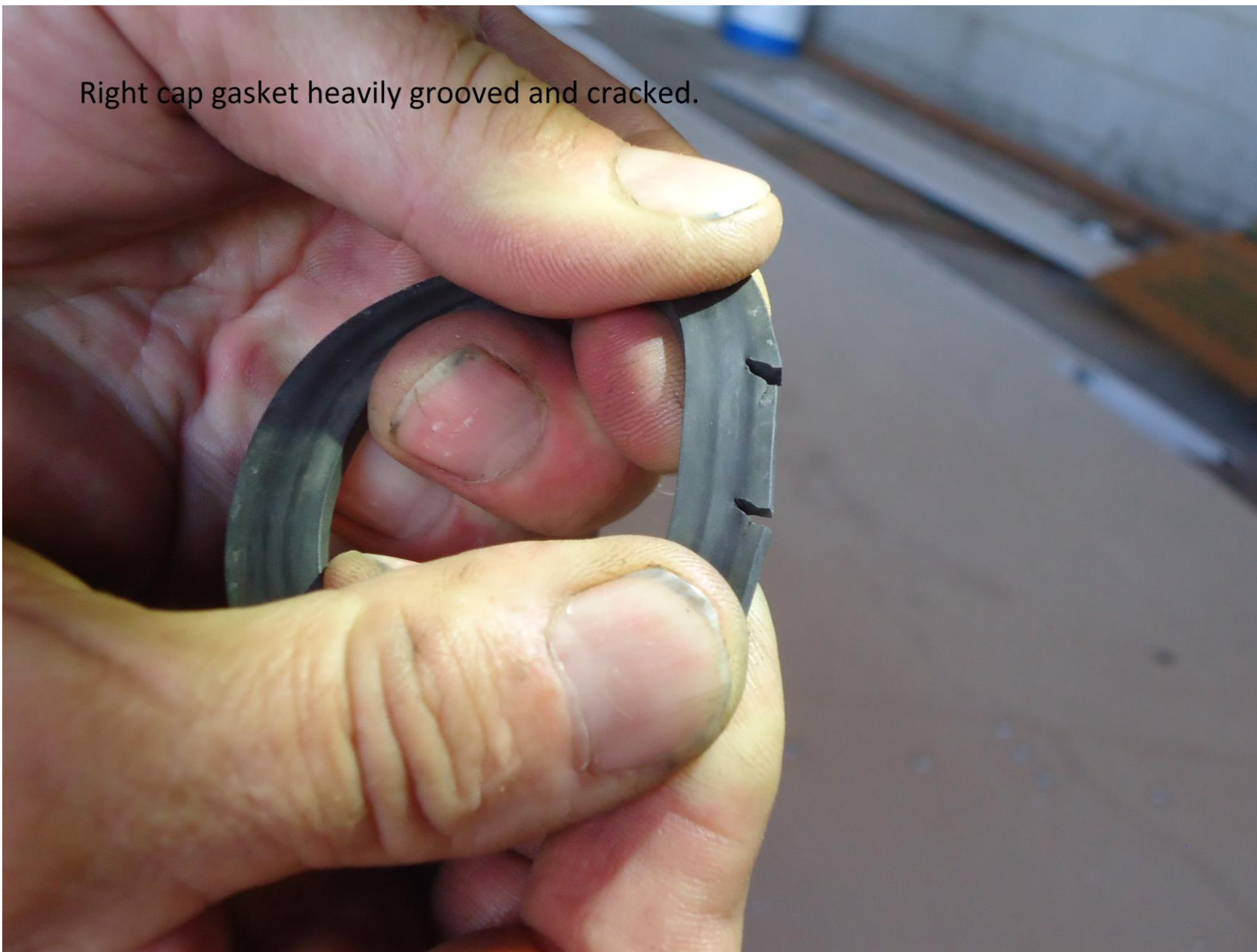
FAA Photo 3 – Right Wing Tank Cap Seal
