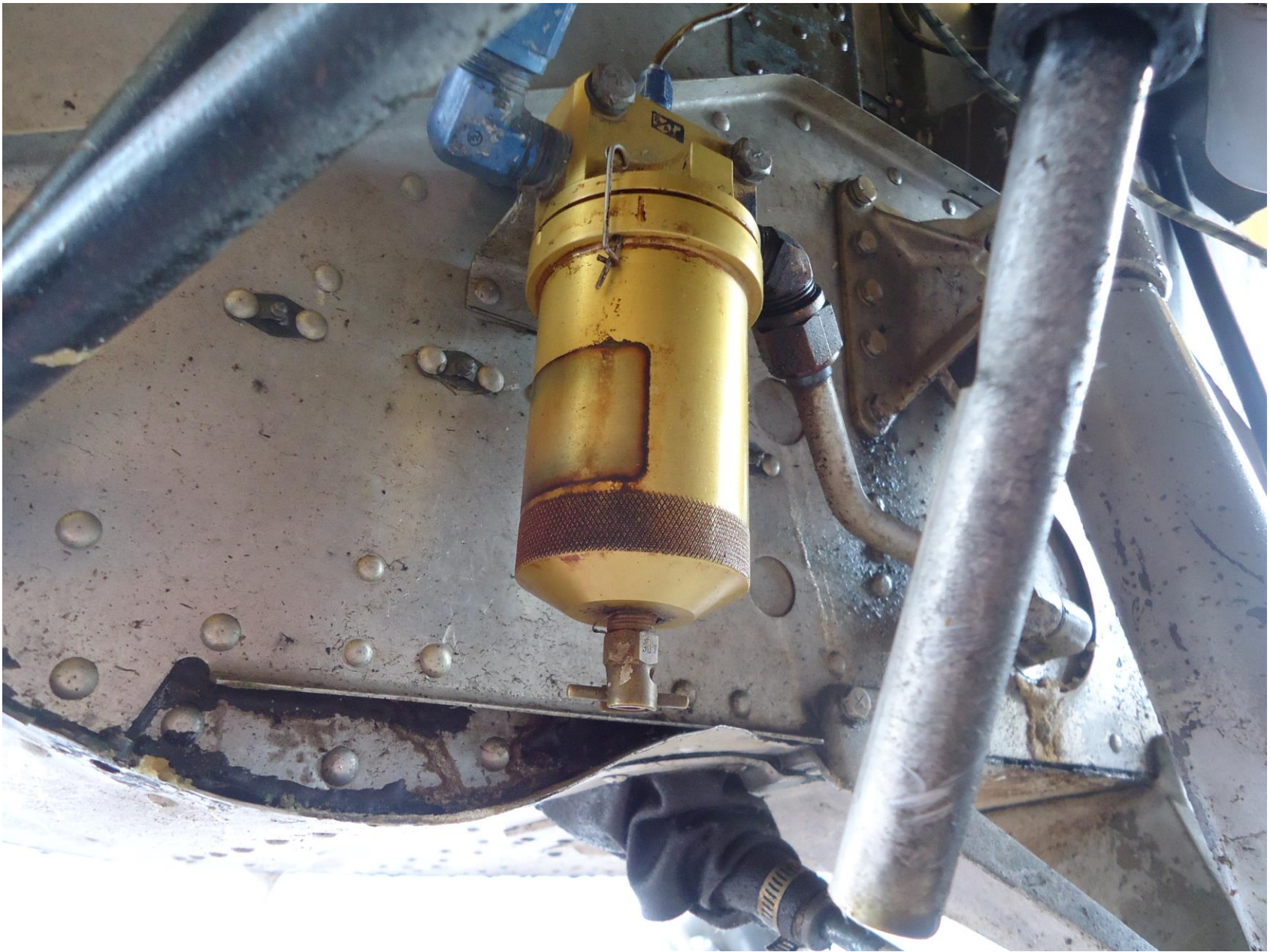
FAA Photo 5 - Gascolator
