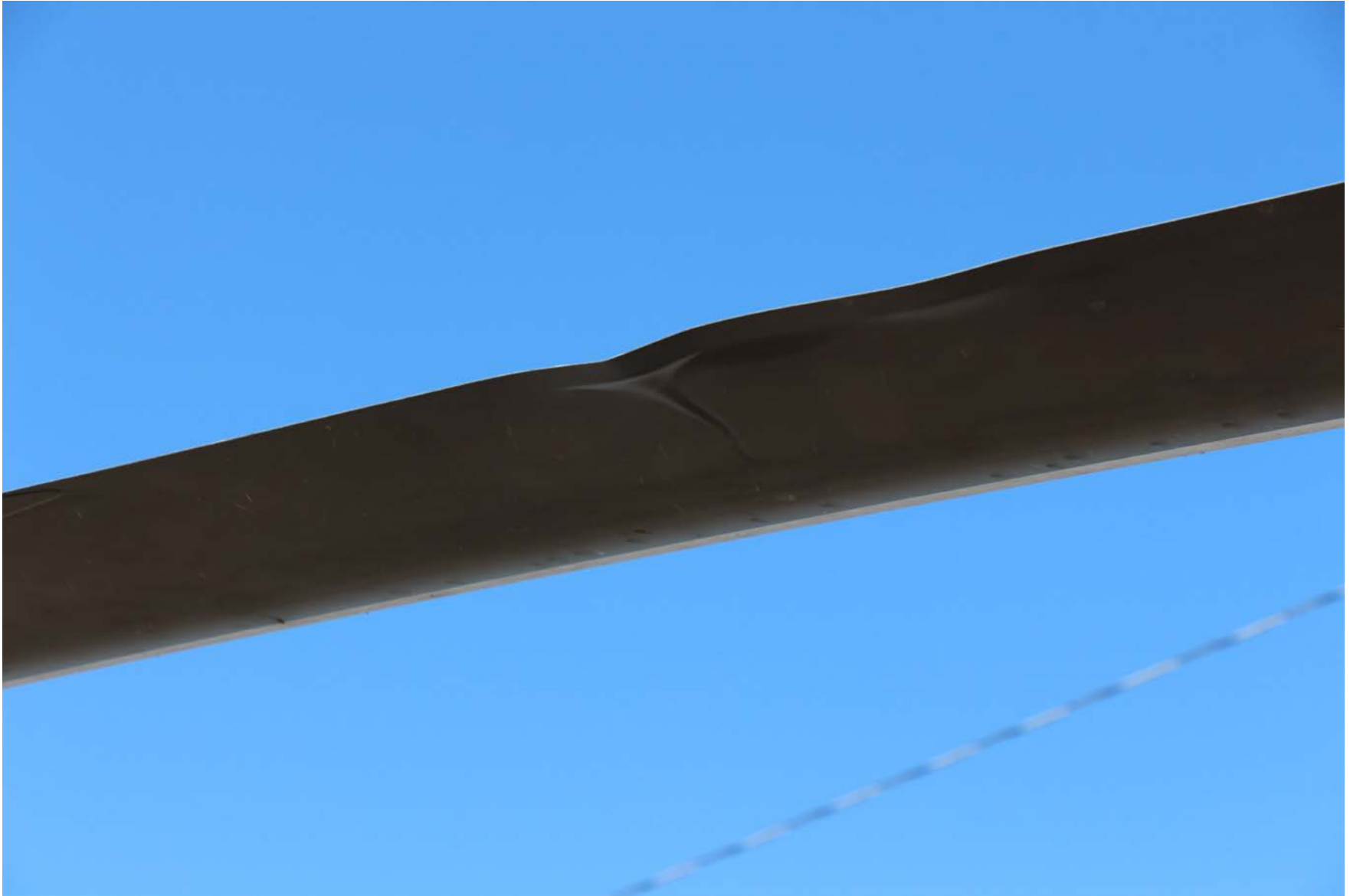
Photo 4 – View of Trailing Edge Damage to Main Rotor Blade
