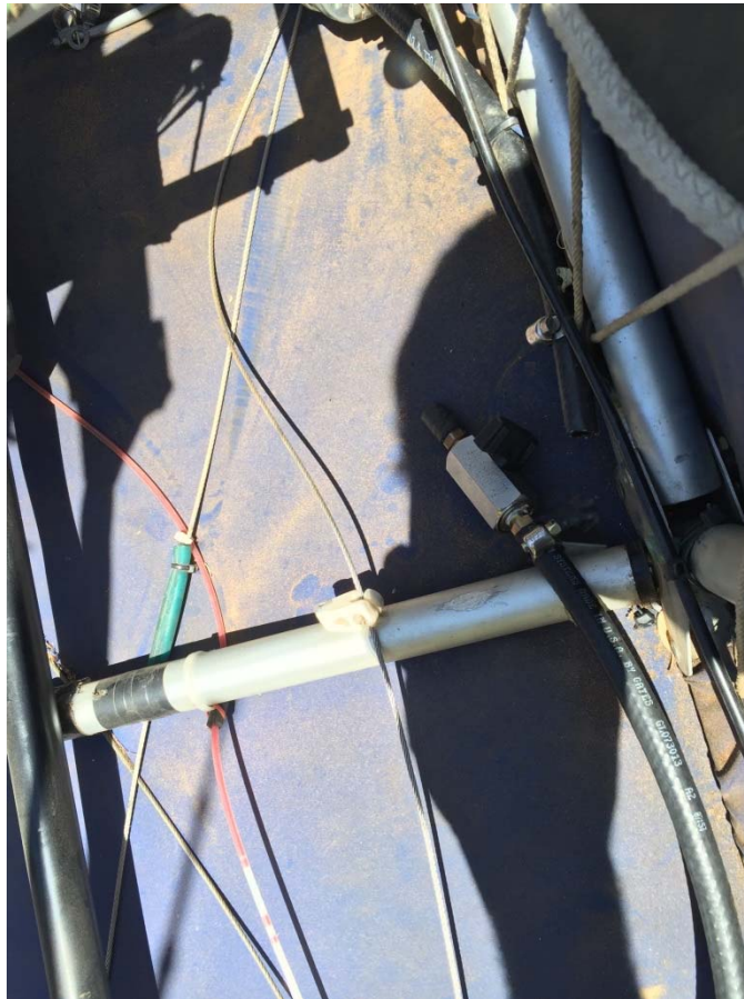
Photo 3: Fuel line and shut off valve and wear mark on the airframe tube.
