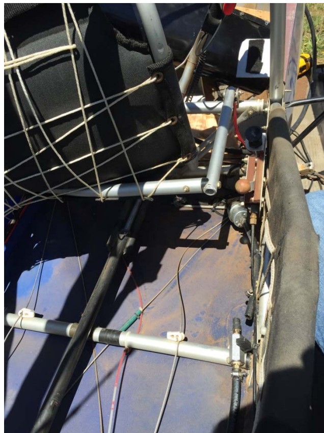
Photo 2: Seat assembly and fuel line (side side).
