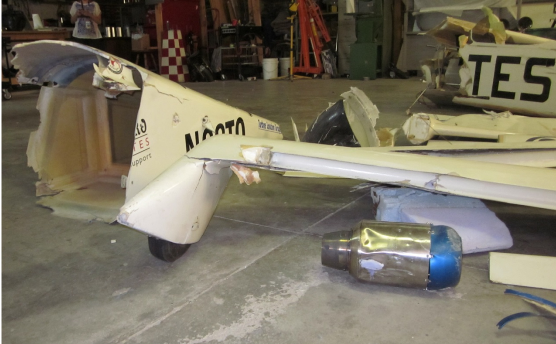
Figure 8 - Left Canard, Fuselage, and Liberated Engine
