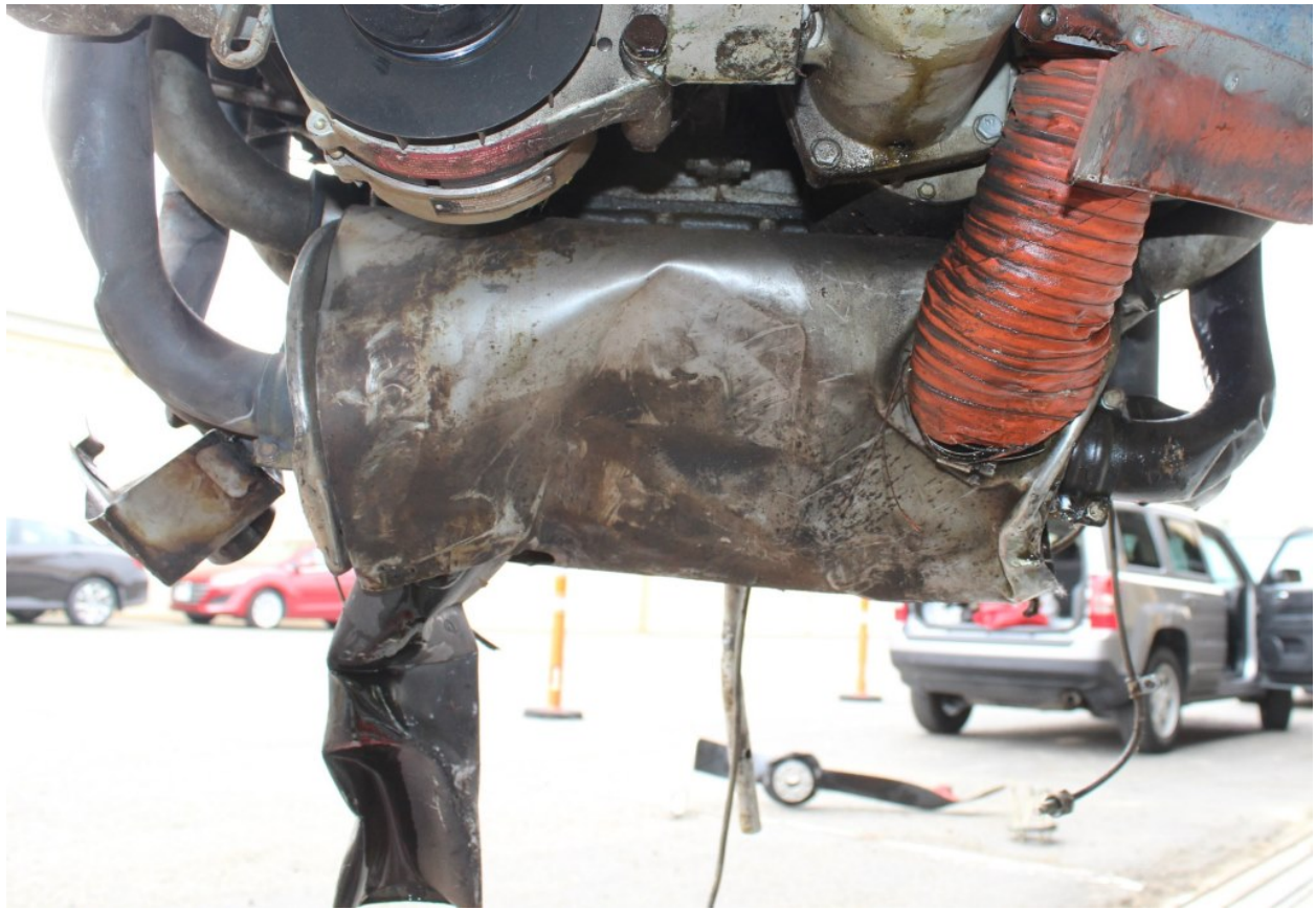
Figure 32 -Exhaust Pipes and Muffler
