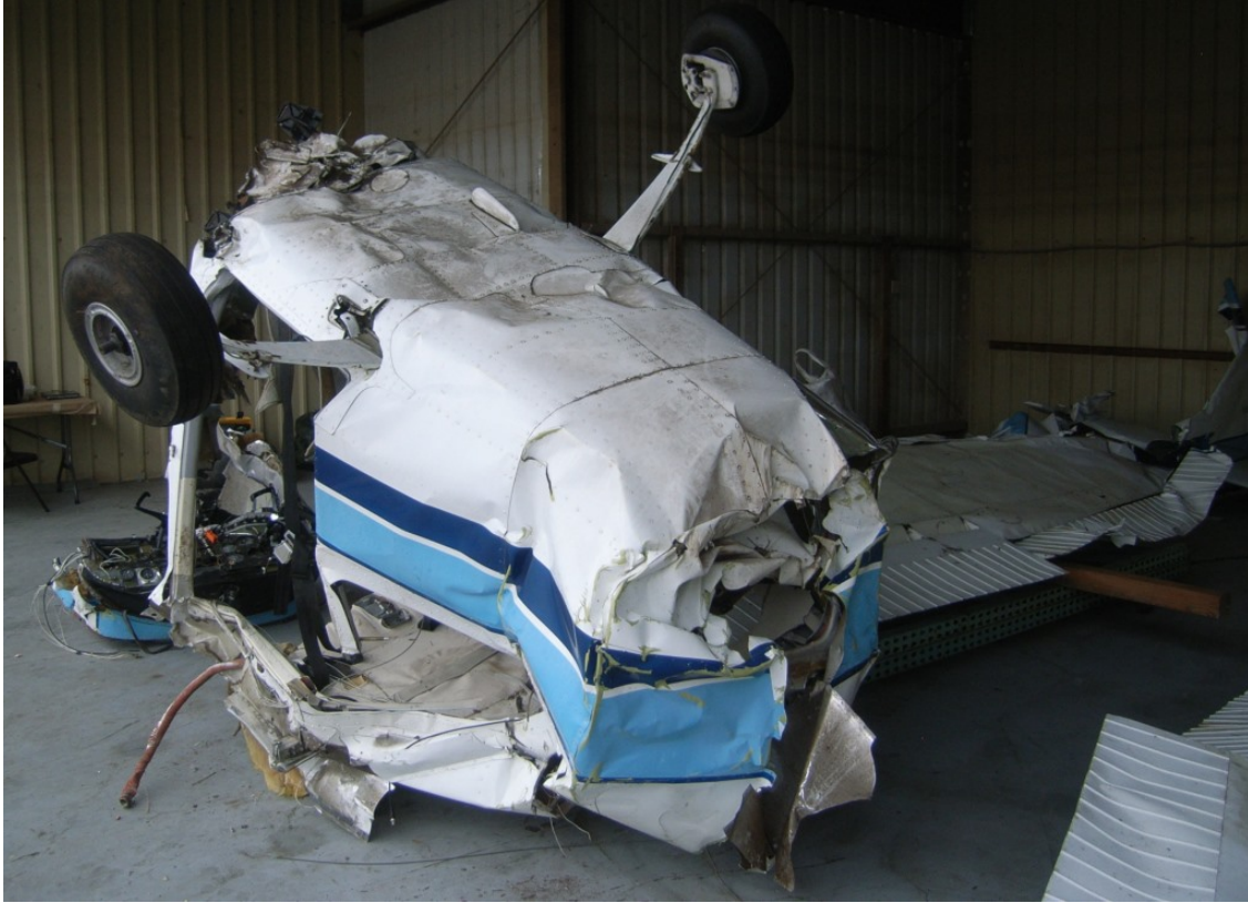
Figure 3 - Aft Right (note forward crushing of fuselage)
