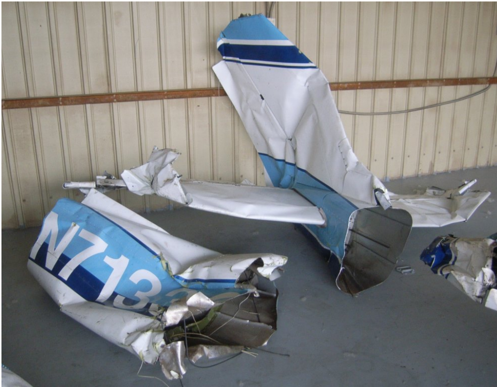
Figure 4 - Empennage and Aft Fuselage
