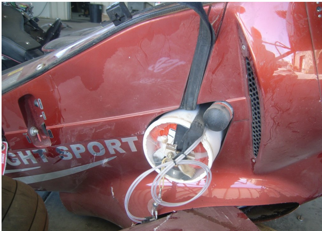
Figure 1 - Left Side of Aircraft (note lack of placards)
