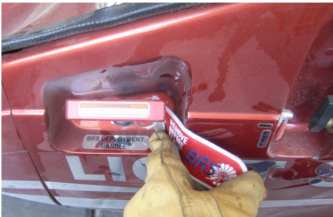
Figure 2 - BRS Deployment Handle (with safety pin in place)
