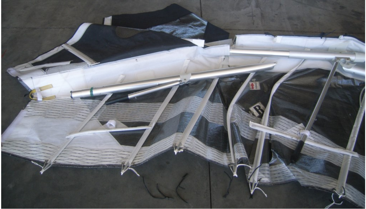
Figure 15 - Fractured Right Spar
