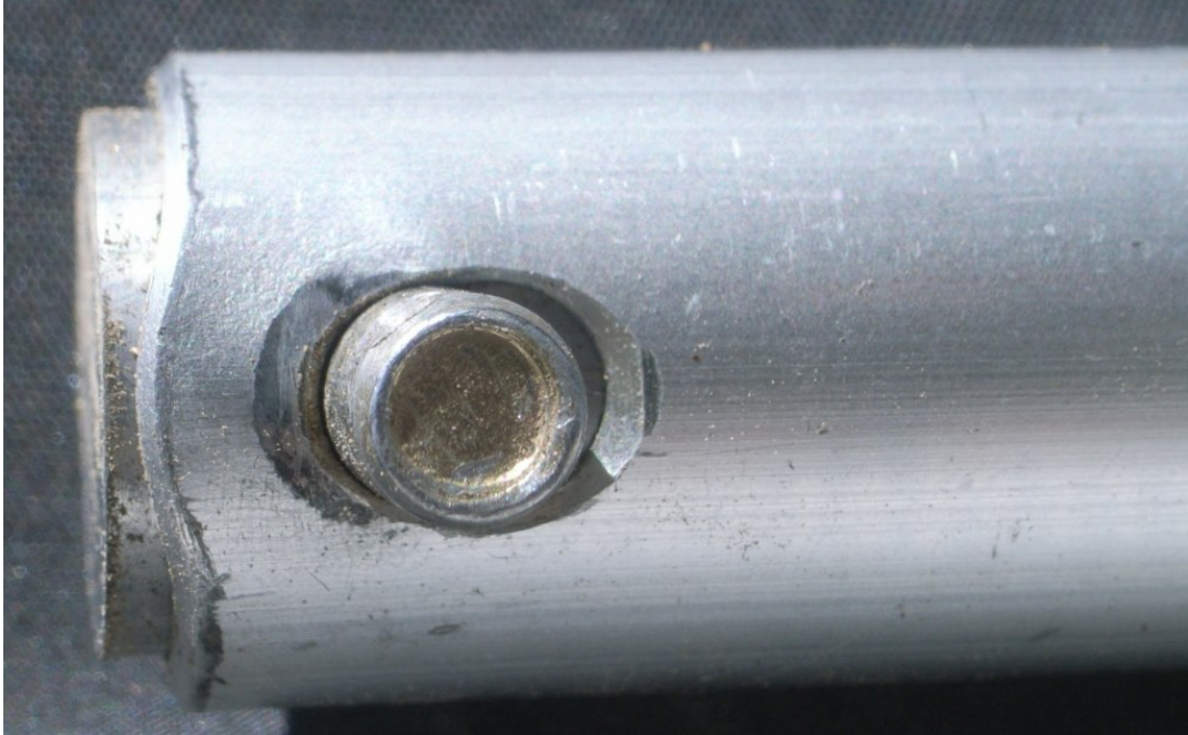
Figure 21 - Elongated Hole in Pitch Trim Actuator
