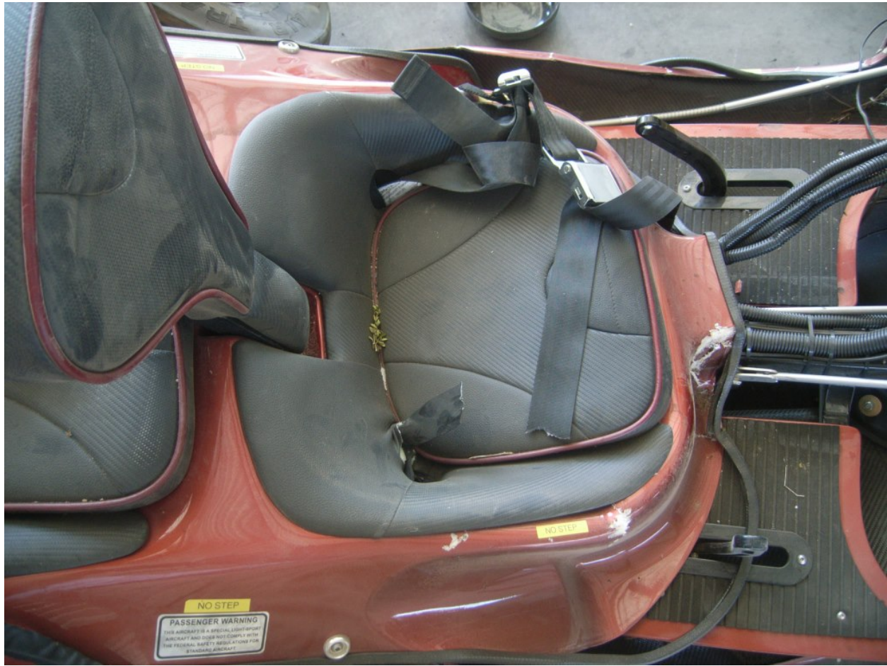
Figure 8 - Forward Seat (note cut belt)
