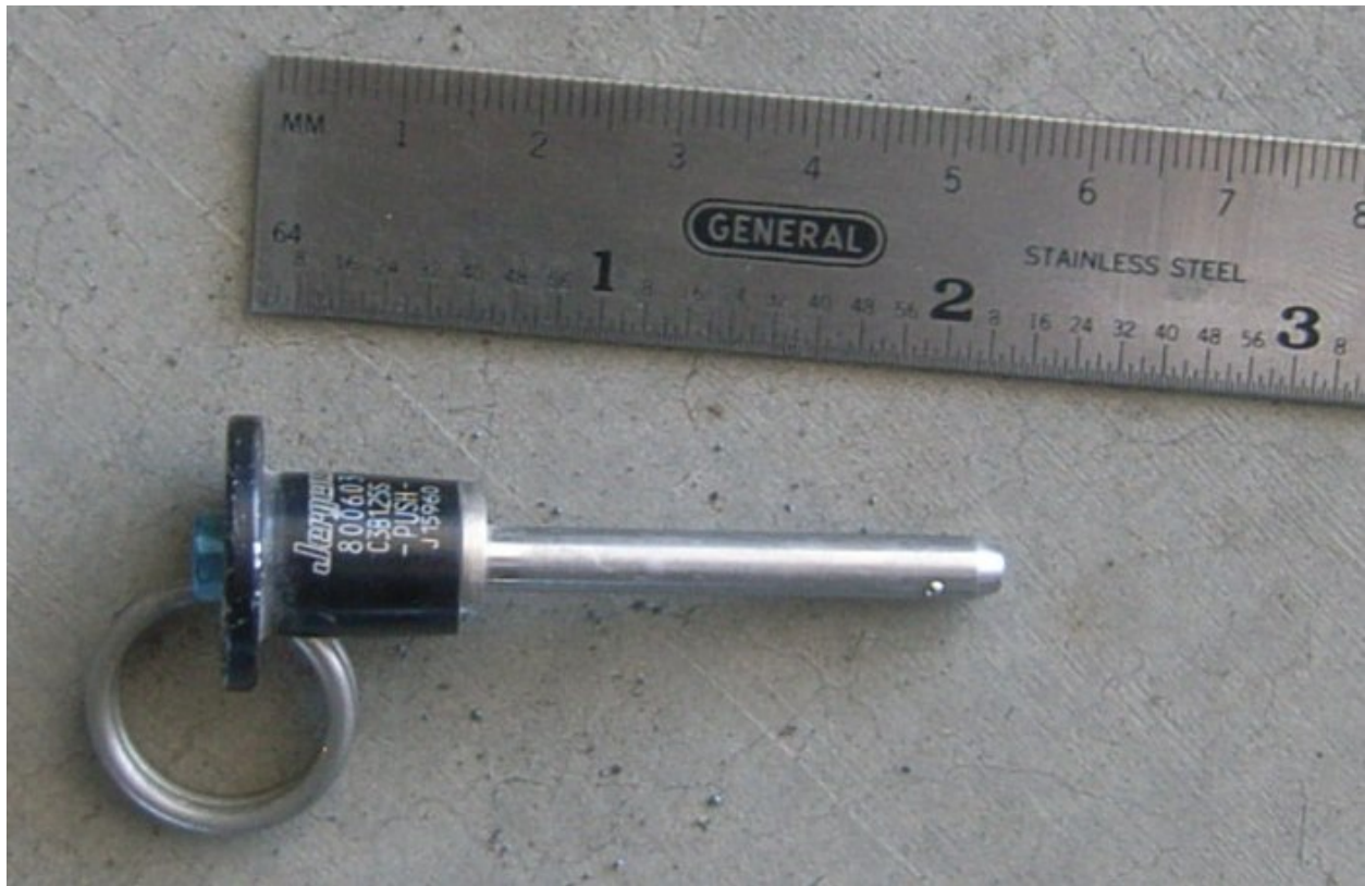
Figure 17 - Unassociated Quick Release Pin
