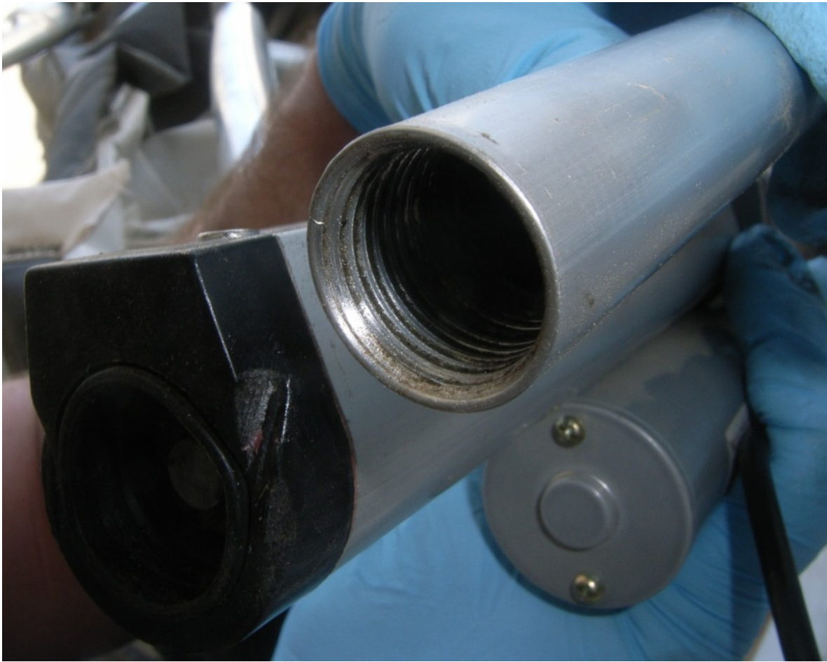
Figure 23 - Separated Actuator Tube (pitch trim)
