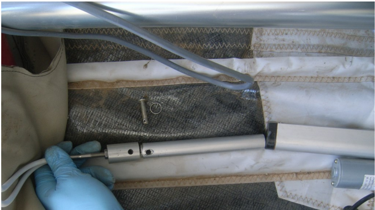
Figure 20 - Pitch Trim Assembly (Pin removed by investigators)
