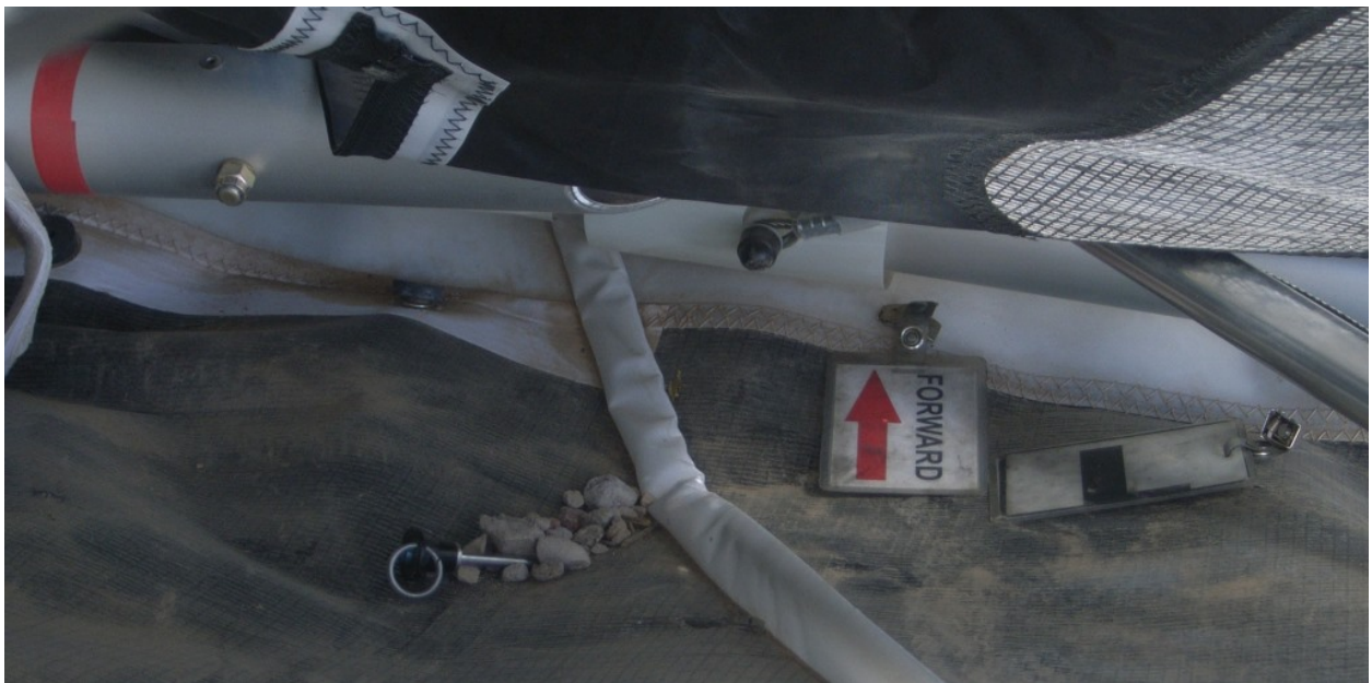
Figure 16 - Quick Release Pin in As-Found Location
