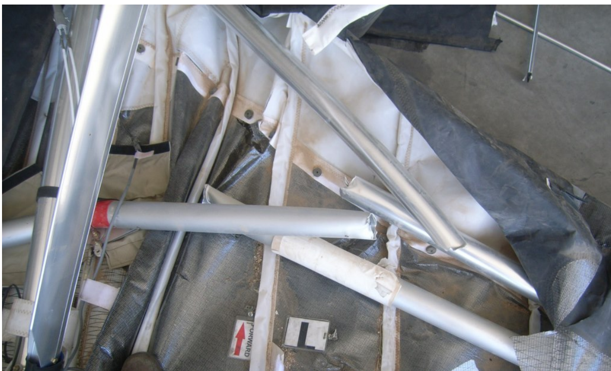
Figure 14 - Fractured Left Spars
