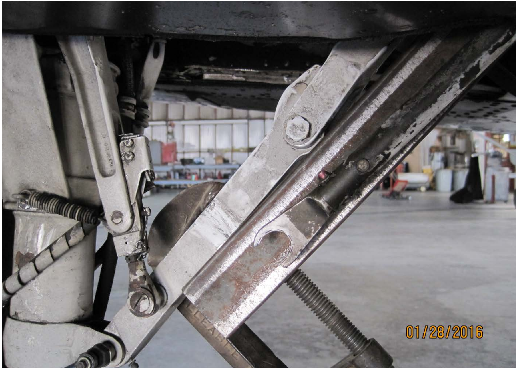
Photo 3 – View of Right Main Landing Gear Aft Tube Rod End
