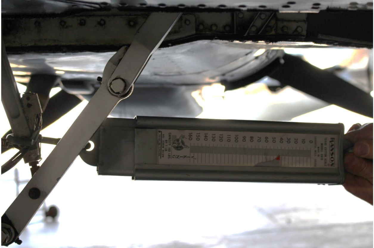
Photograph 3: Right Main Landing Gear Downlock Tension
