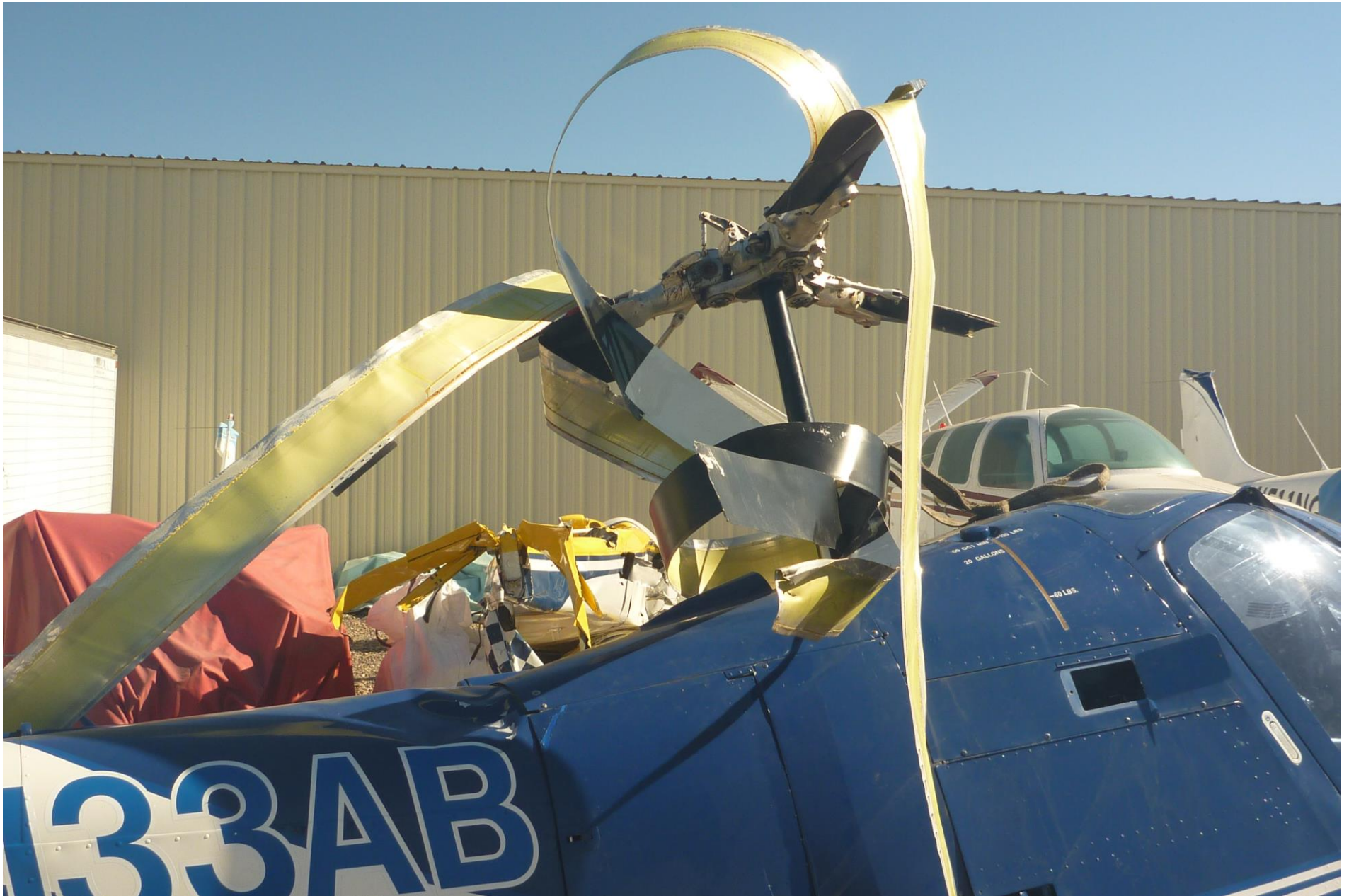
Photo 2 – Main Rotor Damage
