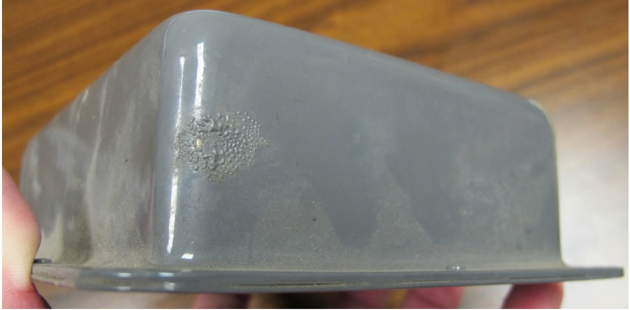
Figure 6 - Bubbled Paint on Control Box
