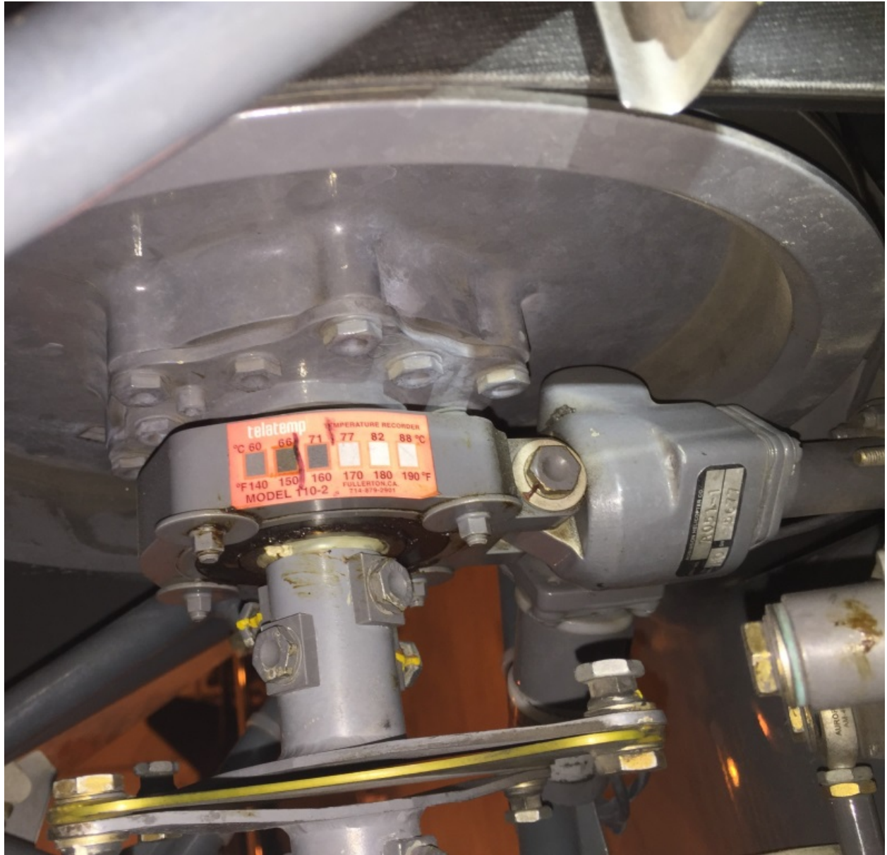
Figure 21 - Telatemp on Clutch Actuator Sheave at Intermediate Flex Coupling
