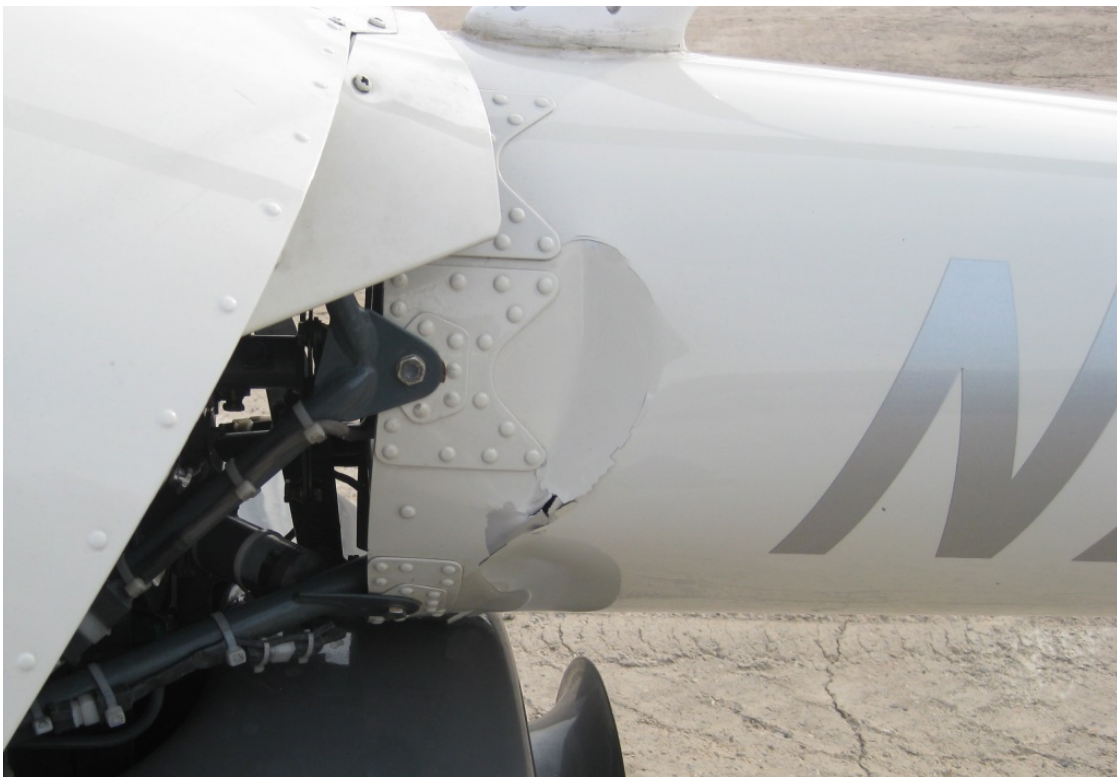
Figure 9 - Buckled Tail Boom
