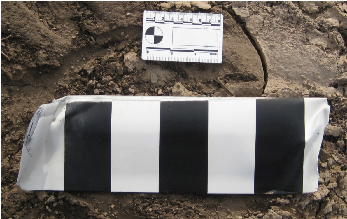
Figure 8 -Fracture-Separated Tail Rotor Blade Segment
