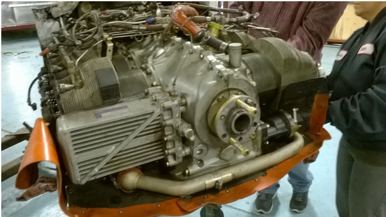
Figure 2 – Teledyne Continental TSIO- 520-RCM, S/n: 512148, Engine Exhibit from N91HC examination 01/05/2016.
