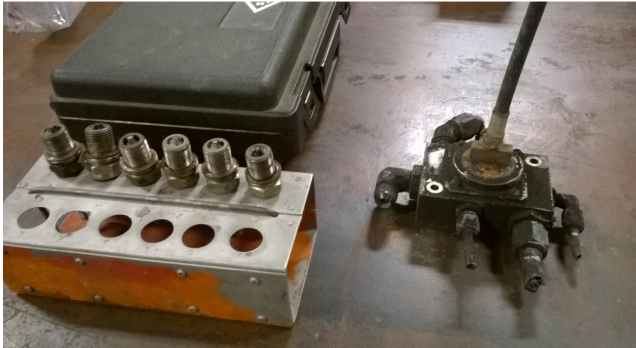
Figure 3 - Shows Top Sparkplug Exhibit's and Fuel Selector Valve from N91HC examination 01/05/2016.
