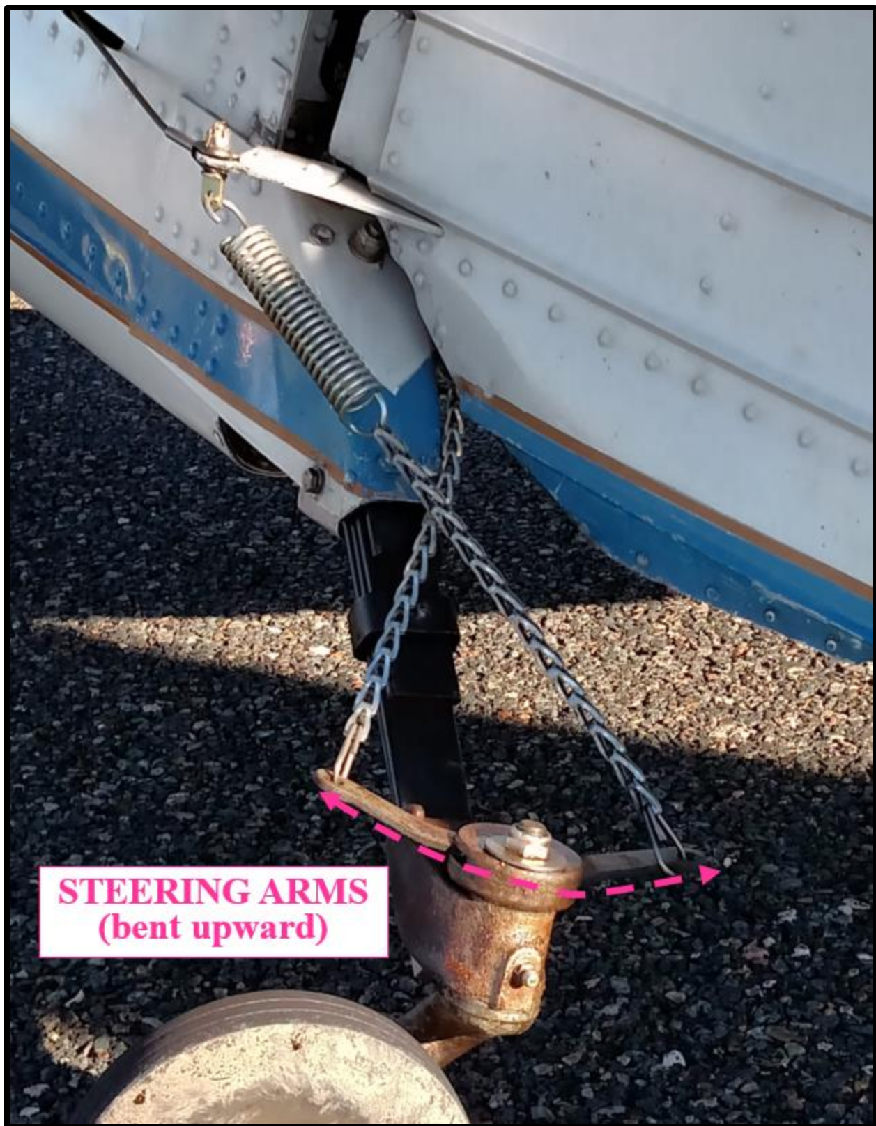
Picture 5: At Accident Site (steering arm bent upward)
