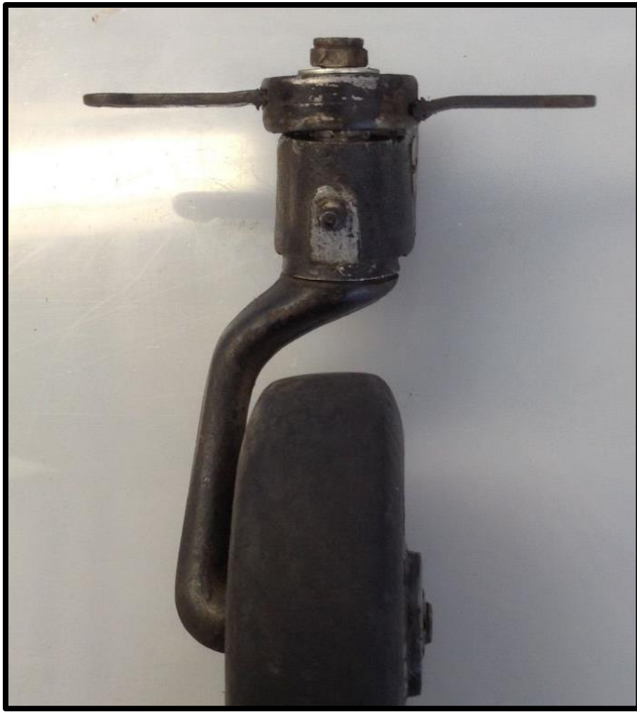
Picture 10: Exemplar steering arms misaligned
