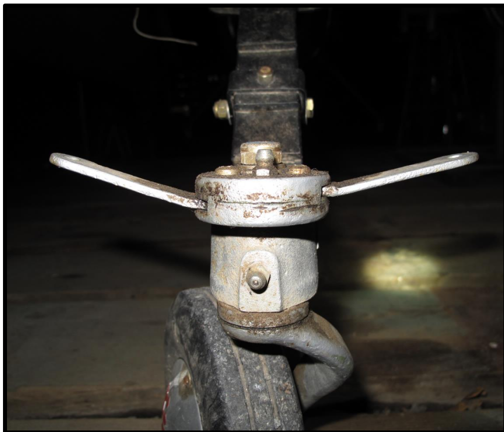
Picture 9: Exemplar steering arms bent upward
