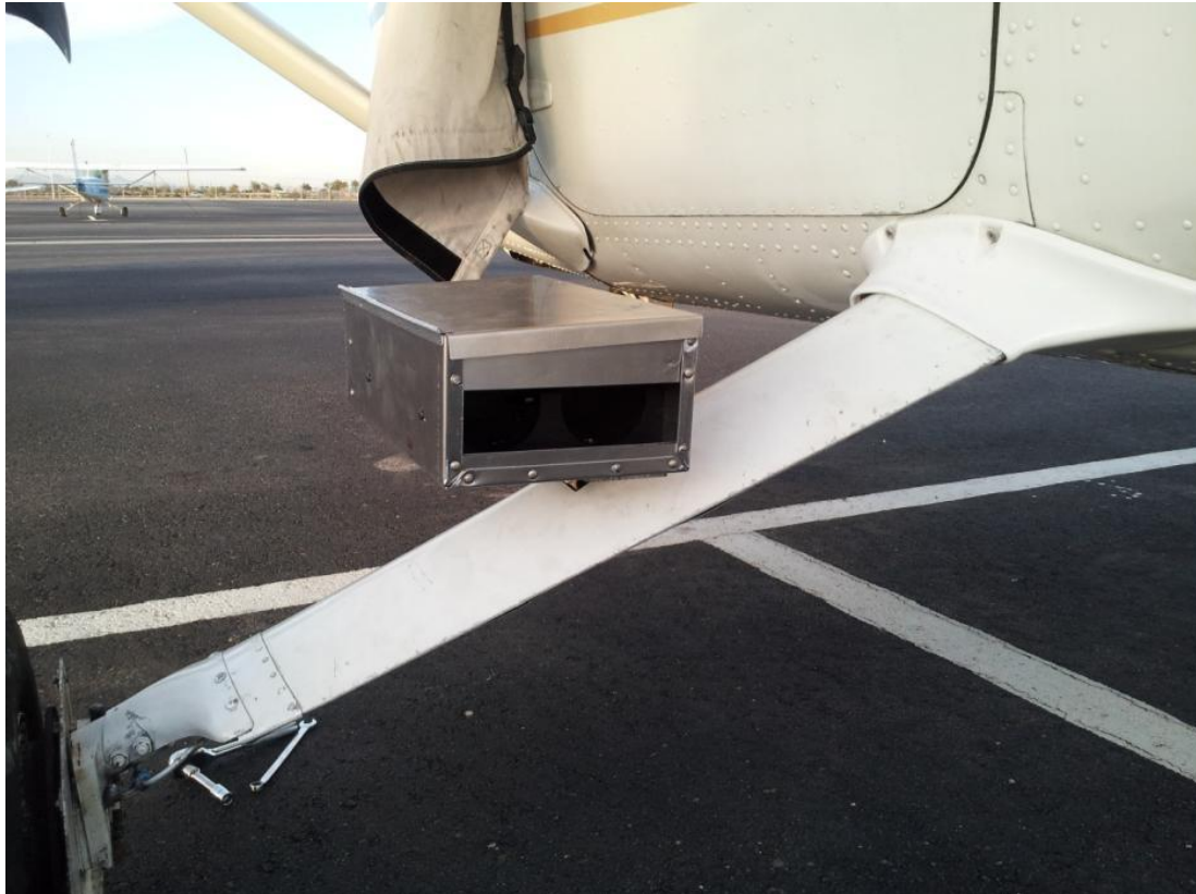
Aircraft owner supplied photograph of fireworks box installation
