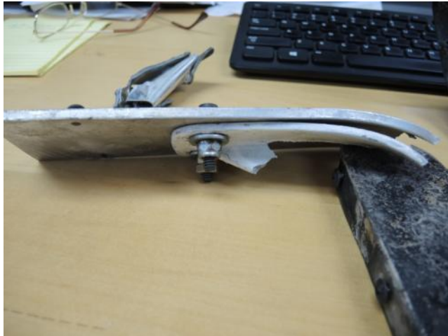
Wreckage exam ASI-16-DG-041.jpg Pyrotechnic box attached to door step
