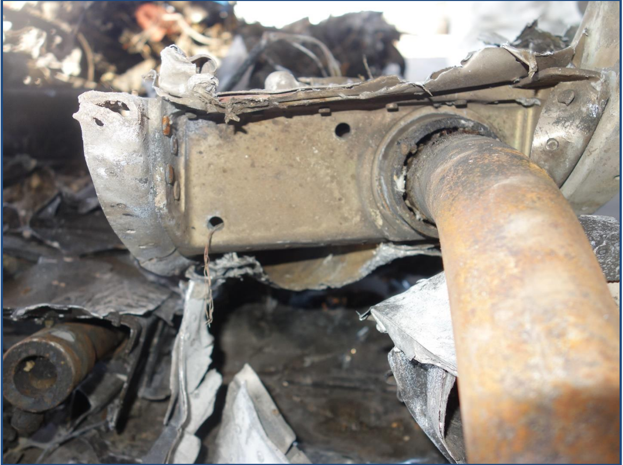
Figure 3: Wire running through a hole in the left landing gear bulkhead.
