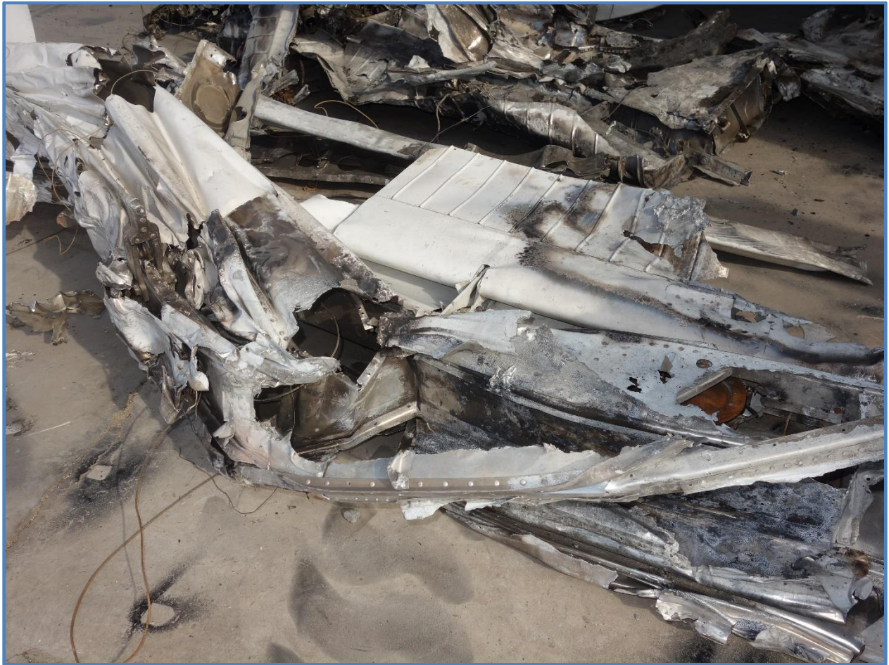
Figure 1: Interior of left wing where left main fuel tank was located.
