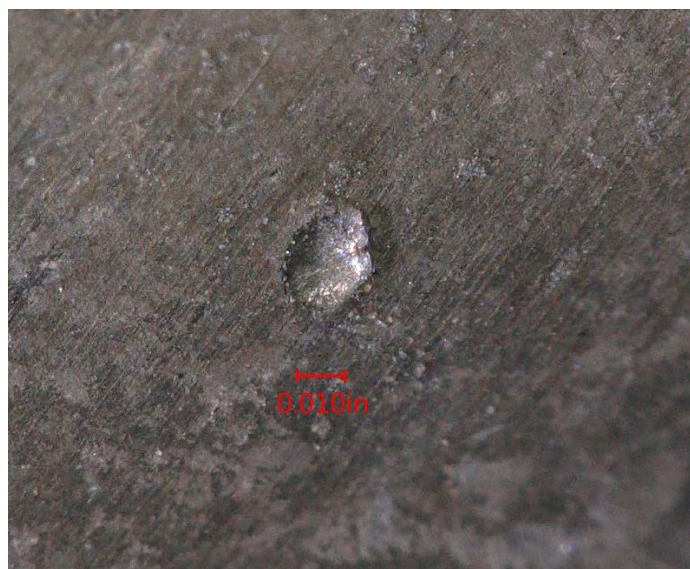
Figure 16: Particle impact craters on interior surface of portion #4.
