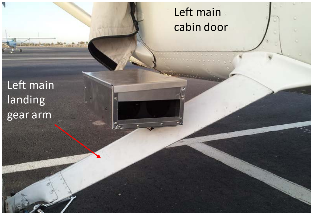
Figure 2: Pyrotechnics box as mounted on the left main landing gear arm.
