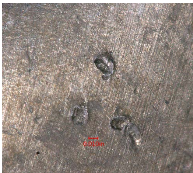
Figure 16: Particle impact craters on interior surface of portion #4.
