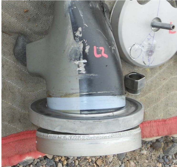
Photo #15 – L2 paint transfer mark and bearing retention lip fracture
