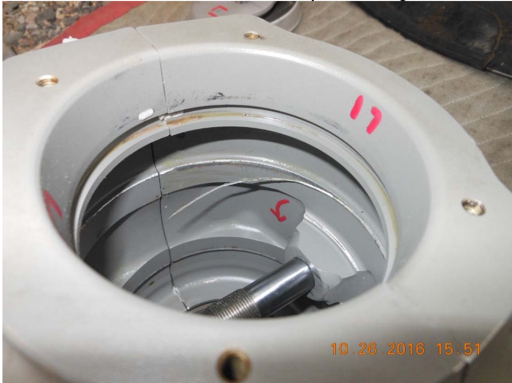
Photo #10 – Left hub L1 blade pocket damage
