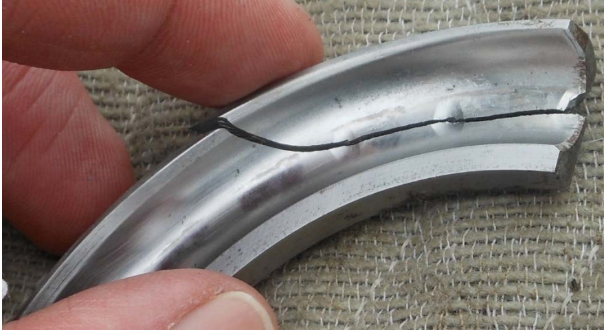
Photo #27 – R1 hub side bearing race fracture with ball impressions
