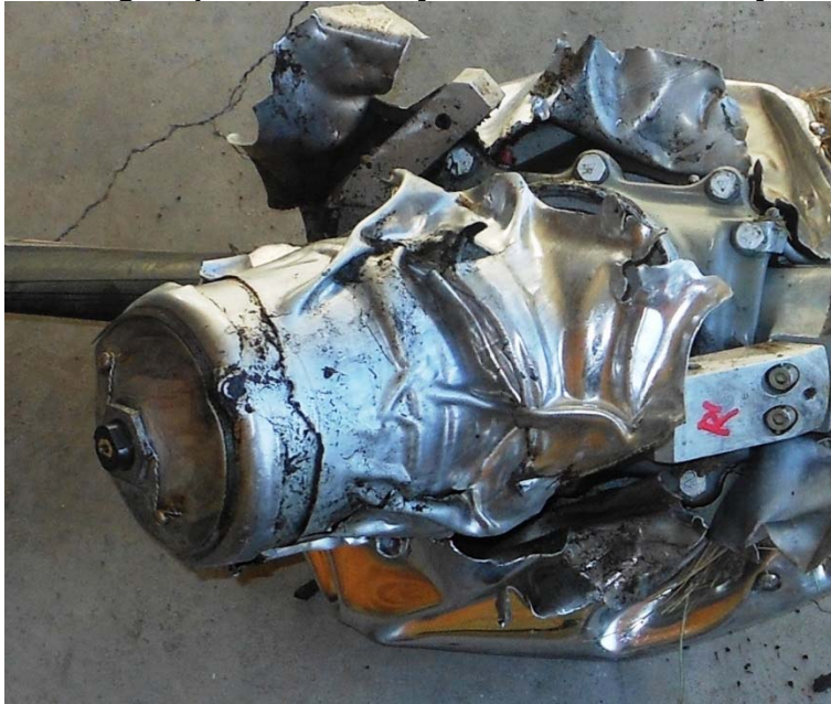
Photo #19 – Right spinner dome hydro-formed around hydraulic unit
