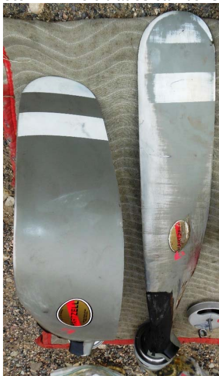
Photo #12 – Left blades camber side
