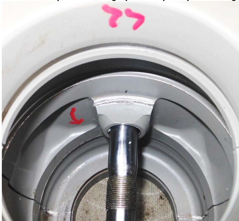
Photo #8 – Left hub L2 blade pocket damage (fwd side) and pitch change rod scuff marks
