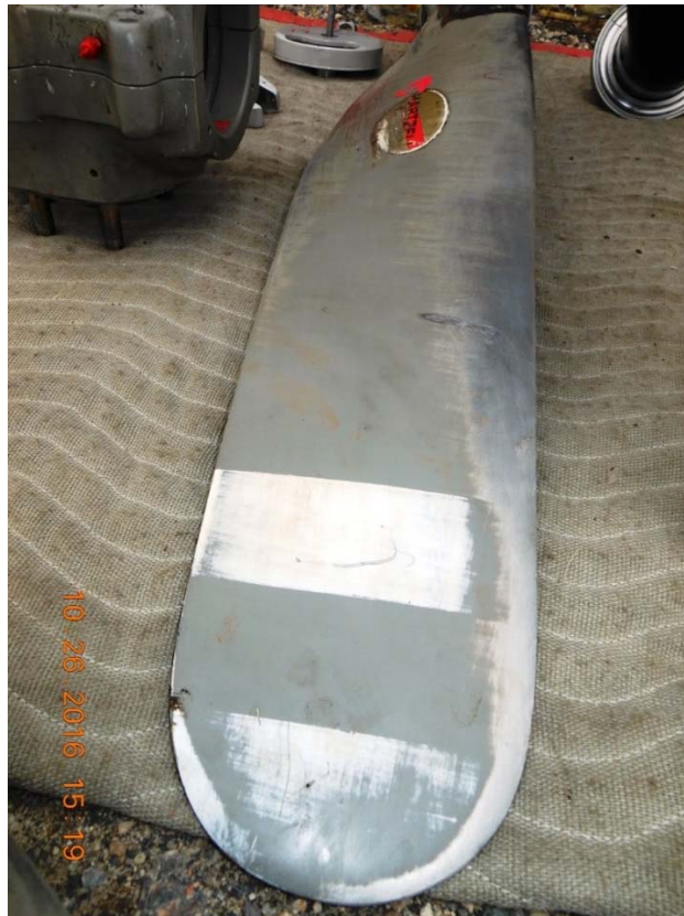
Photo #16 – L2 camber side chordwise/rotational abrasion
