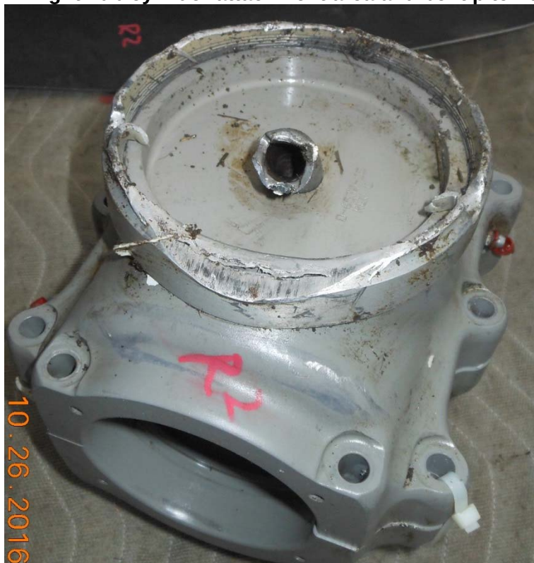
Photo #22 – Right hub cylinder attachment area and bent pitch change rod
