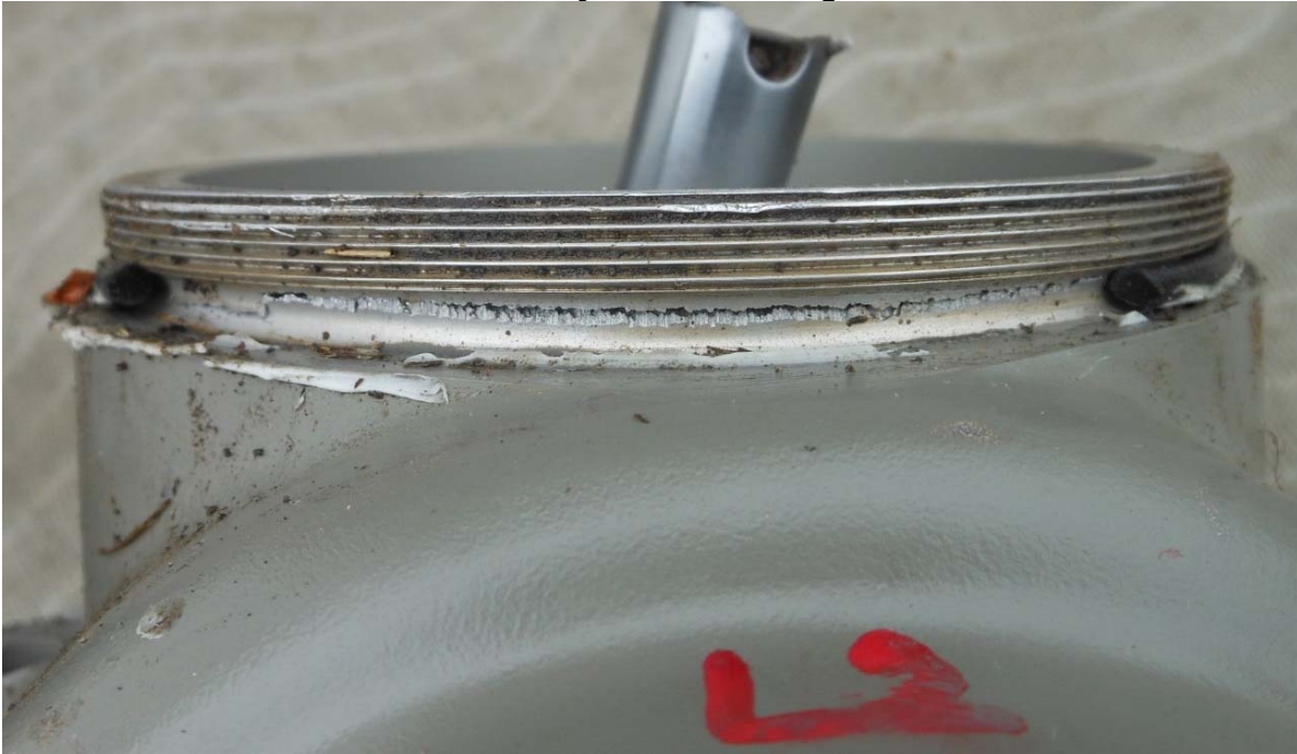
Photo #9 – Left hub cylinder mounting boss fracture
