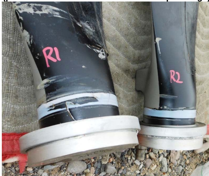
Photo #32 – Right blades shank trailing edge view (paint transfer mark and Teflon rub strip damage)
