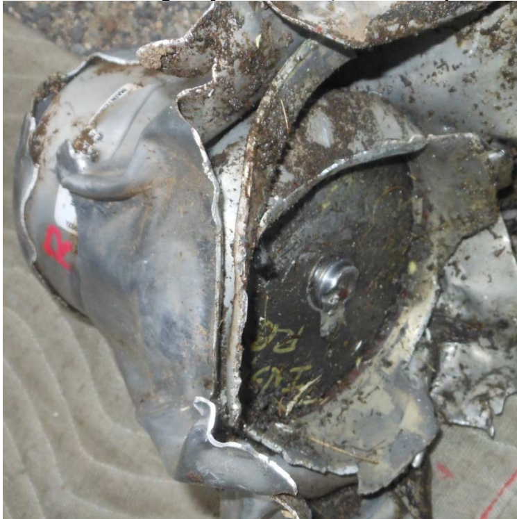
Photo #21 – Right hydraulic unit, aft side of piston
