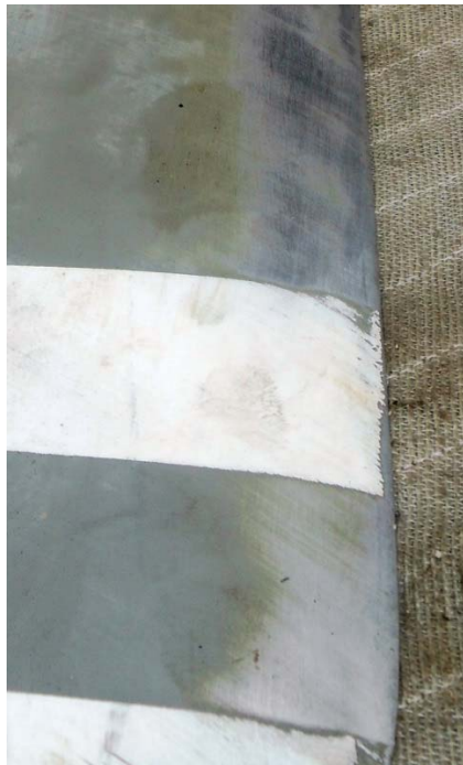
Photo #30 – R1 camber side chordwise/rotational abrasion
