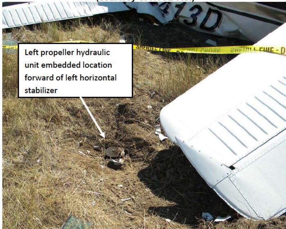
Photo #4 – Left propeller impact crater location, hydraulic unit dug out (courtesy of NTSB ASI)
