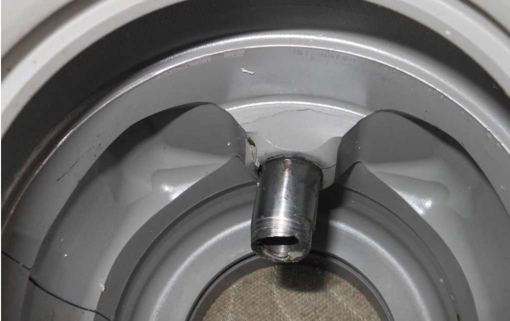
Photo #23 – Right pitch change rod forward segment and fractured boss
