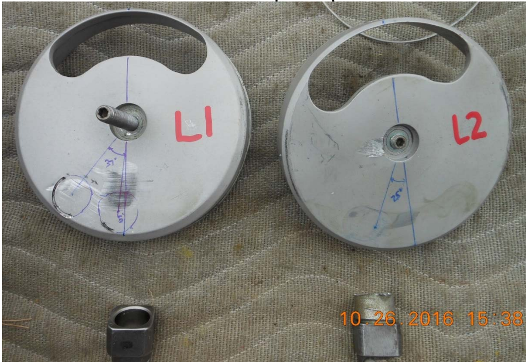
Photo #11 – Left preload plates
