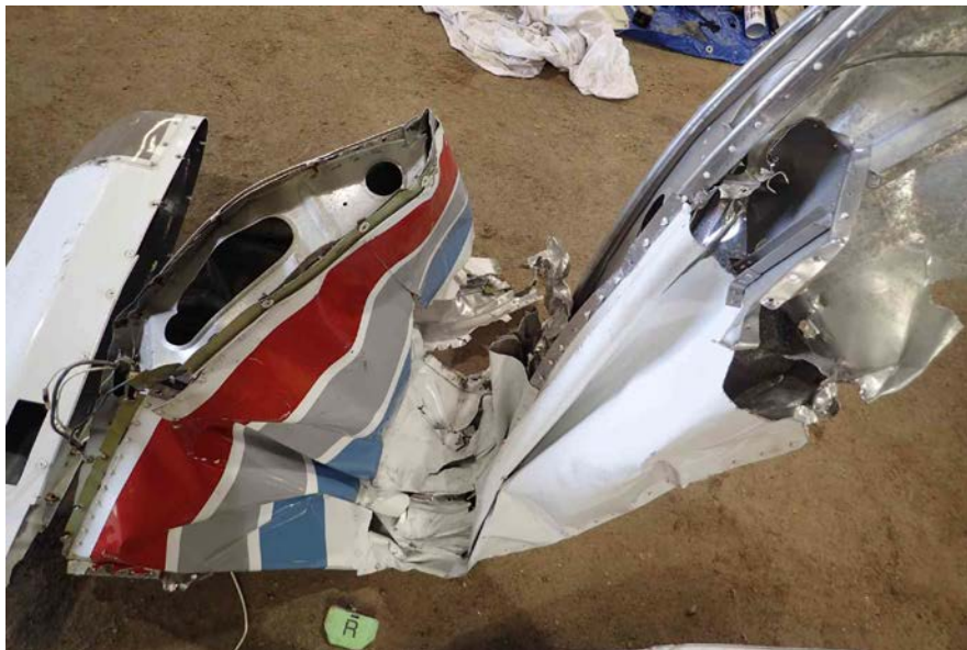
Photo 8 – Right Outboard Wing Section
