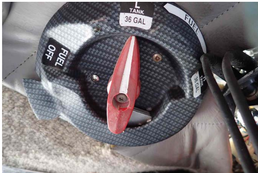
Photo 4 – Fuel Selector Valve
