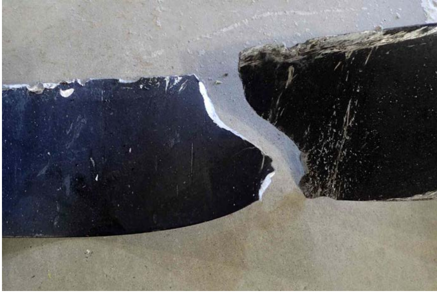
Photo 11 – Propeller Blade Separation
