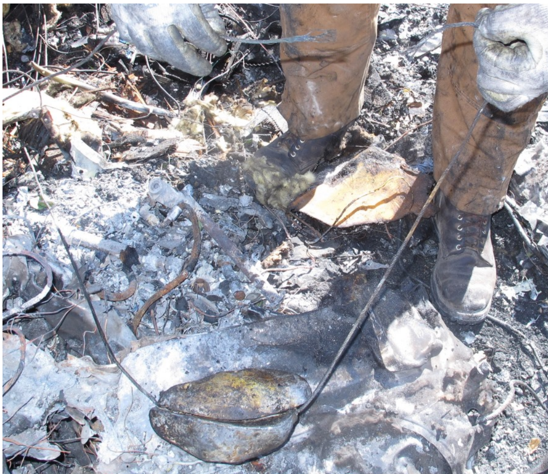
Figure 33 - Pitch Bobweight and Failed Cable Ends
