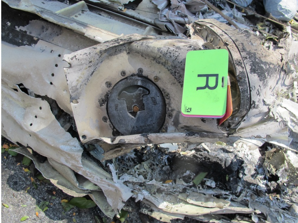
Figure 25 - Right Fuel Cap and Receptacle
