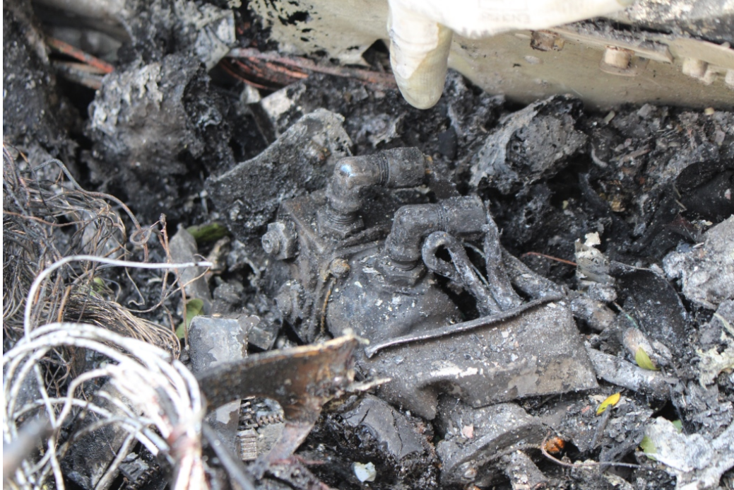
Figure 15 - Fuel Selector Valve (in situ)
