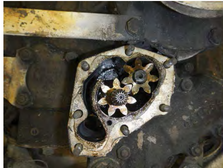
Figure 11 - photo 1 of oil pump
