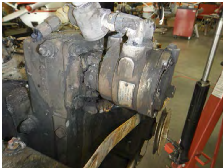
Figure 17 - photo of vacuum pump
