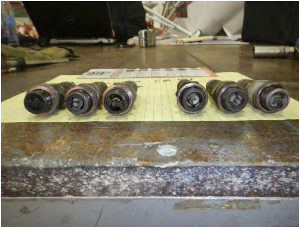
Figure 8 - photo of condition of spark plugs
