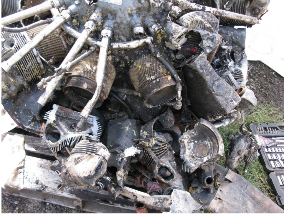
Figure 2: Engine and Damaged Cylinders
