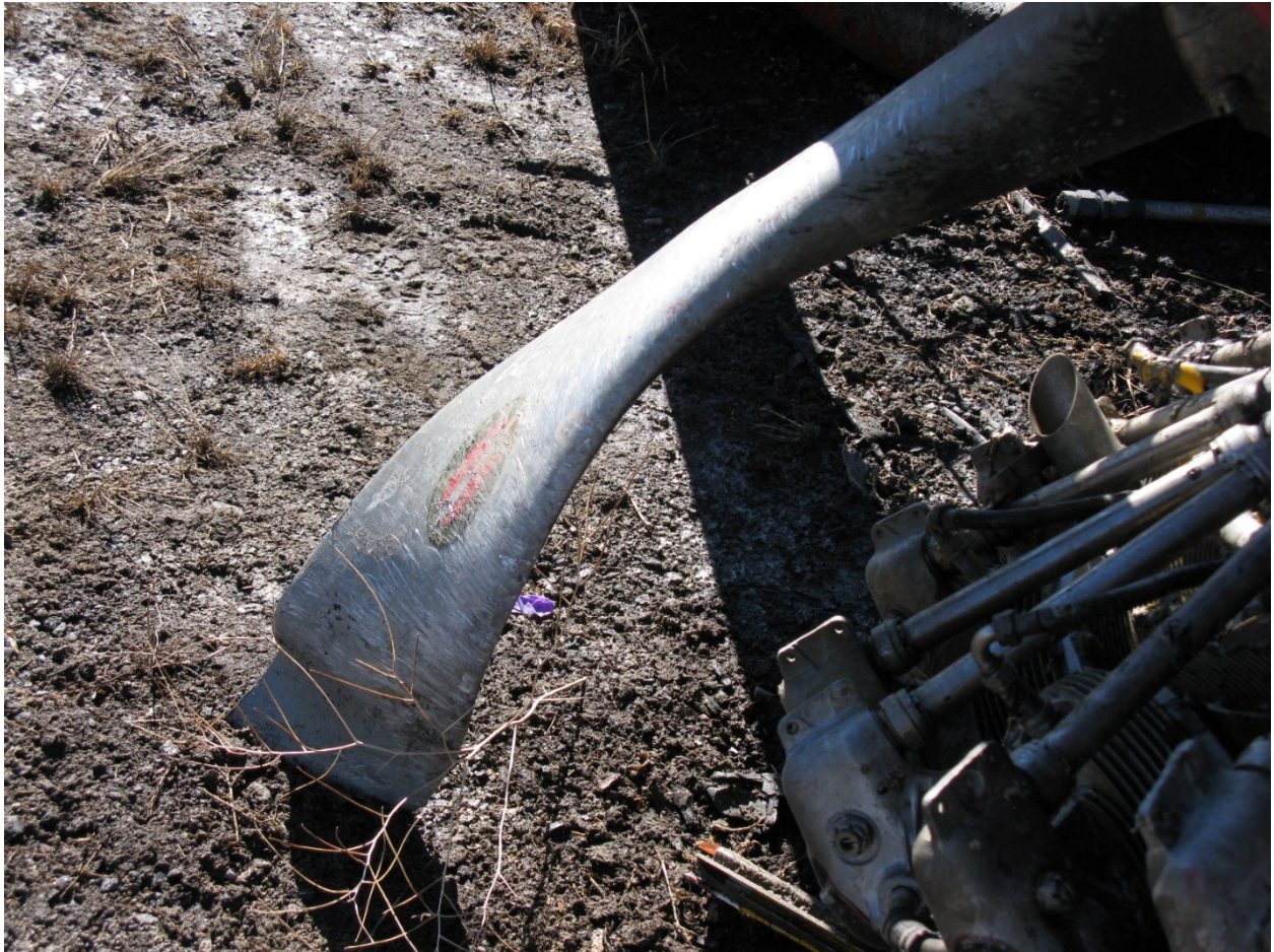
Figure 10: Propeller Blade “B” damage
