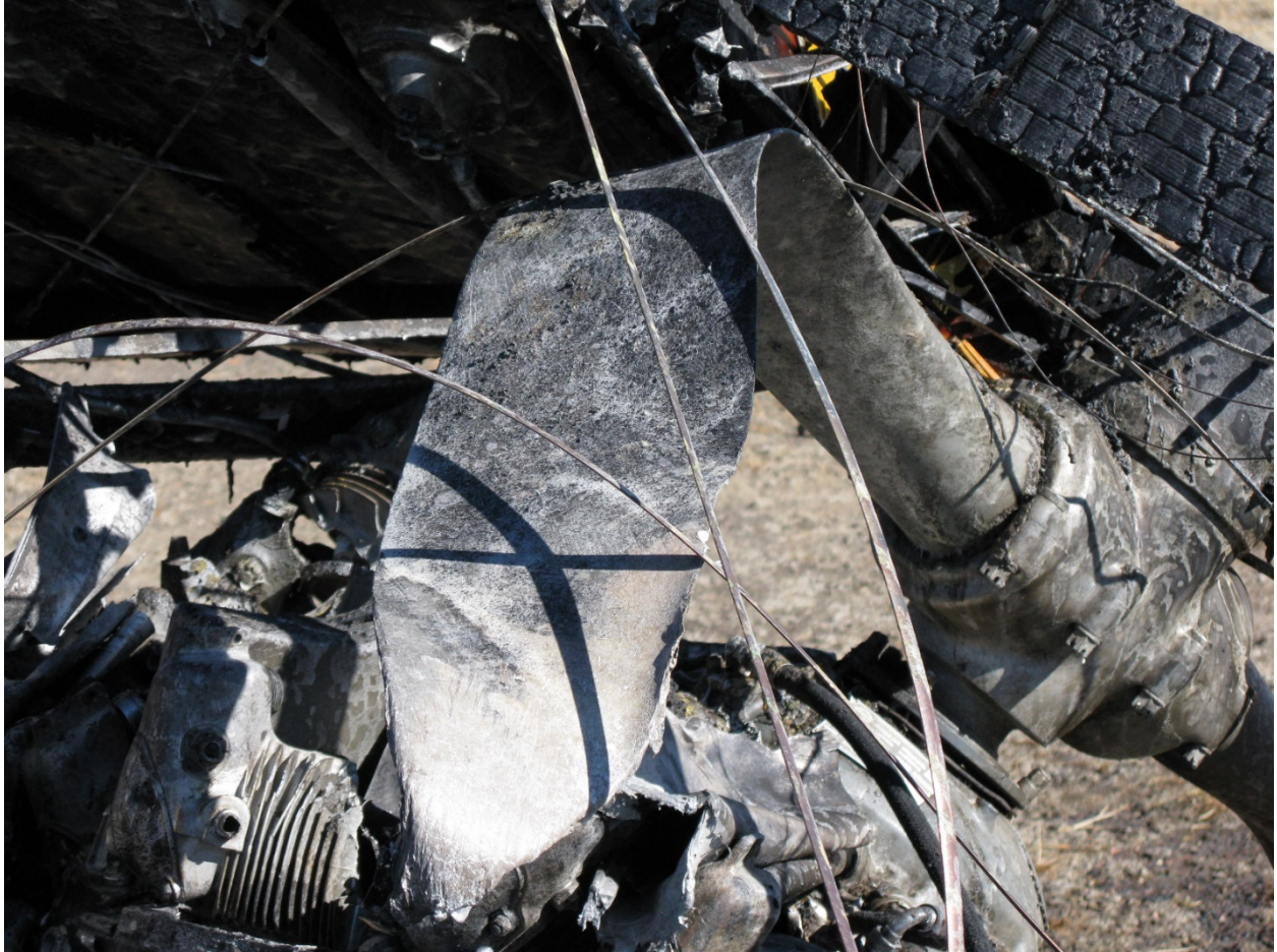
Figure 9: Propeller blade “A” Damage
