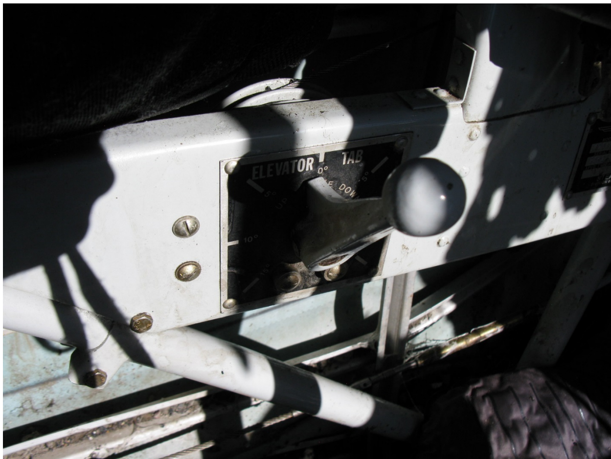
Figure 6: Elevator Trim Control set 0 Degrees Trim
