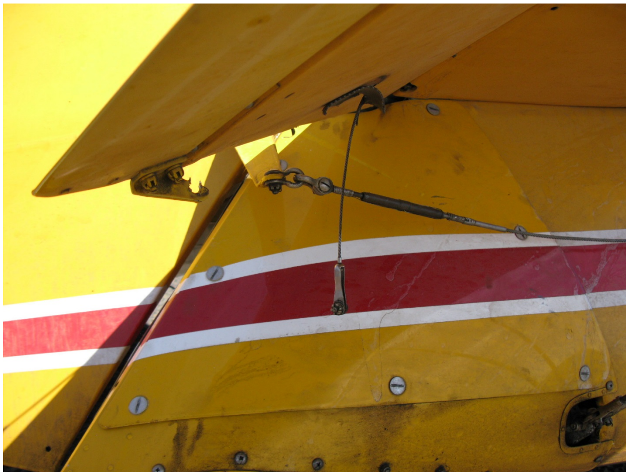
Figure 5: Right Elevator Lower Trim Cable Broken Free
