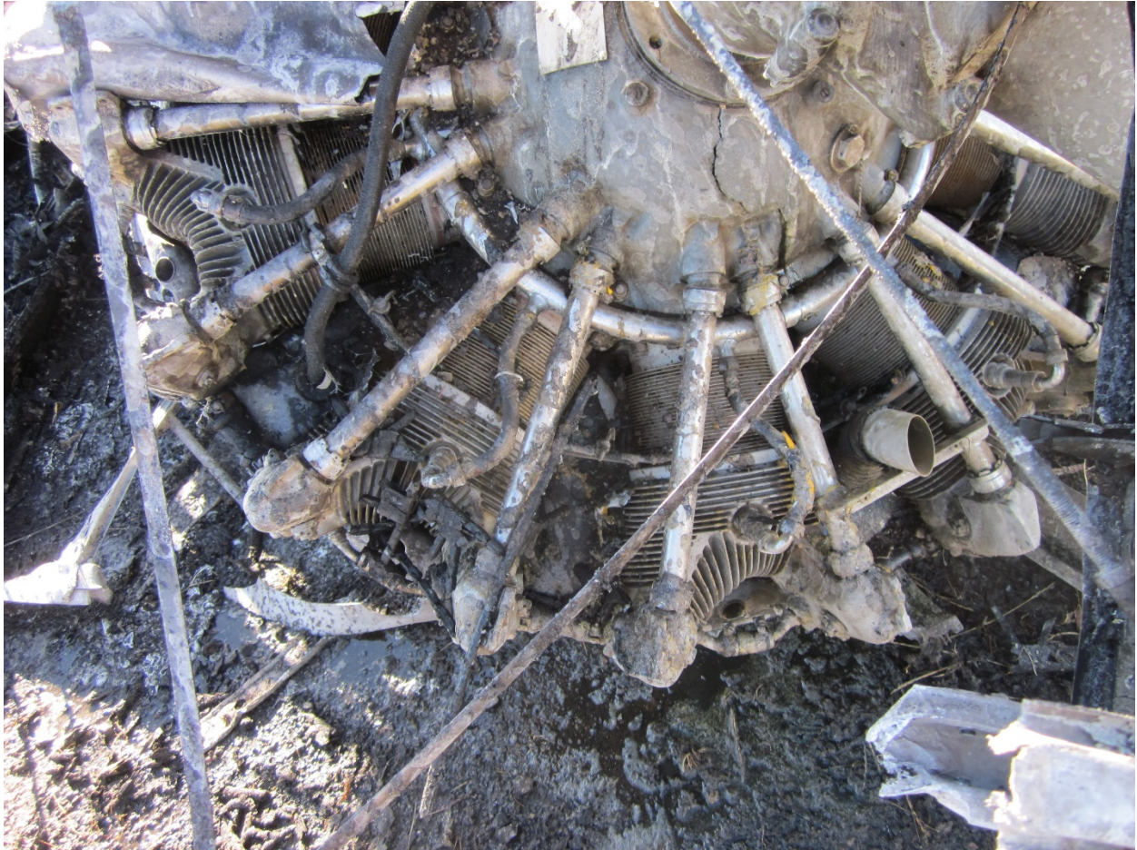
Figure 7: Close-up, Engine Impact Damage
