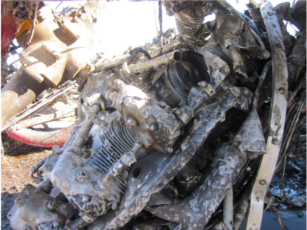
Figure 8: Close-up, Engine Impact Damage Lower Cylinders
