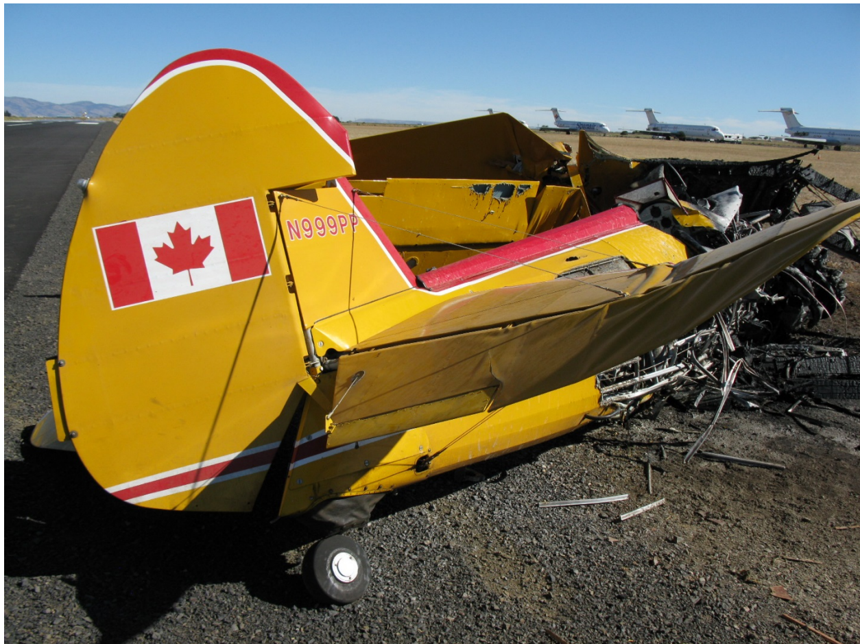
Figure 4: Right Horizontal Stabilizer and Elevator Impact Damage
