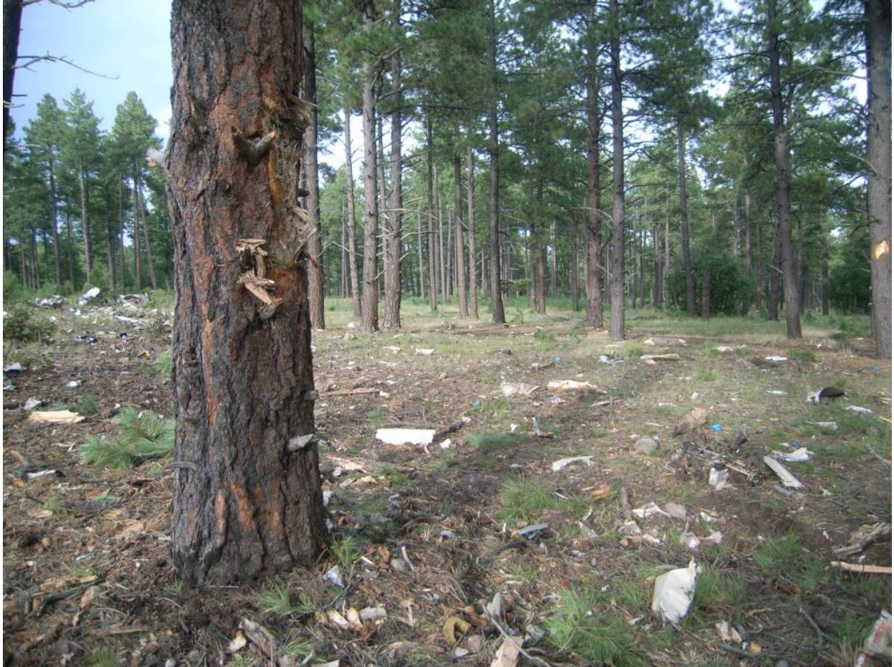
Figure 5 - Tree 8 (with L engine impact mark)
