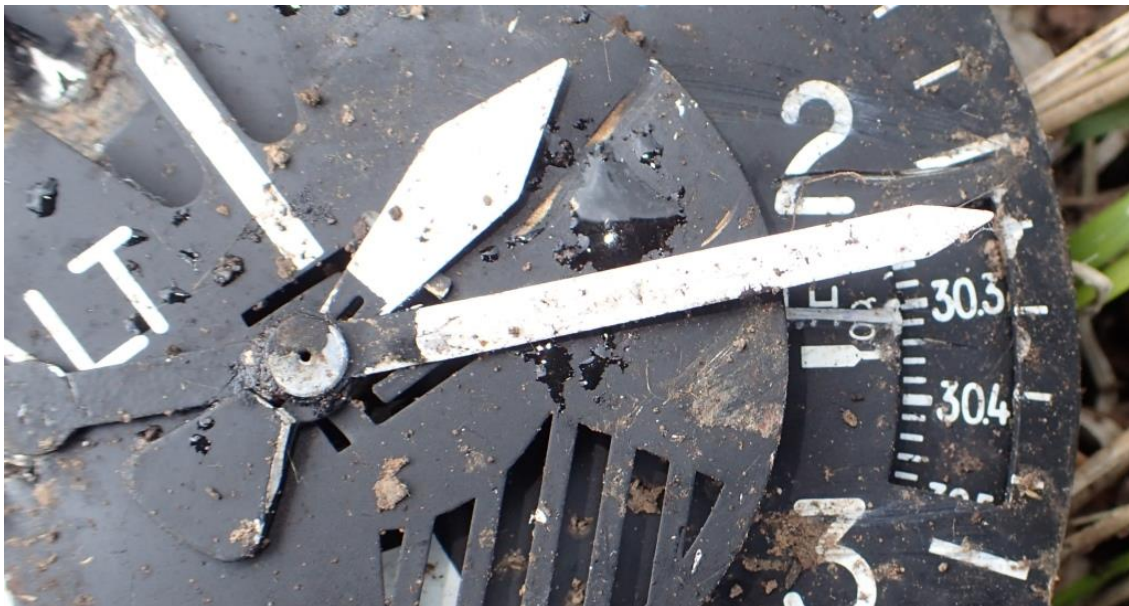
Figure 22 - Altimeter Barometric Setting
