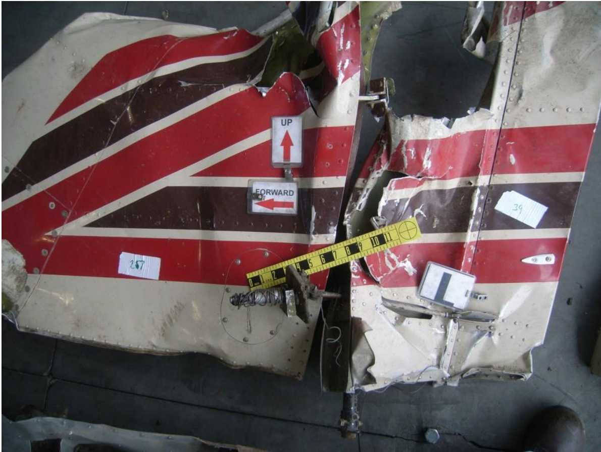
Figure 45 - Vertical Stabilizer and Rudder Segments
