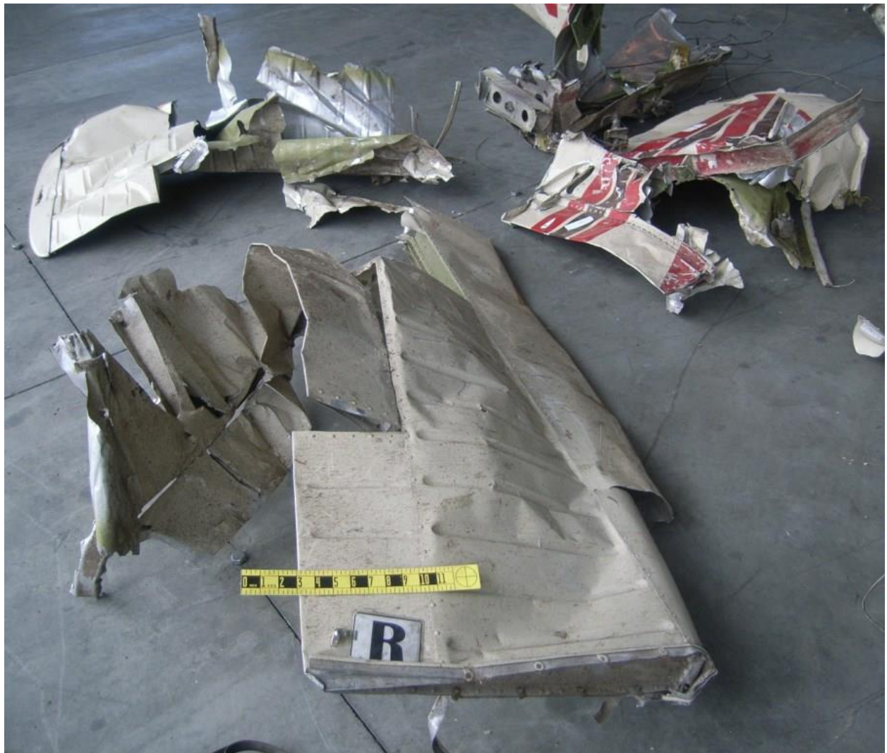
Figure 38 - L & R Stabilator, and Vertical Stabilizer Fragments
