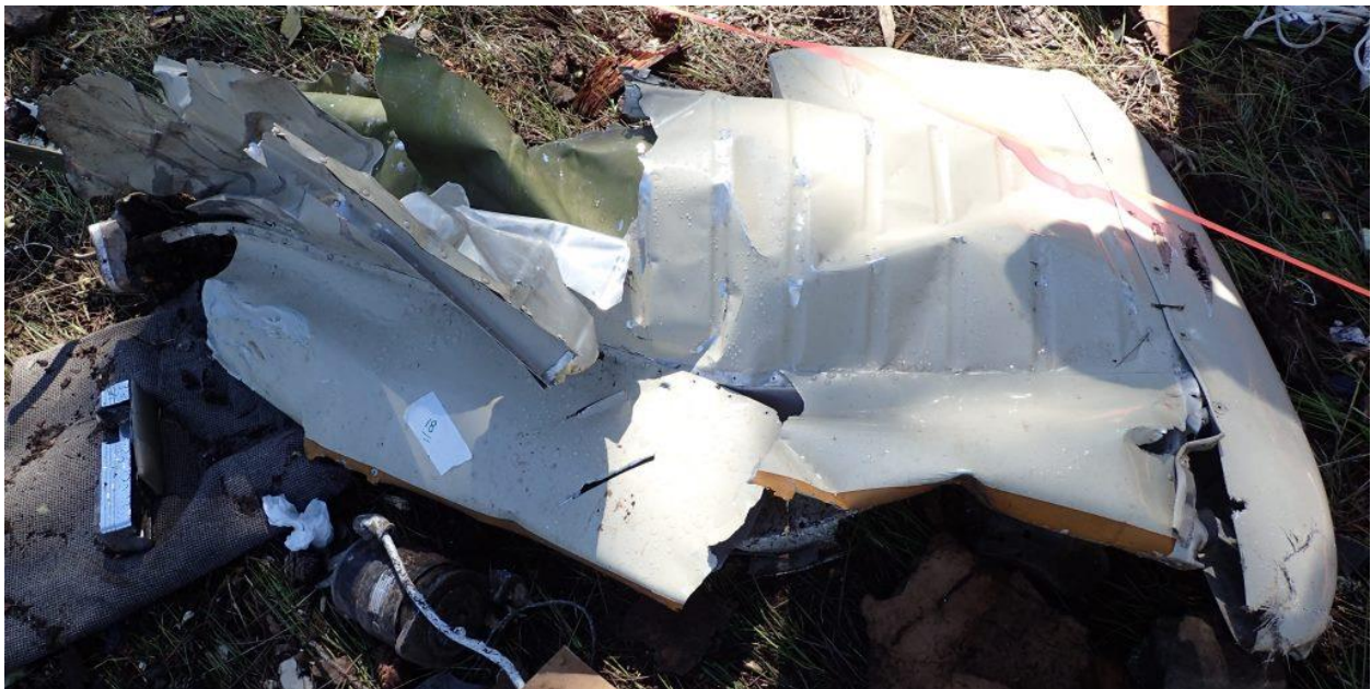
Figure 17 - Left Stabilator Fragment
