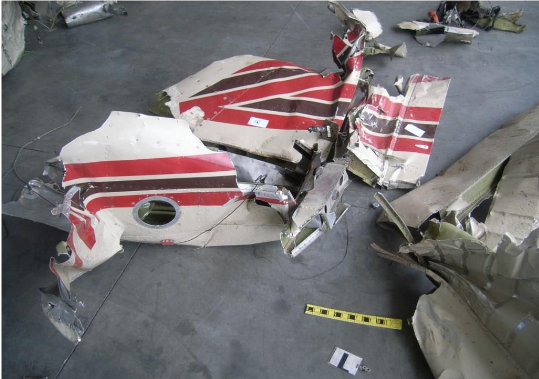
Figure 36 - Vertical Stabilizer and Rudder
