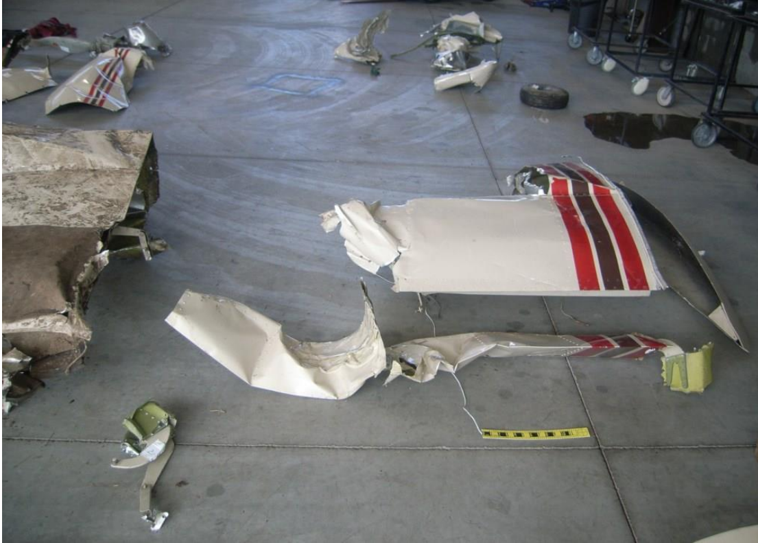
Figure 42 - Outboard Right Wing
