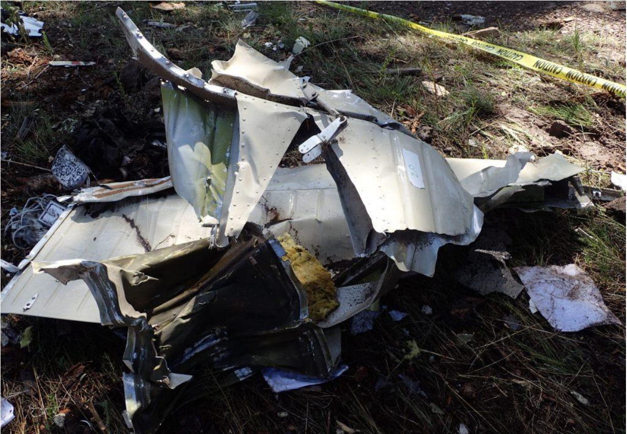
Figure 18 - Right and Center Stabilator Fragment
