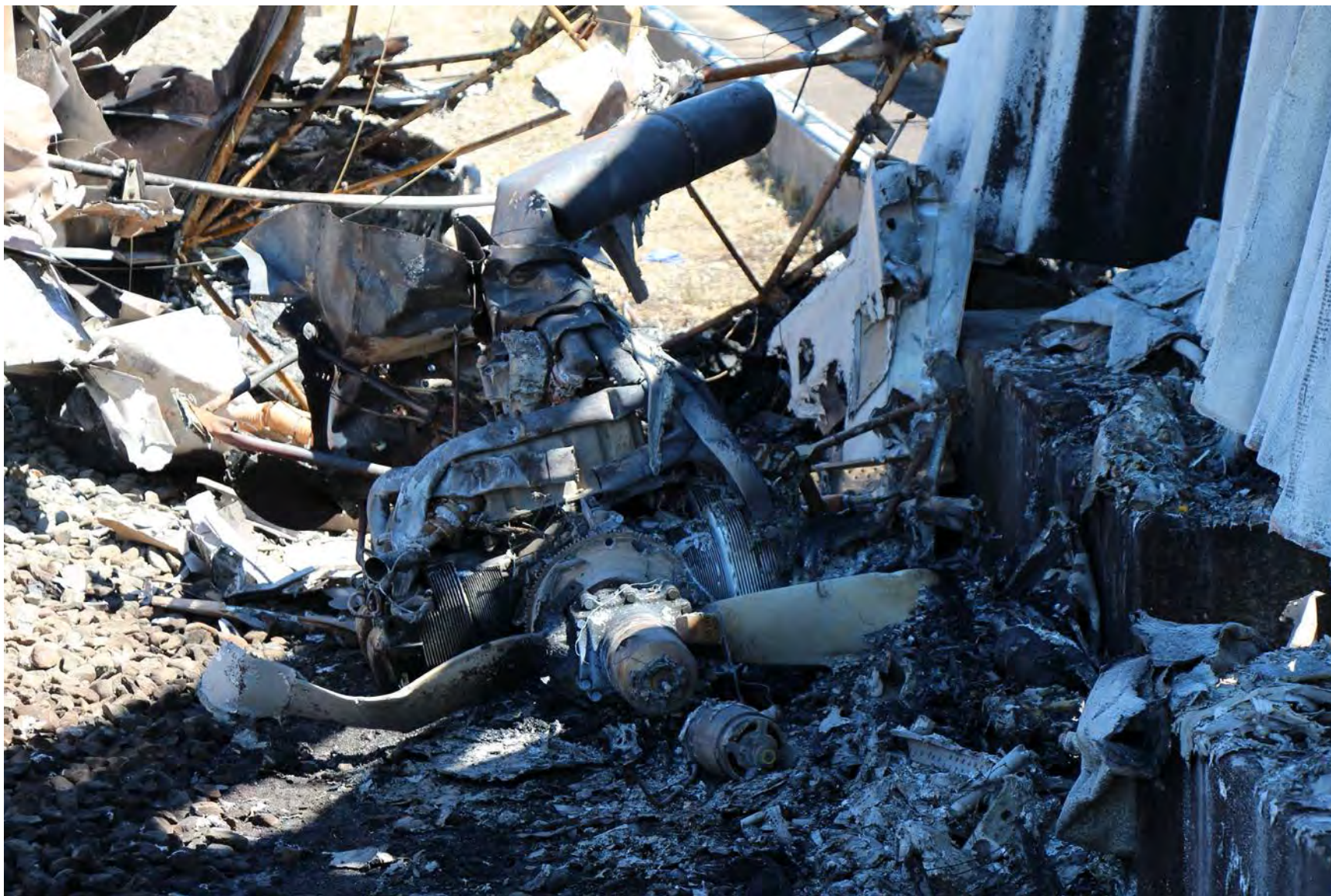
Photo 4 – Remnants of Right Wing and Right Engine at Accident Site
