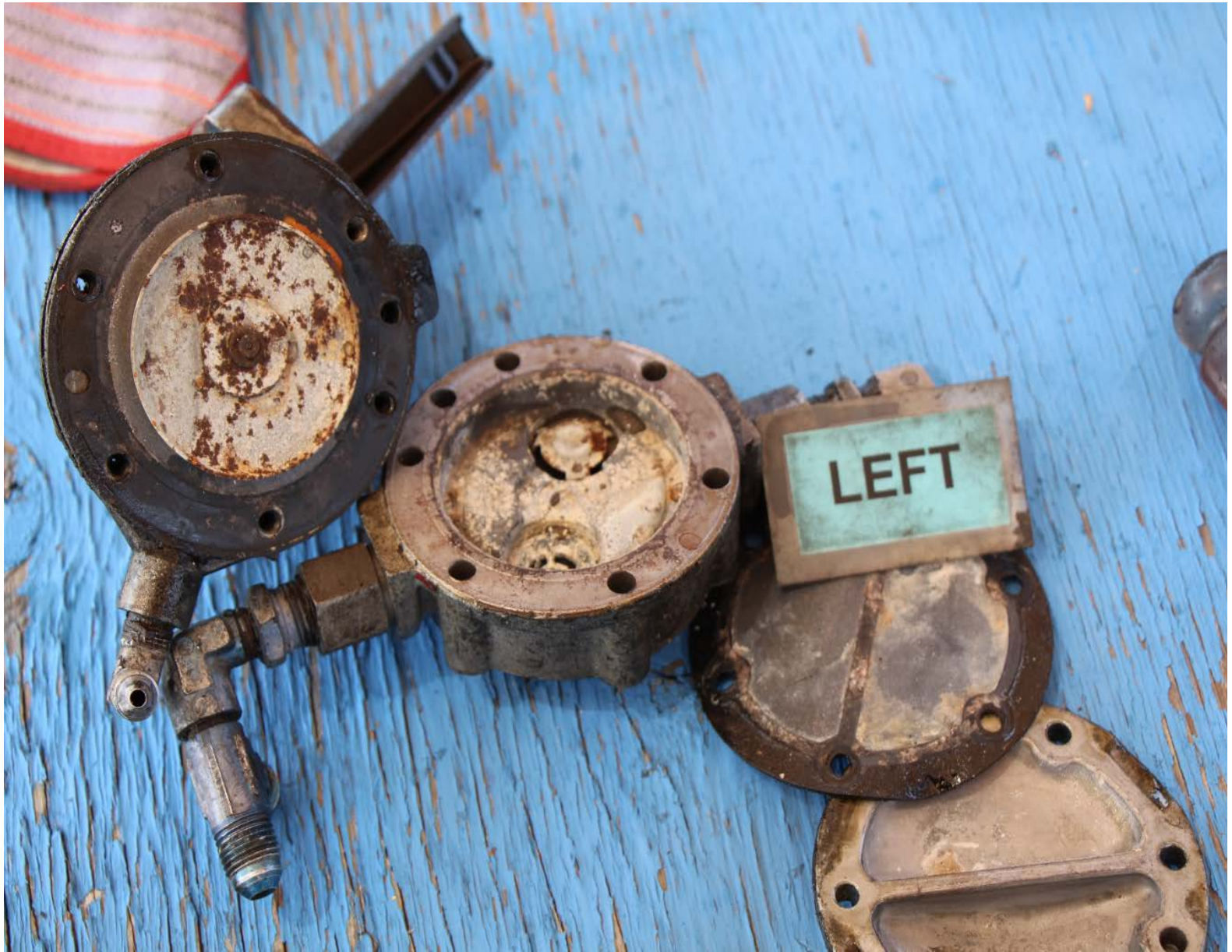
Photo 7 – Left Engine Fuel Pump
