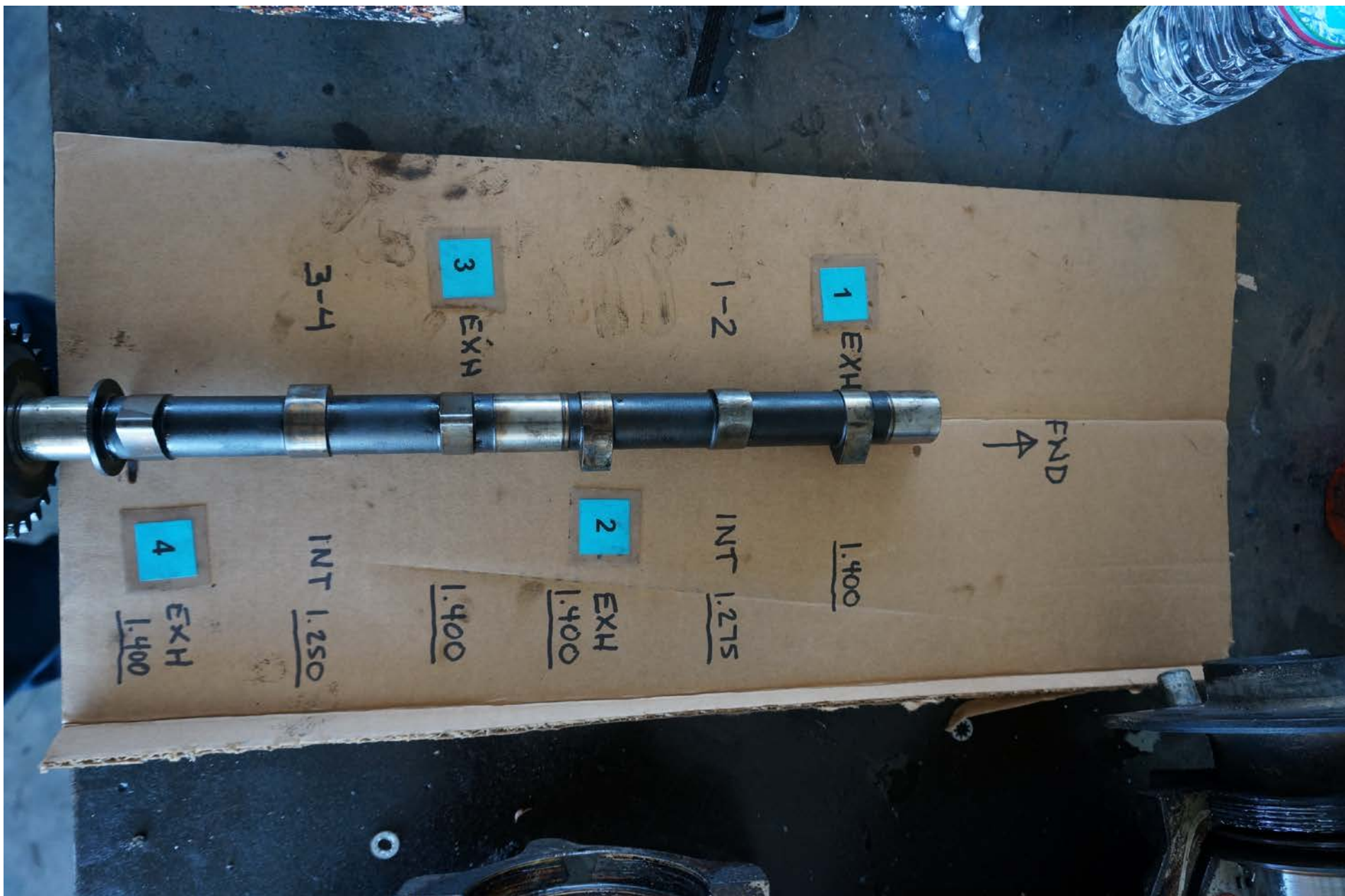
Photo 7 – Camshaft displaying wear to intake valve lobes
