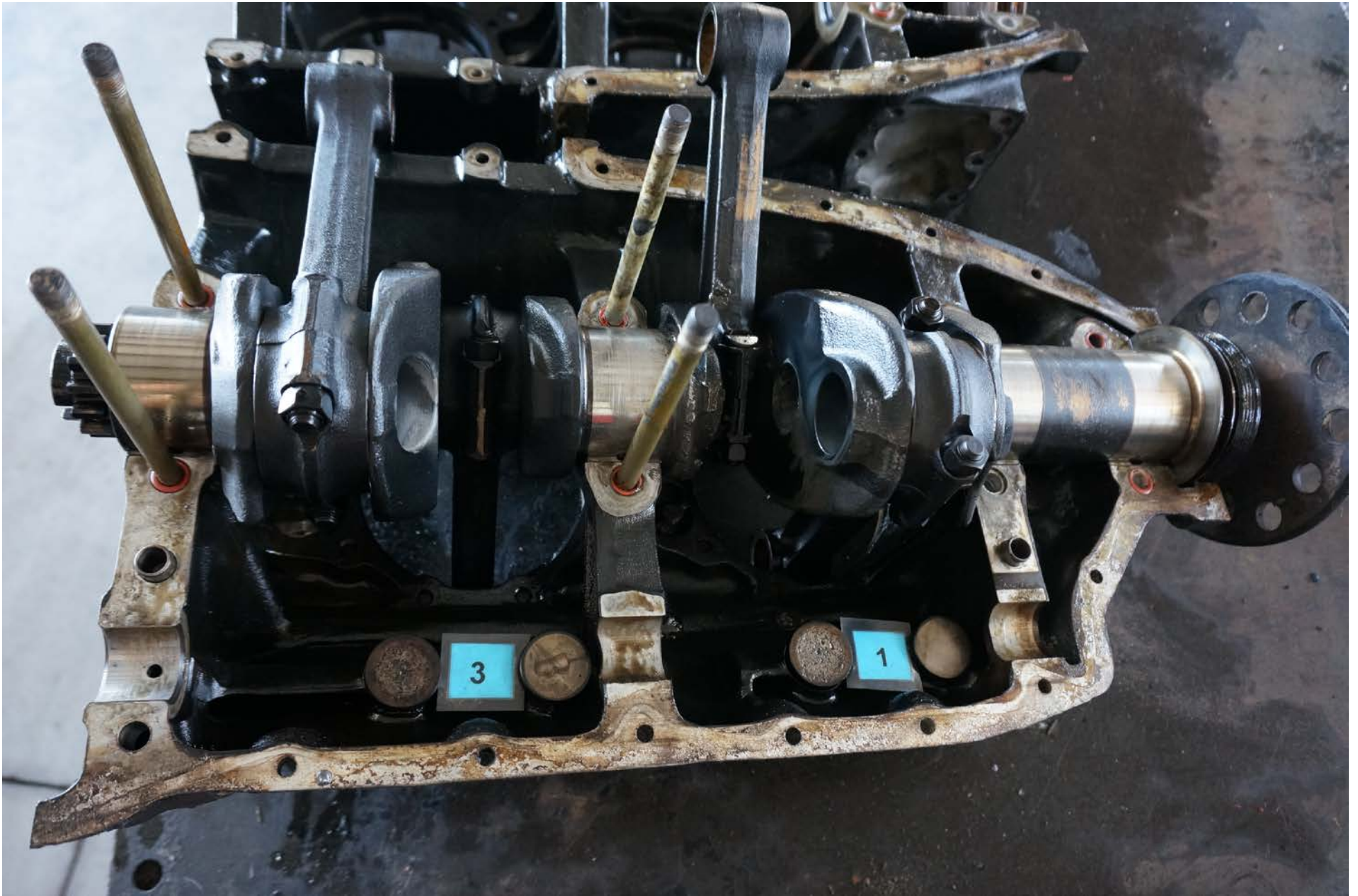
Photo 6 – Other case half displaying spalling of intake valve tappet faces
