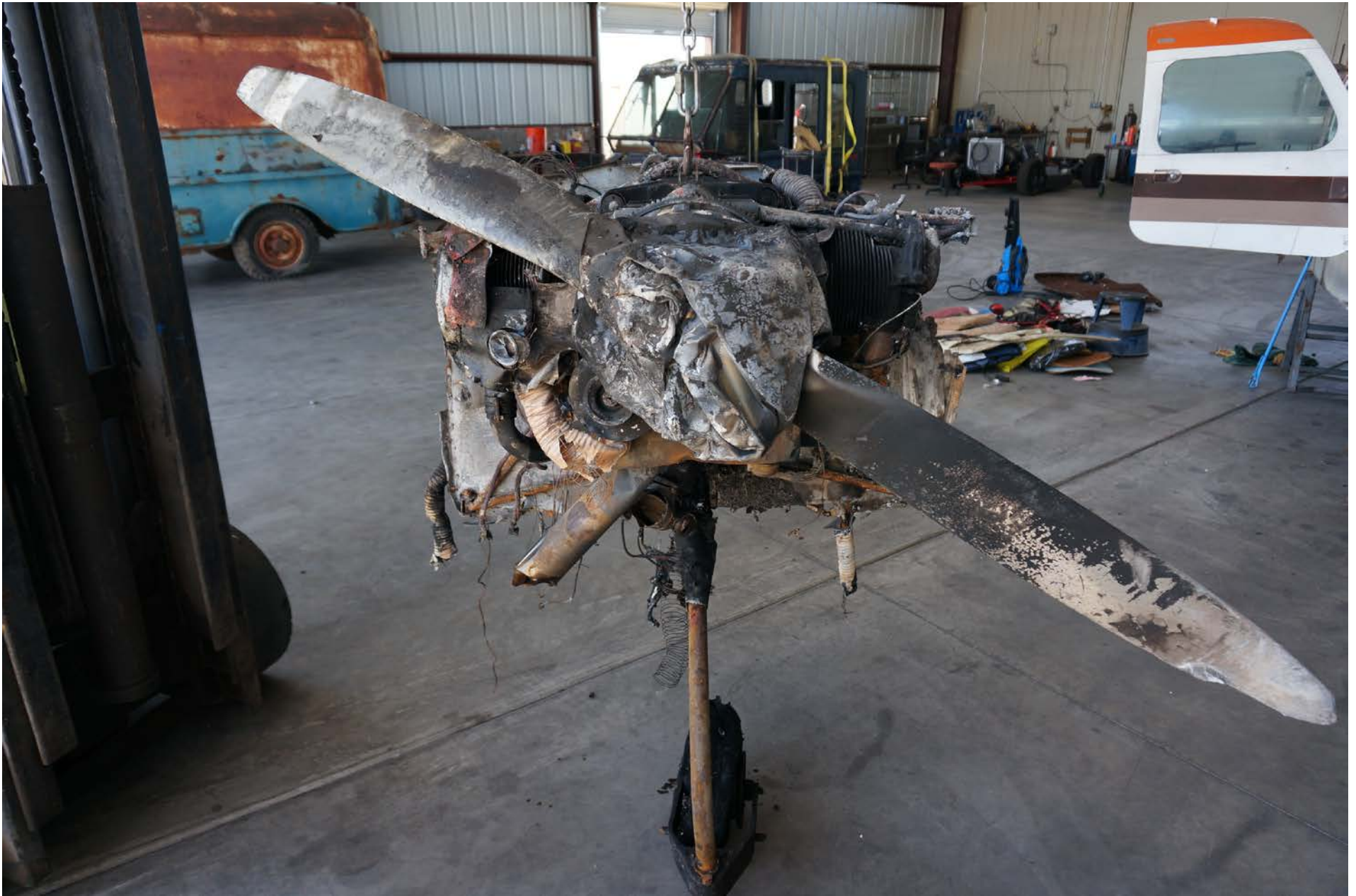
Photo 3 – Engine from front after recovery from accident site
