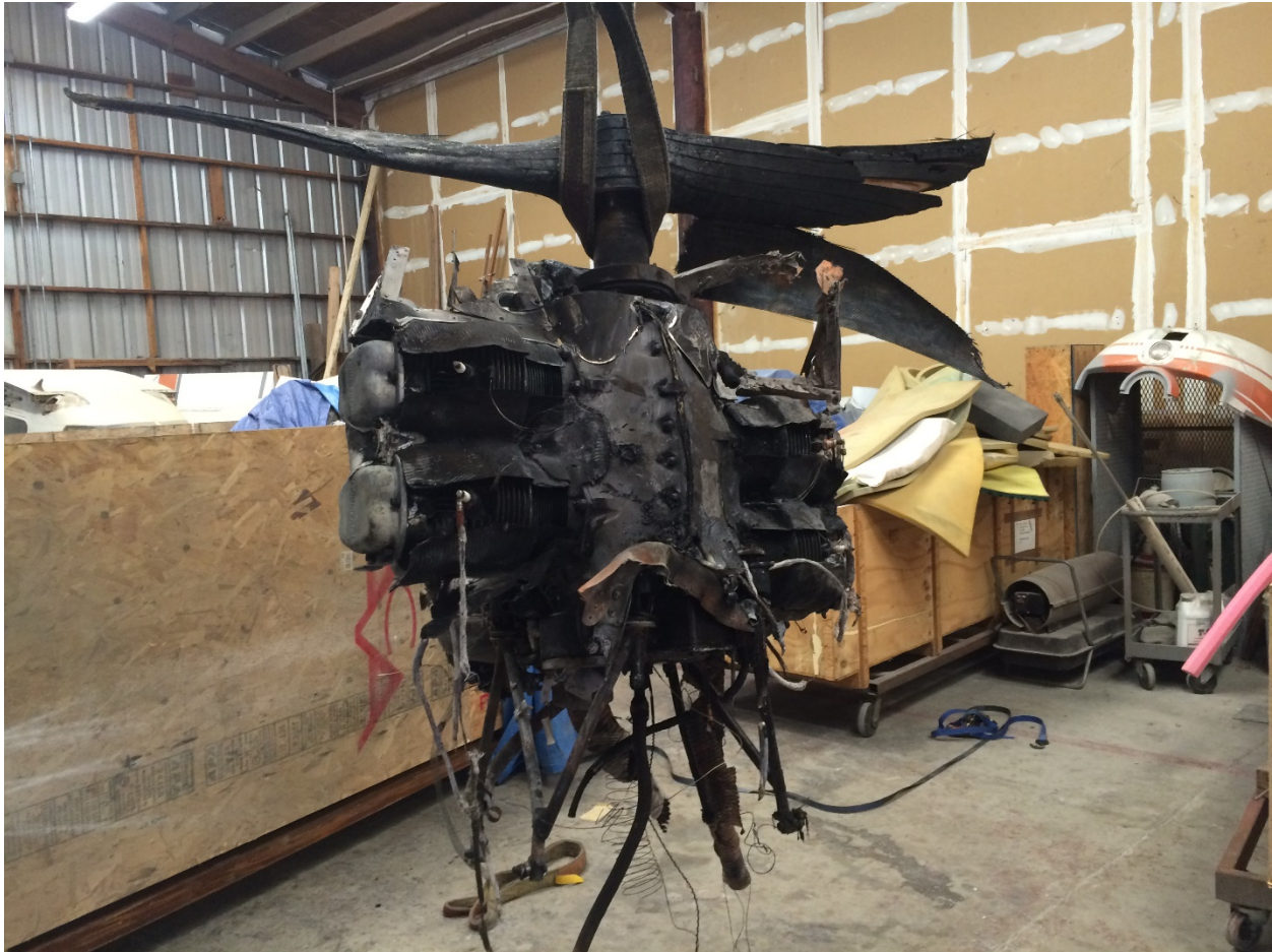
Photo 04 – Top View of Engine (NTSB)
