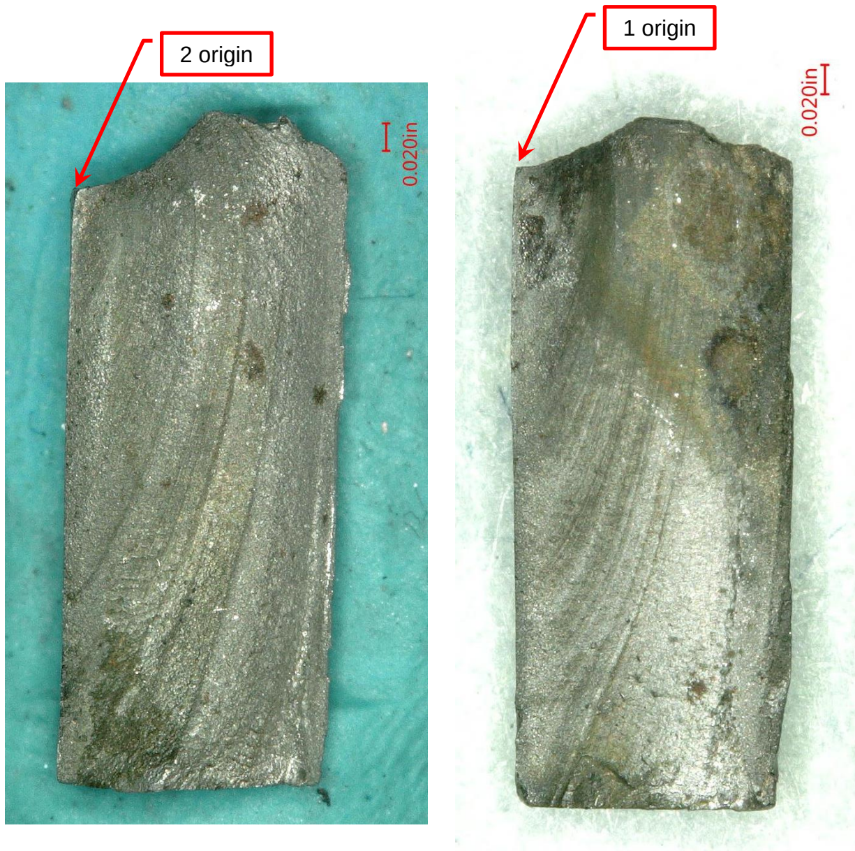
Figure 4 Magnified views of the fracture faces on separated teeth #1 and #2 showing fatigue origins and beach marks. Progression was through almost entire cross section of each tooth.
