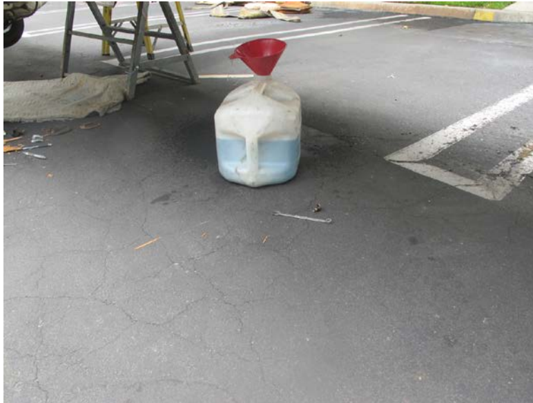
Figure 6 - container of fluid drained from left fuel tank
