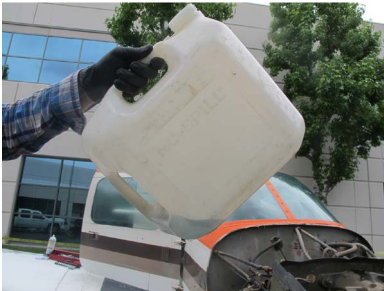
Figure 7 - container with all fluid drained from right fuel tank
