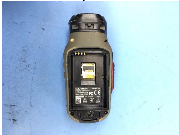
Figure 2. The Garmin VIRB recovered from the wreckage site with the battery cover and battery removed.
