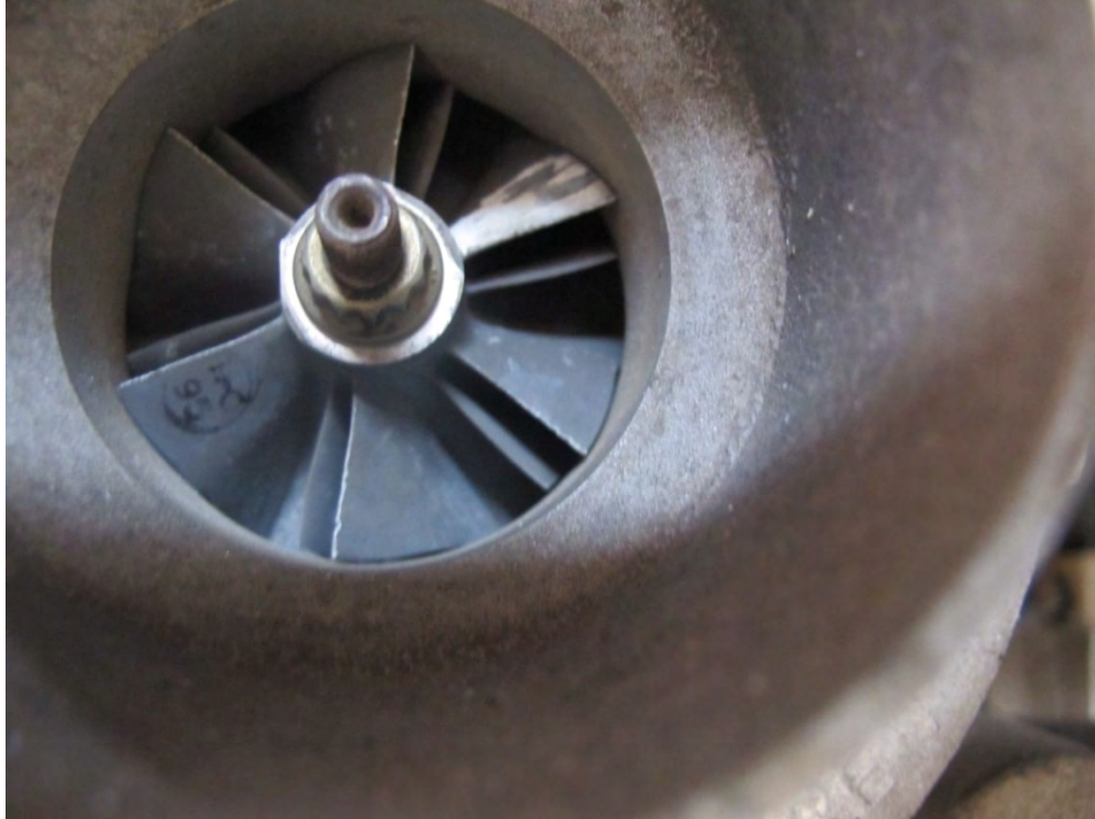
Photo 8 Left Turbocharger Compressor Blades
