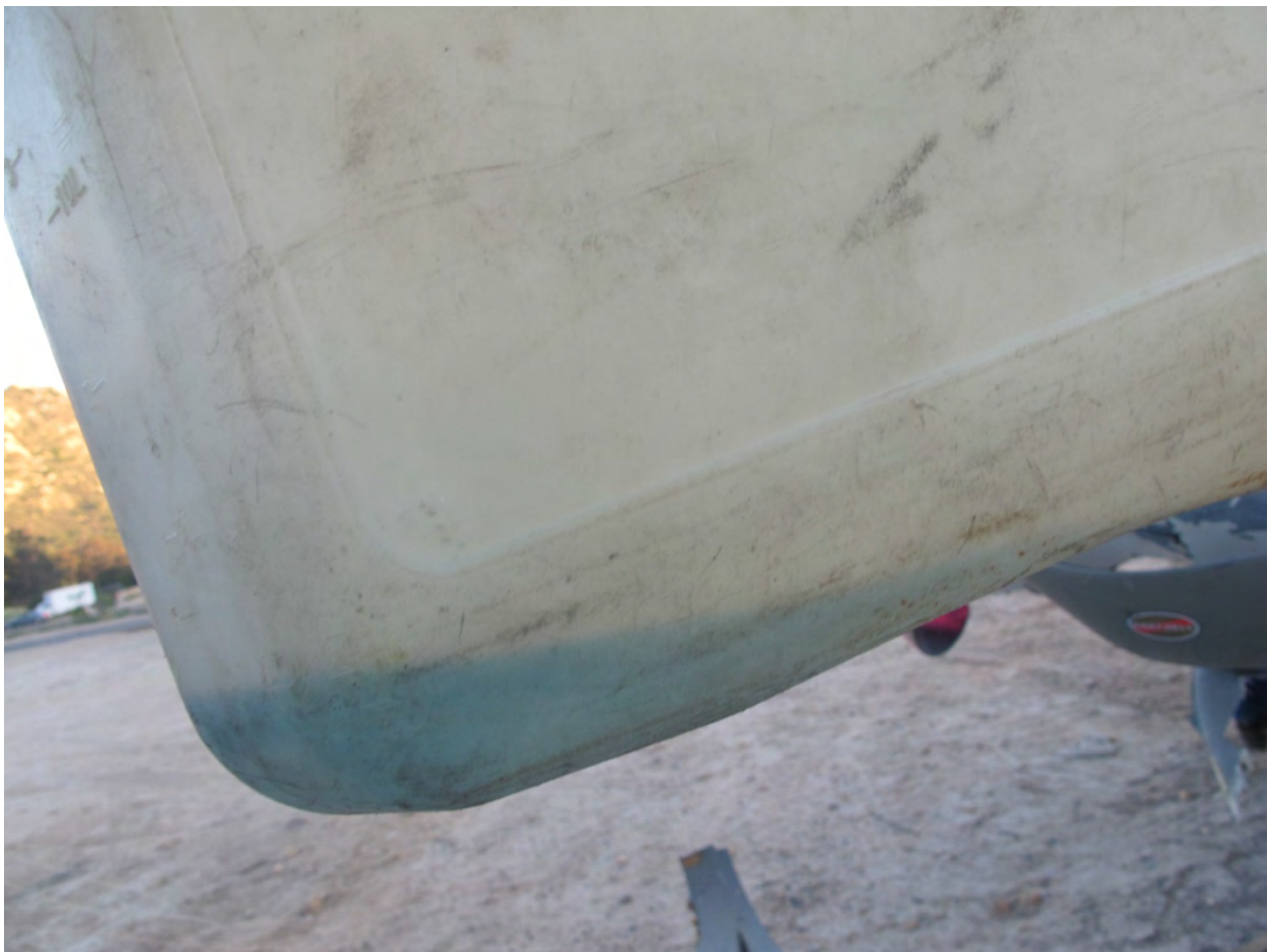
Photo 12 Blue Fluid Drained from Left Wing Root Quick Drain
