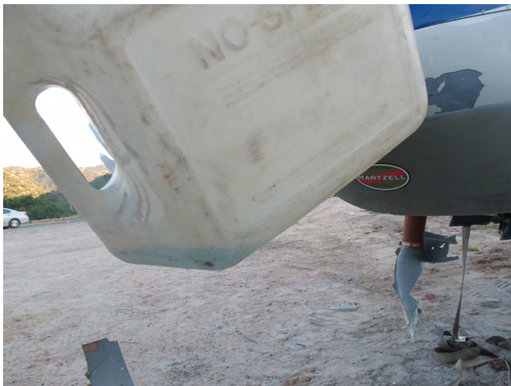
Photo 13 Blue Fluid Drained from Right Wing Root Quick Drain
