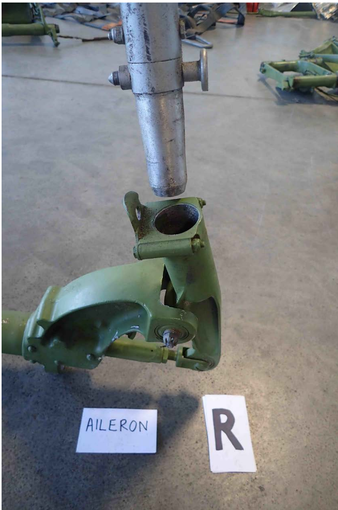
Photo 40 – Rear Control Stick Assembly
