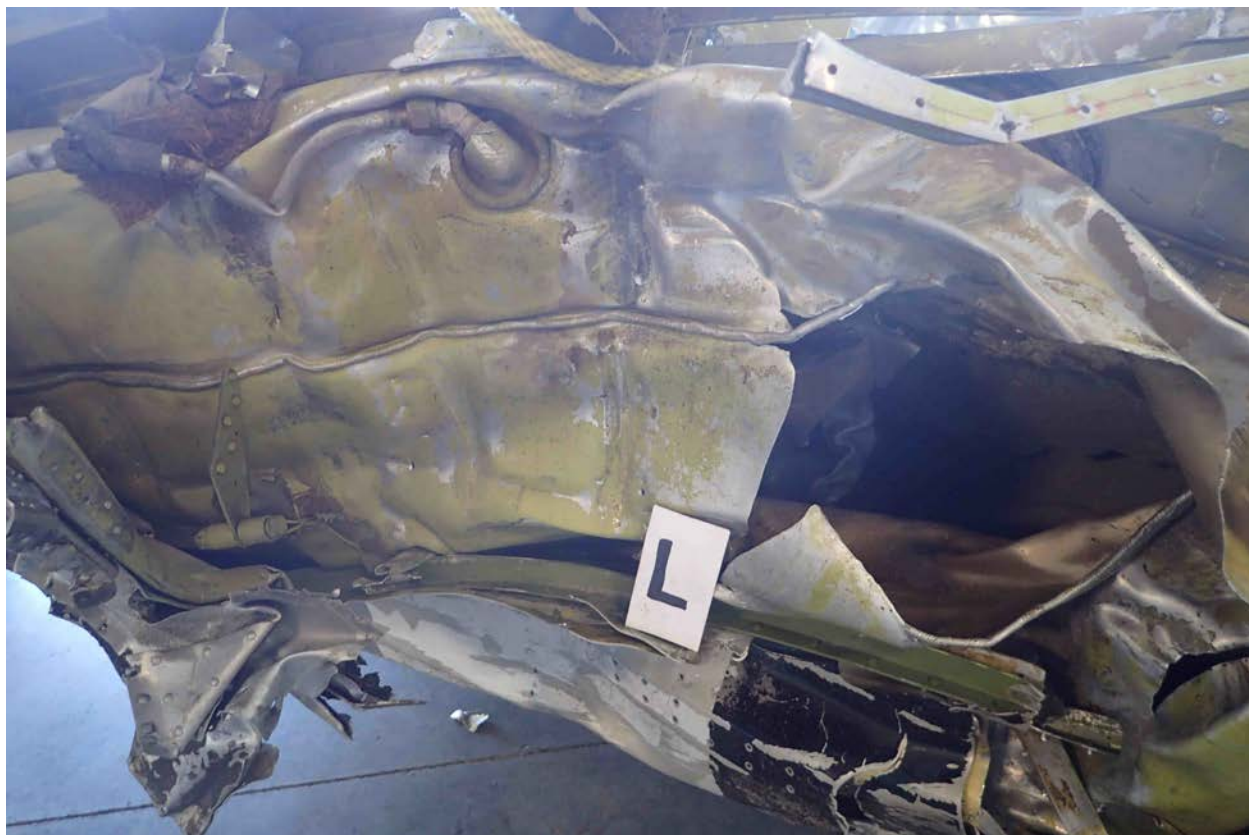
Photo 30 – Left Fuel Tank
