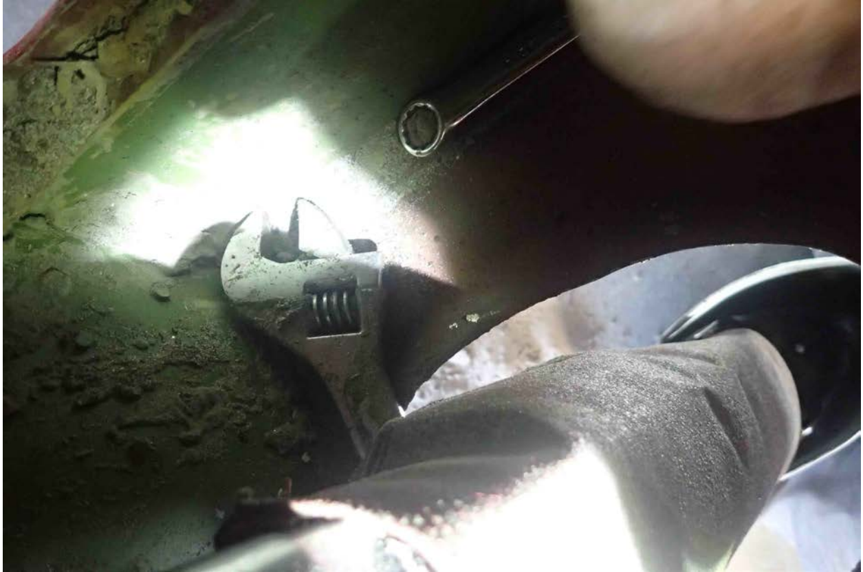
Photo 51 – Tools Found Within Tailwheel Well
