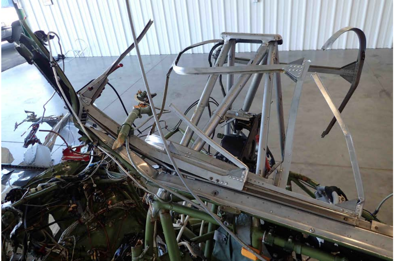
Photo 5 – Canopy Remnants on Left Side of Airframe
