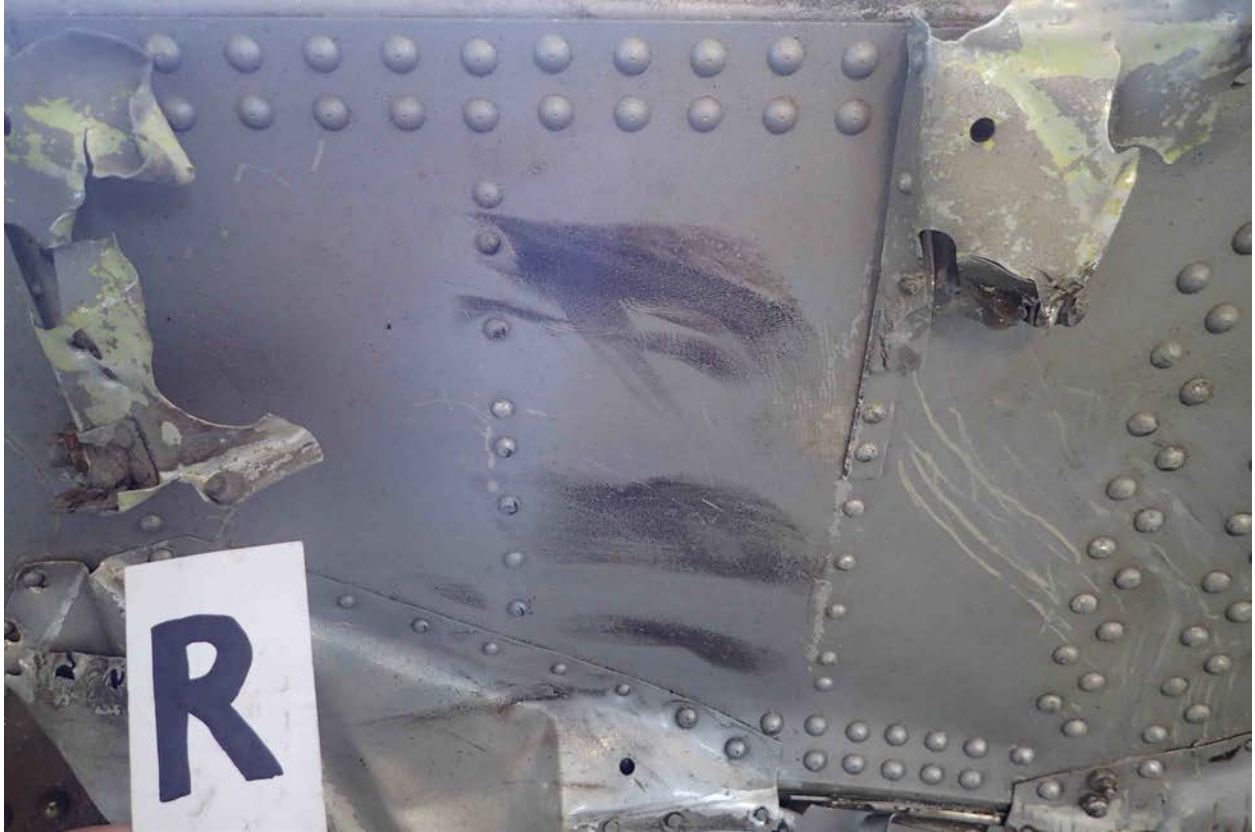
Photo 29 –Transfer Marks in Right Wheel Well
