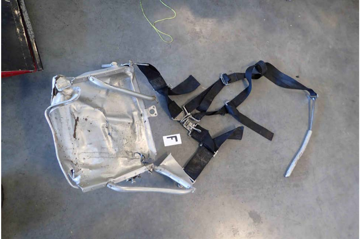
Photo 15 – Front Seat Pan and Belt
