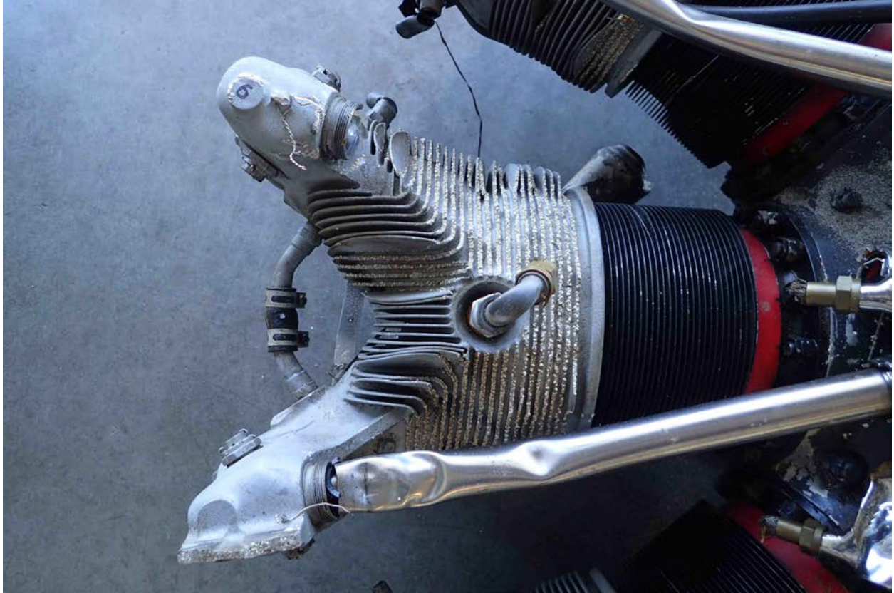
Photo 57 – Forward Fin Damage to Cylinder Head
