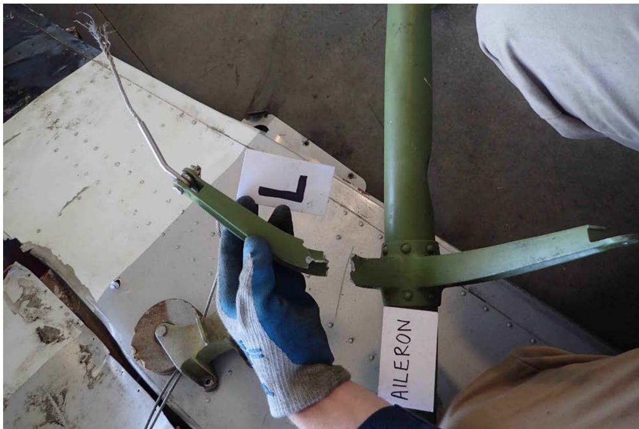
Photo 41 – Aileron Control Arm
