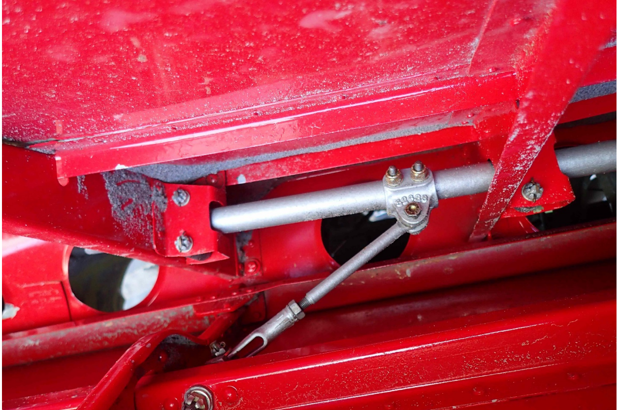
Photo 67 – Flap Extension Pushrod
