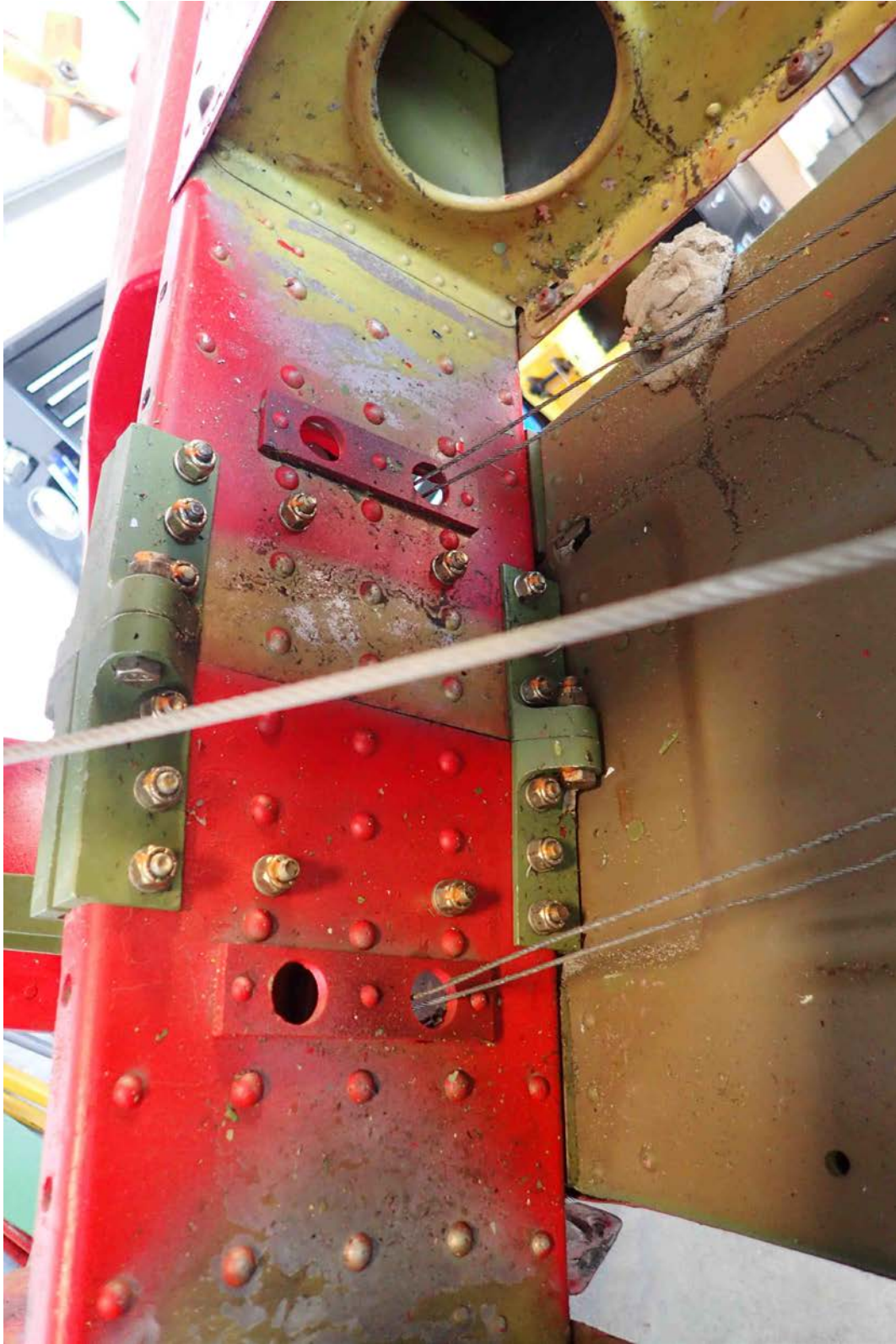
Photo 35 – Horizontal Stabilizer Root Fittings
