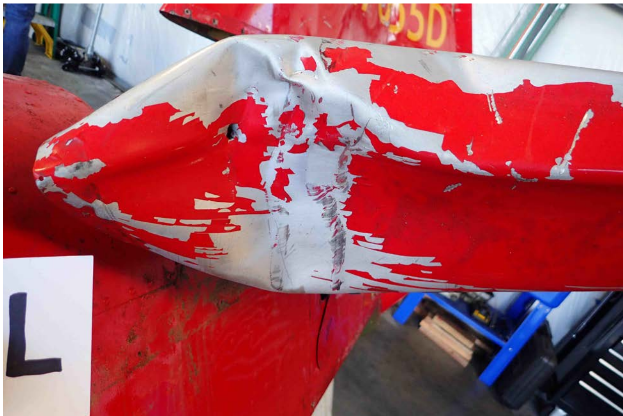
Photo 36 – Left Horizontal Stabilizer Leading Edge
