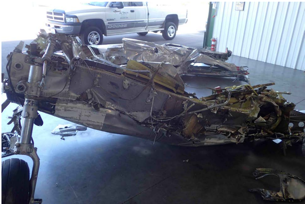
Photo 27 -Right Main Landing Gear
