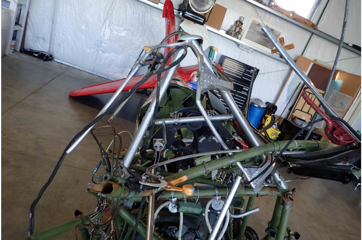
Photo 6 – Canopy Remnants Wrapped around A-Pillar
