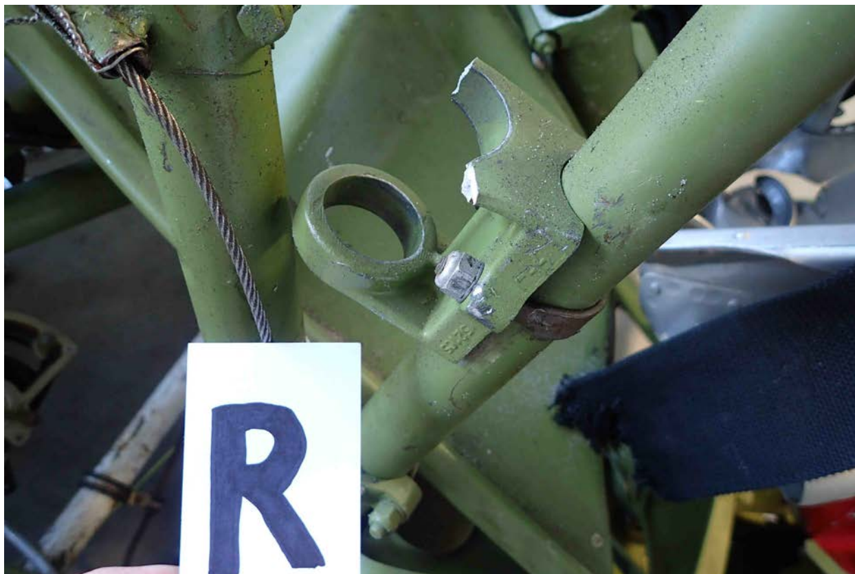
Photo 13 – Rear Control Stick Storage Dock
