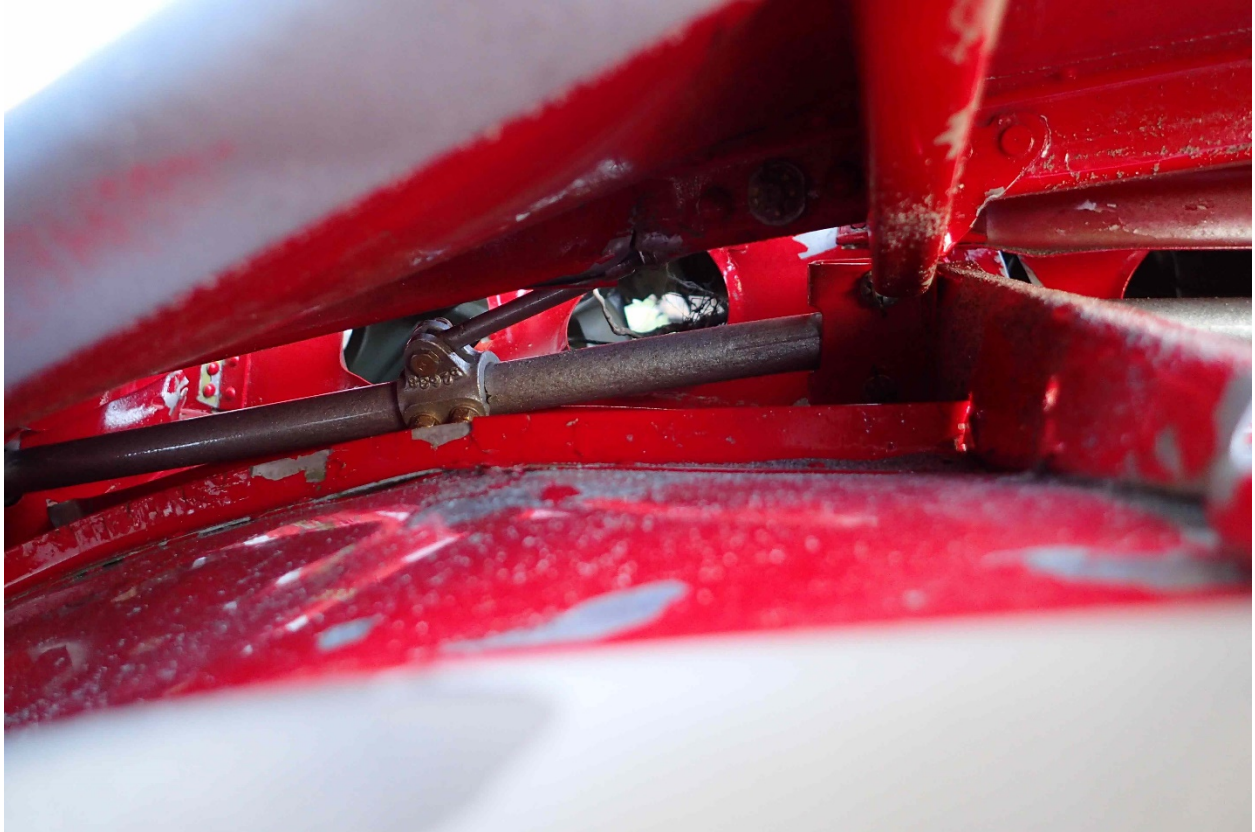
Photo 68 - Flap Extension Pushrod
