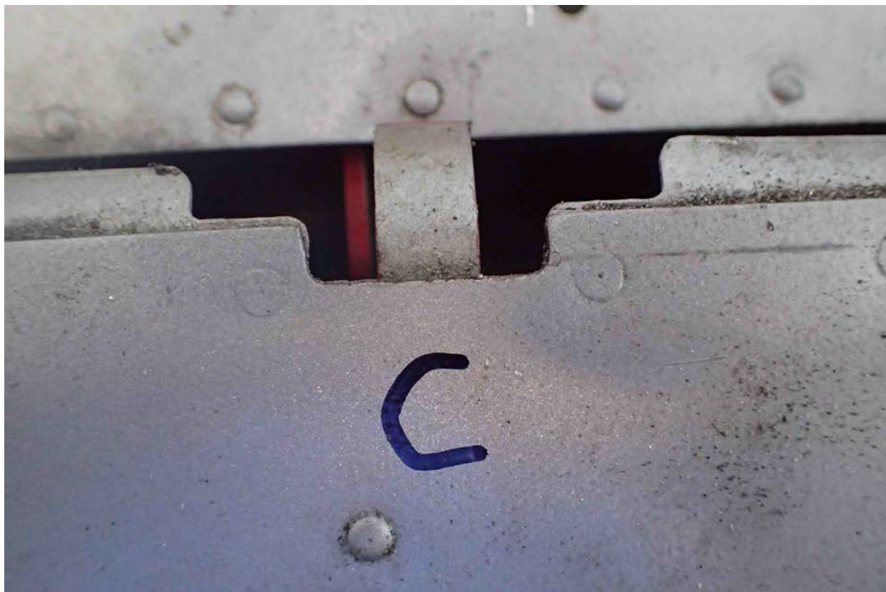
Photo 32 – Center Flap Hinge
