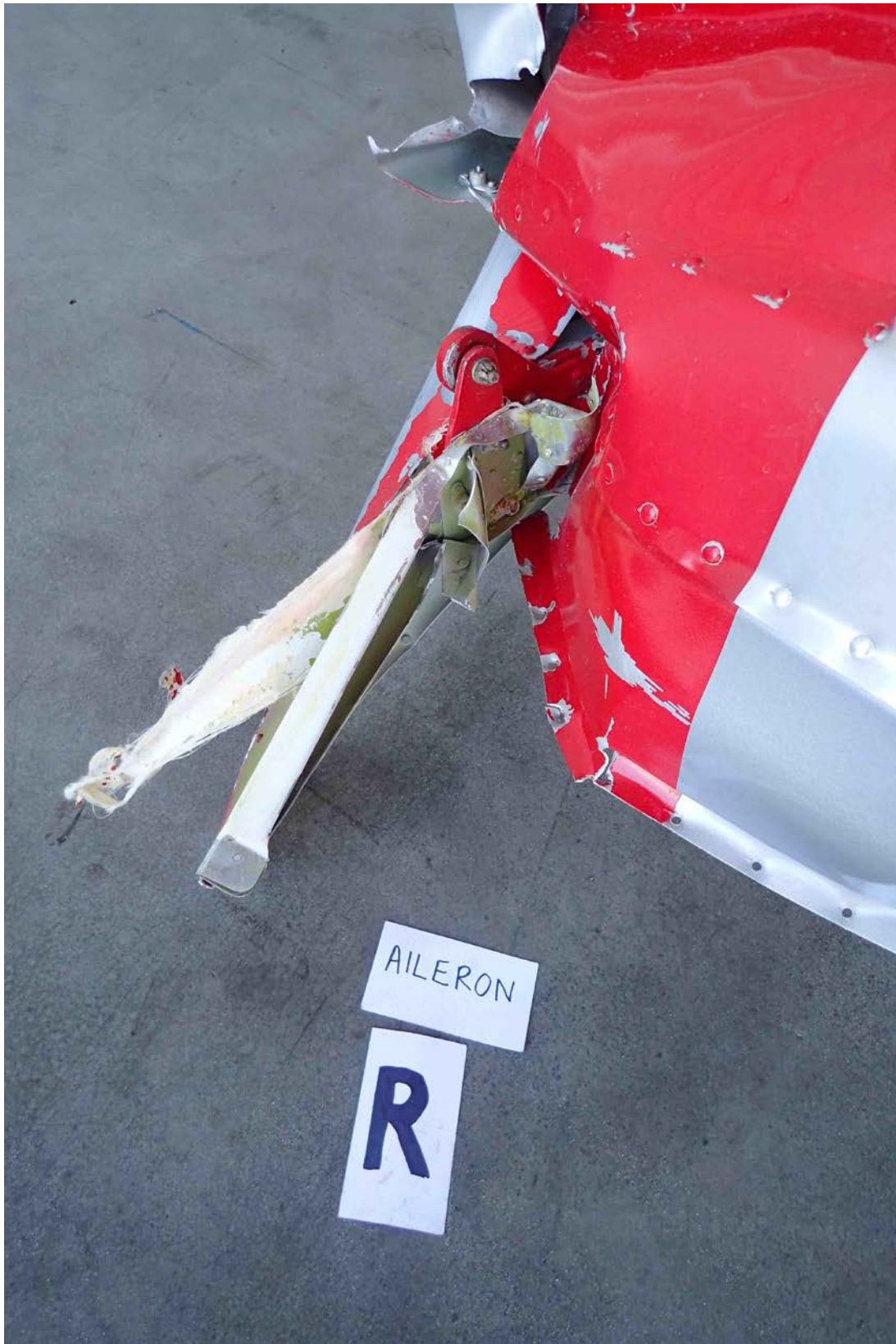
Photo 46 – Right Aileron Remnants
