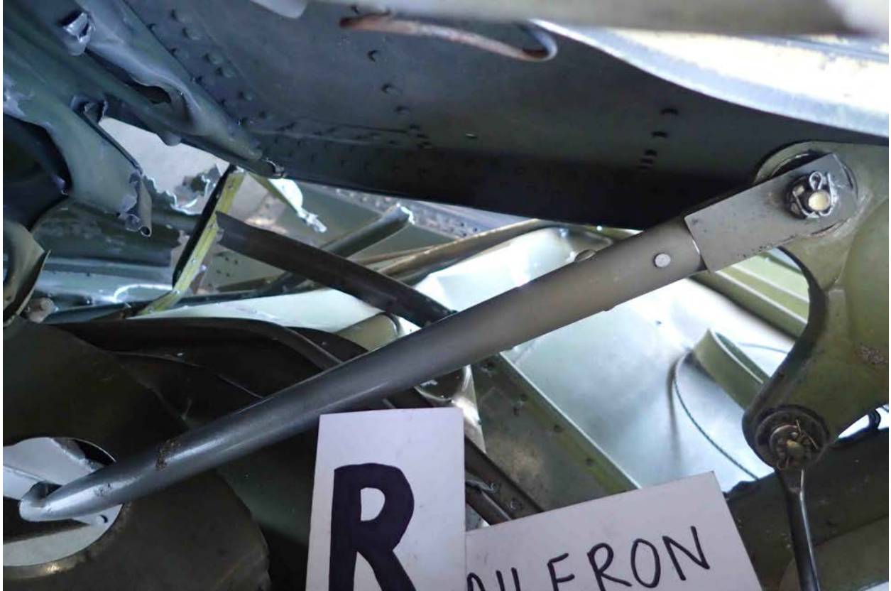
Photo 45 – Right Wing Aileron Bellcrank
