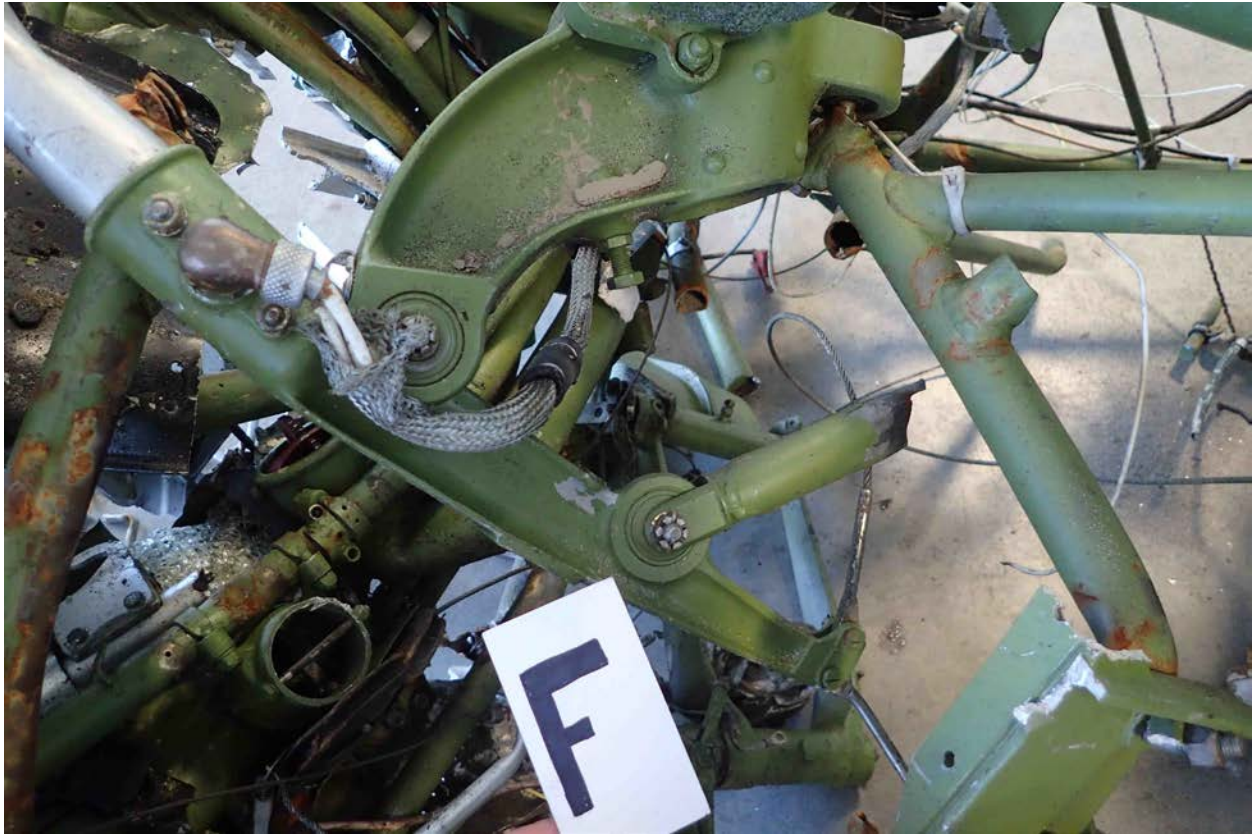
Photo 16 – Forward Control Stick Assembly
