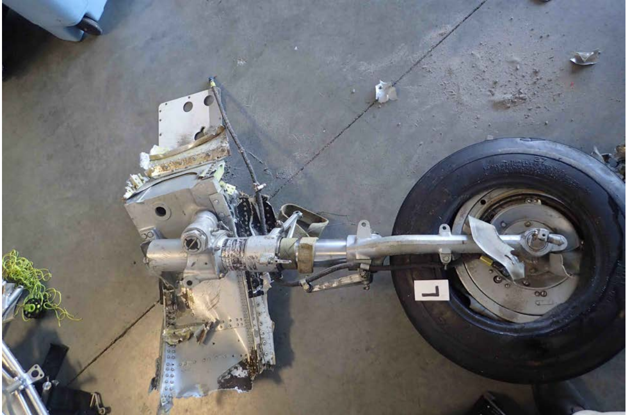
Photo 28 – Left Main Landing Gear
