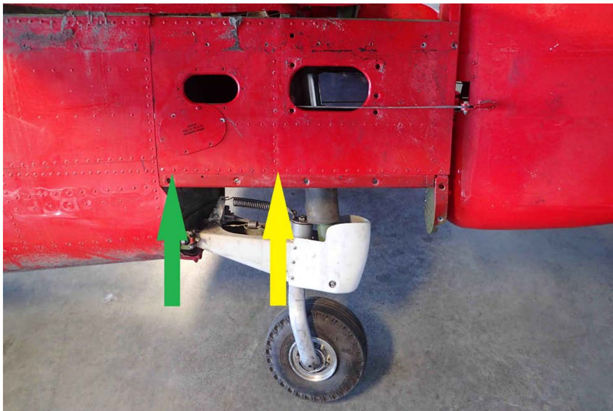
Photo 53 – Location of Tools Found in Tailwheel Well
