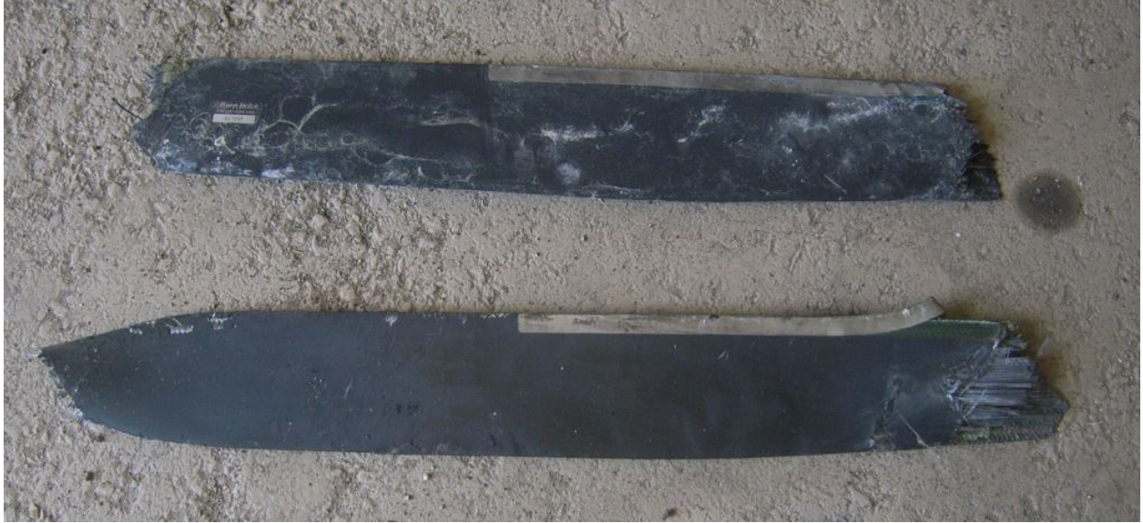
Figure 36 - Two Fractured Propeller Blades
