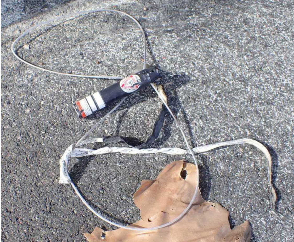
Figure 16 - Airframe Parachute Extraction Rocket
