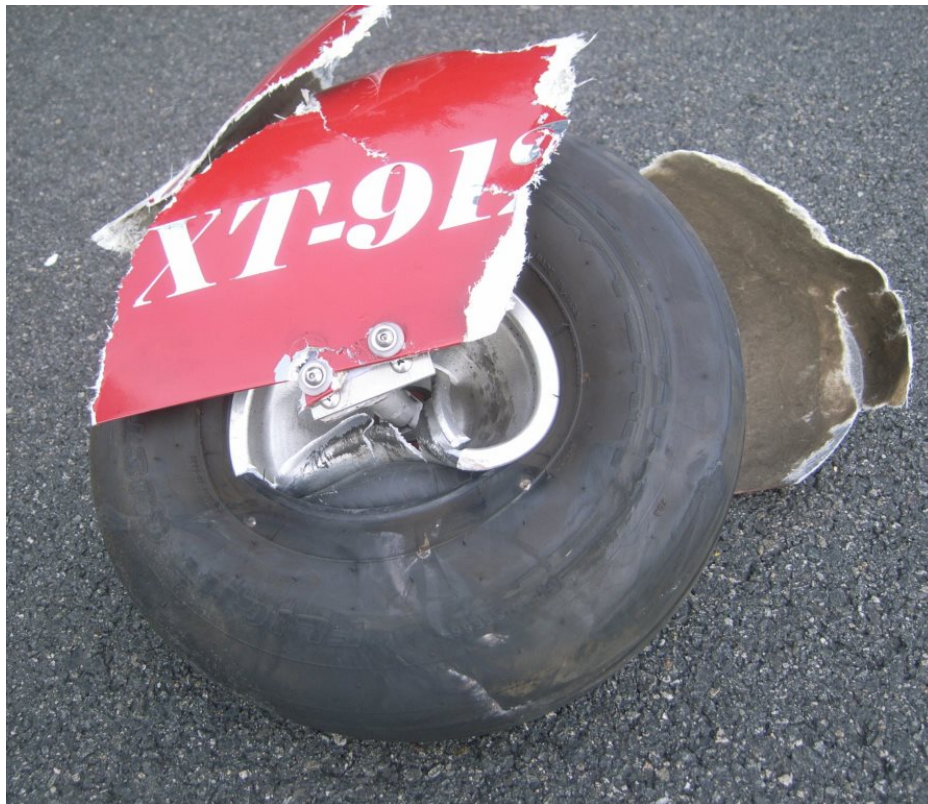
Figure 19 - Outboard Side of Right Wheel Assembly (note damage)
