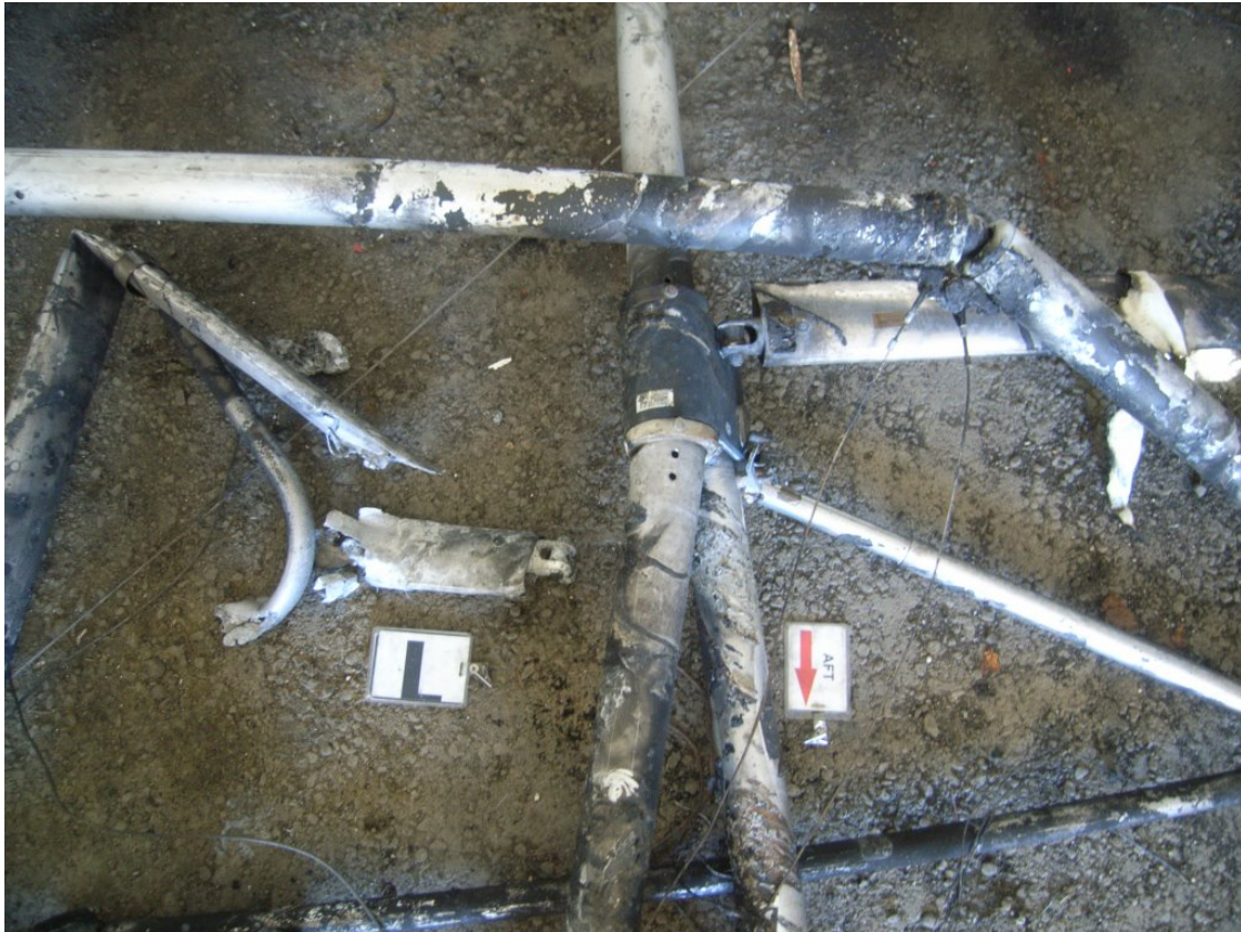
Figure 28 - Wing/Frame Pivot Location
