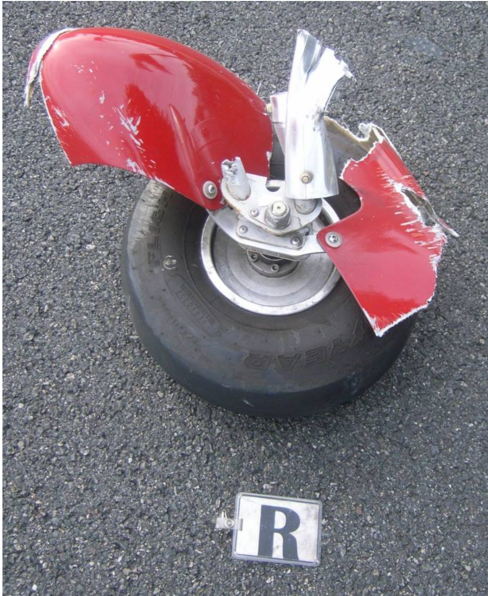
Figure 20 - Inboard Side of Right Wheel Assembly
