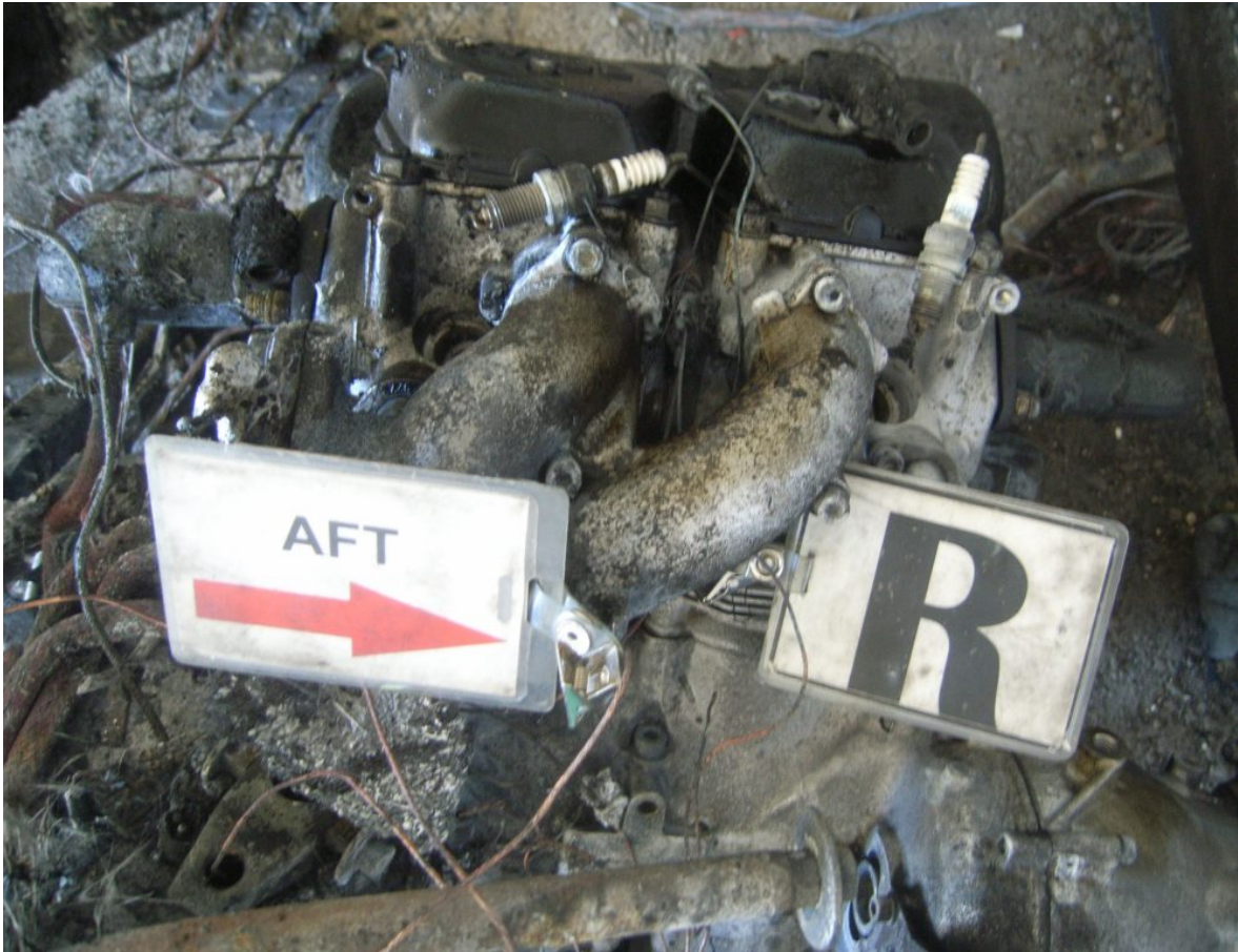
Figure 40 - Right Cylinder Bank with Spark Plugs
