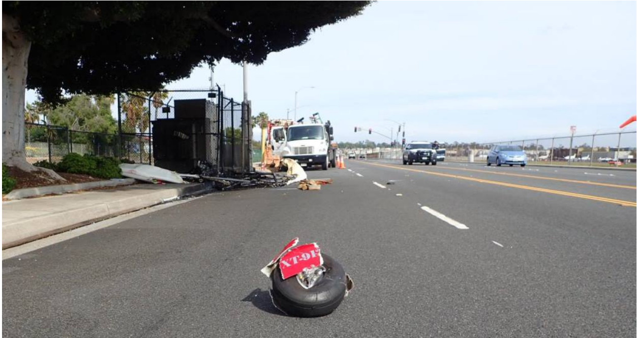
Figure 18 - Right Main Wheel Assembly
