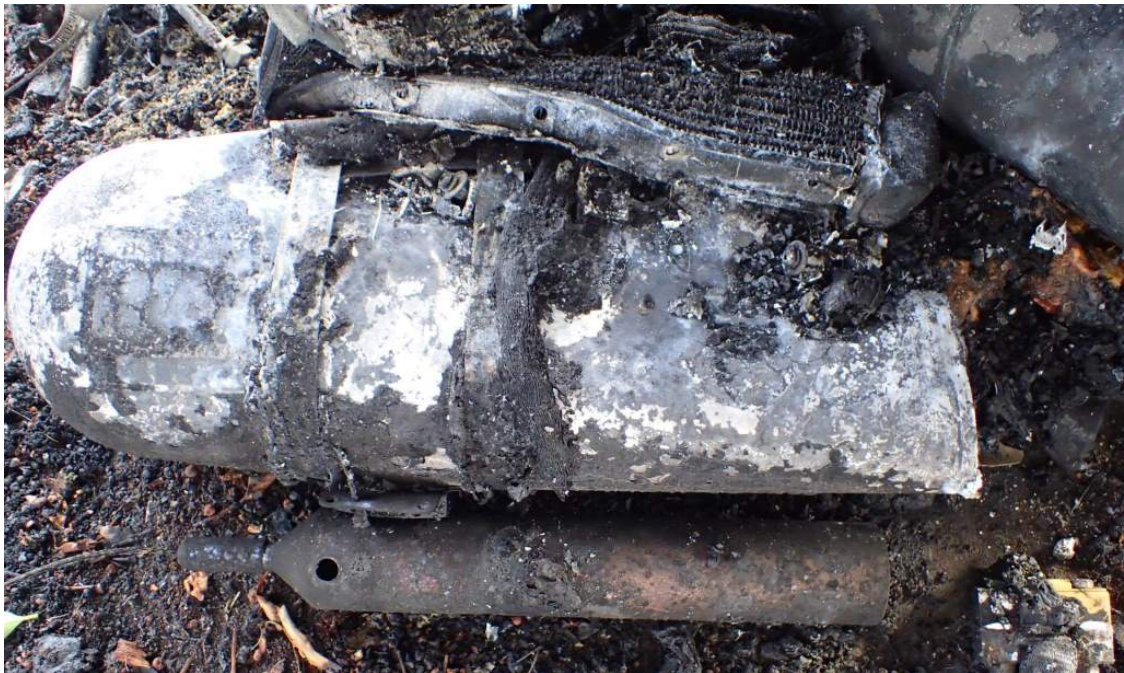
Figure 17 - Parachute (top) and Rocket (bottom) Cases
