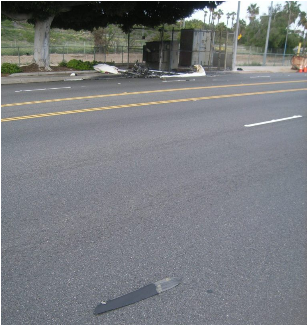
Figure 35 As-Found Fractured Propeller Blade
