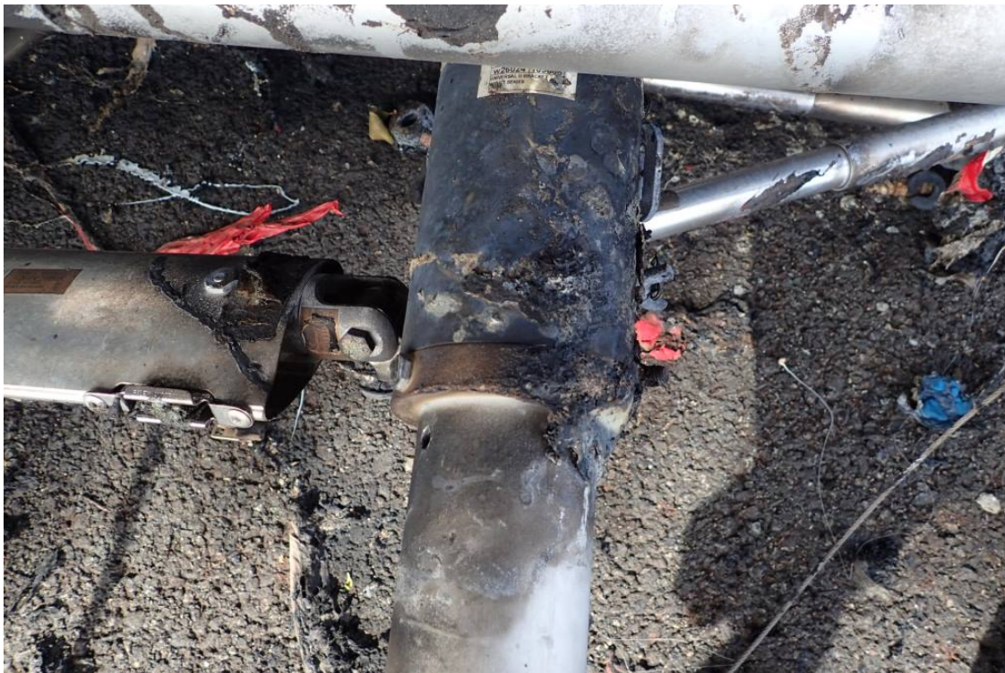
Figure 29 - Wing Strut Juncture (note fractured left upper attach; looking aft)
