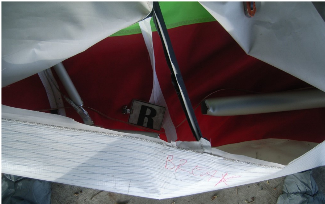
Figure 27 - Right Wing Tip (sail opened to show spar break)
