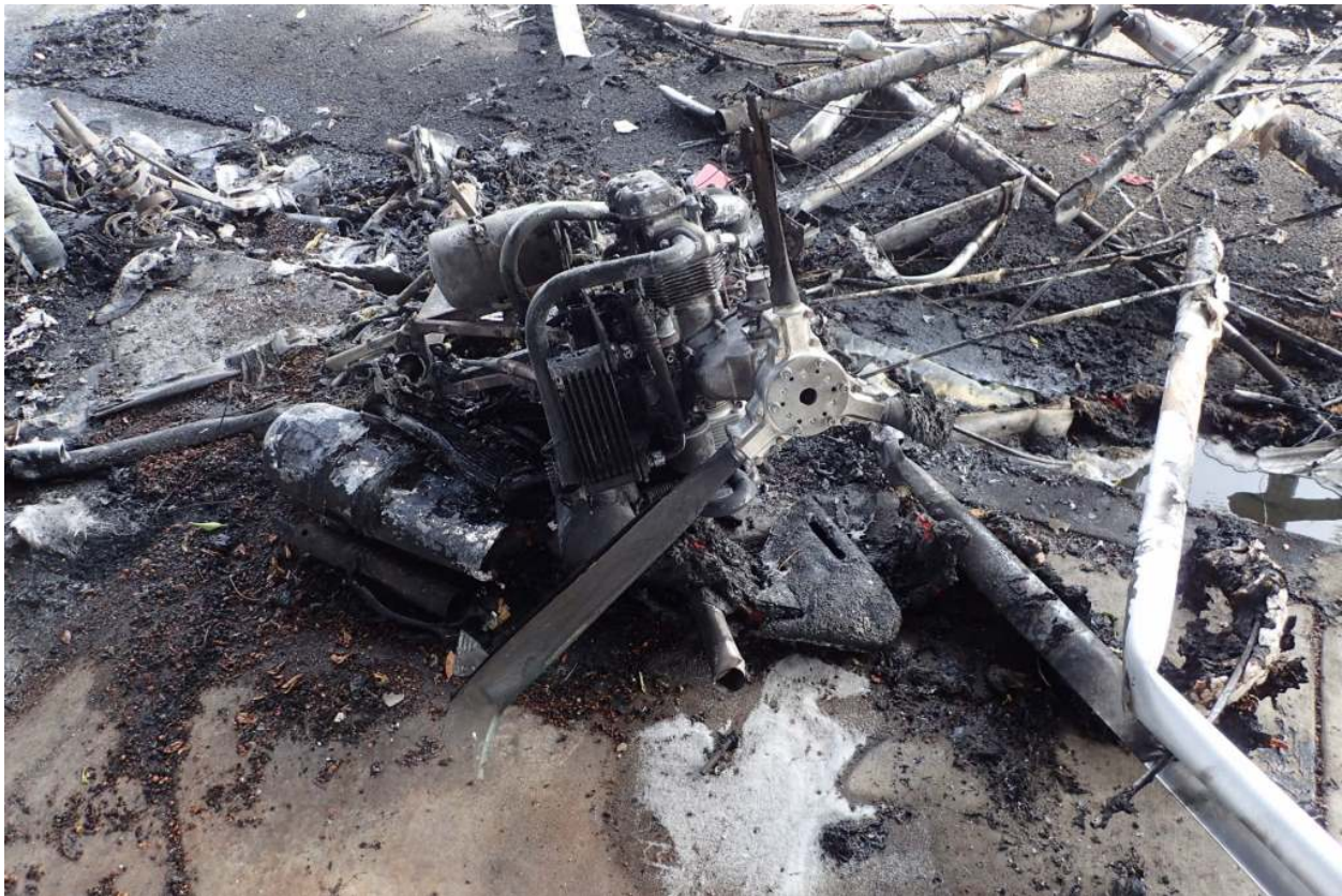
Figure 34 - Engine in Wreckage
