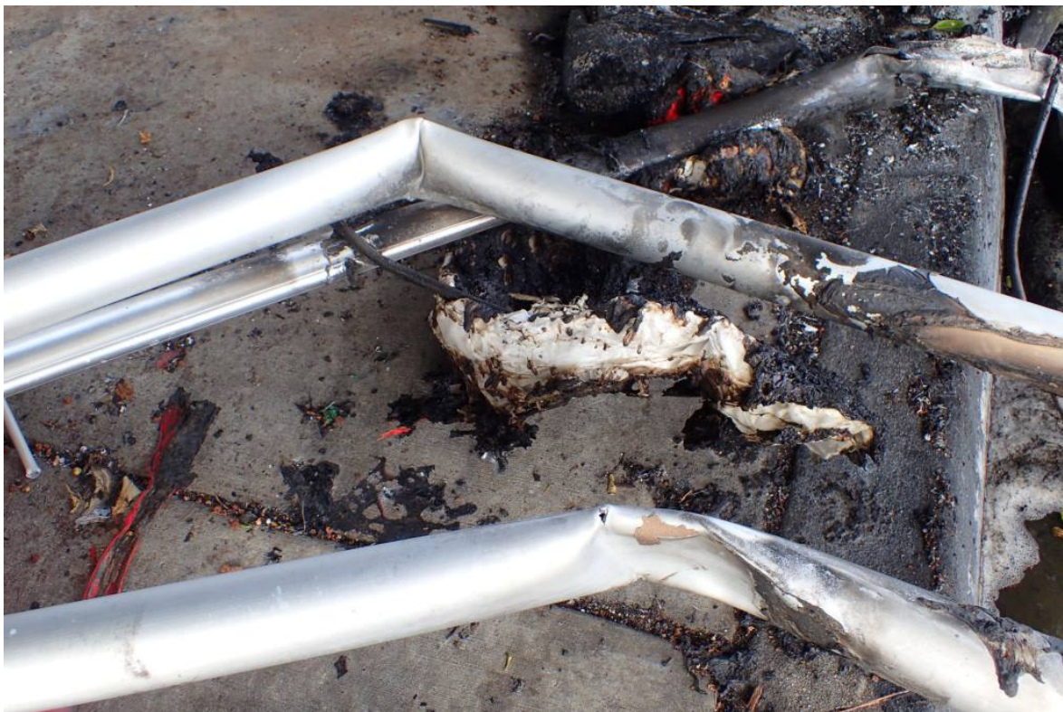
Figure 25 - Right Wing LE Spar (bottom) and Aft Spar (top)
