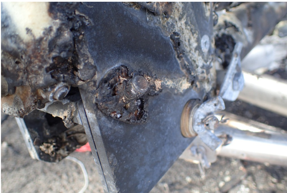
Figure 32 - Fractured Upper Left Strut Attach
