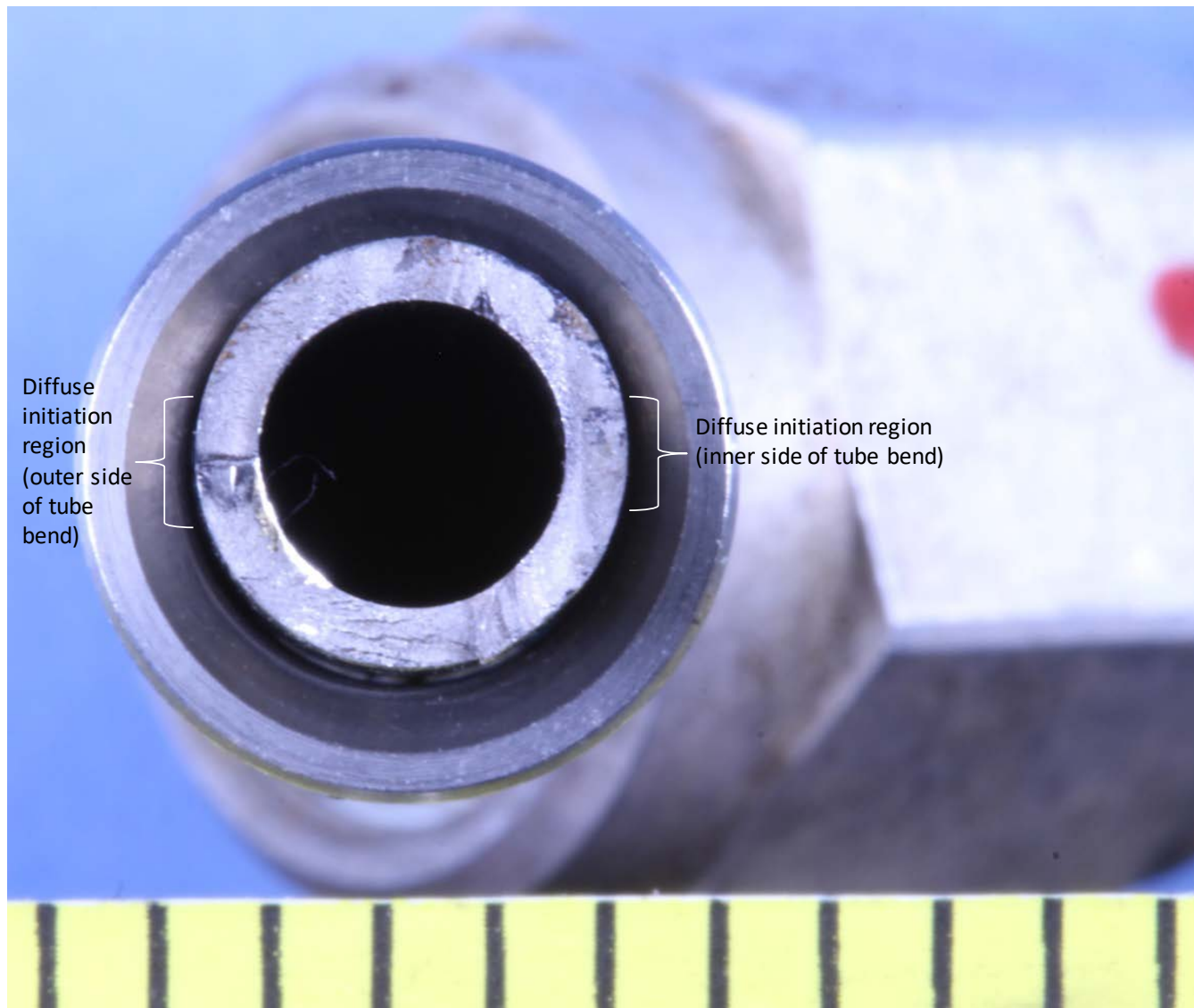
Figure 3 Close view of the fractured end of the fuel line tube with the fracture initiation regions identified.
