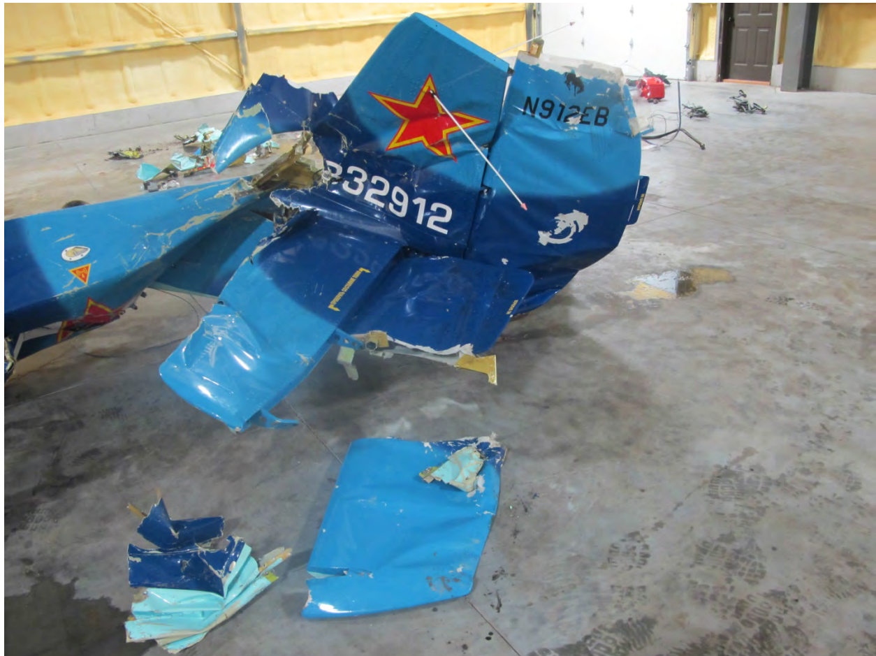
Figure 7. Left Side of the Empennage
