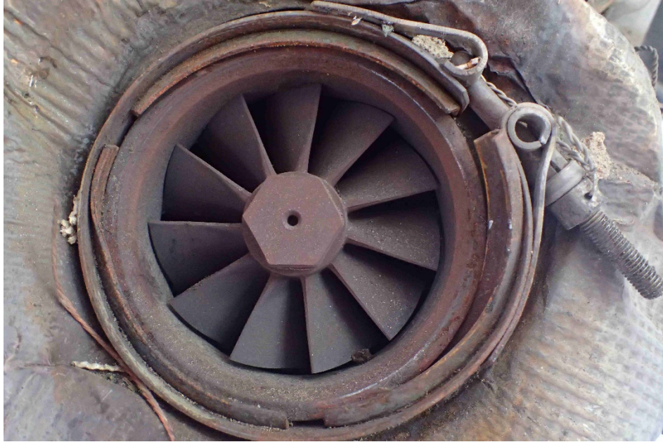
Photo 5 – Turbo Charger Turbine Wheel
