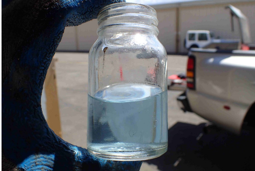
Photo 7 – Fuel From Fuel Selector Valve
