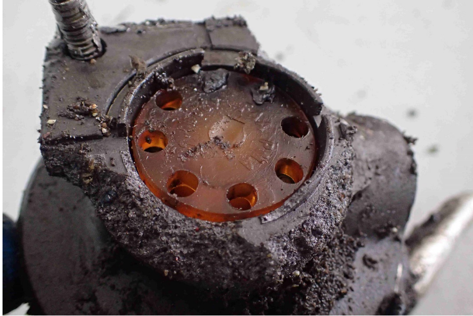
Photo 9 – Primary Vacuum Pump Drive Coupling
