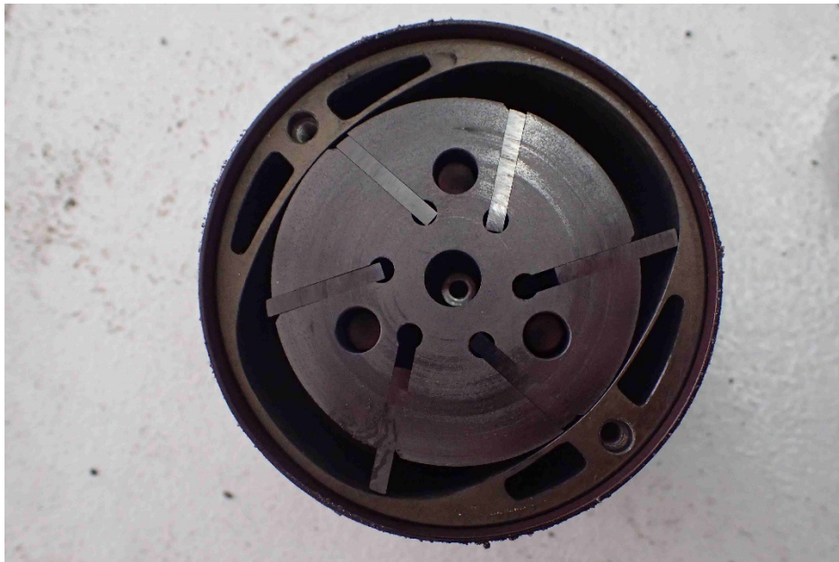
Photo 13 - Secondary Vacuum Pump Vanes and Rotor
