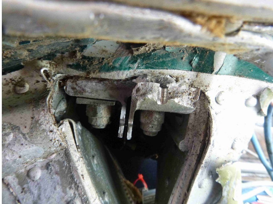
Photo 11 – Right Wing Main Spar Upper Web
