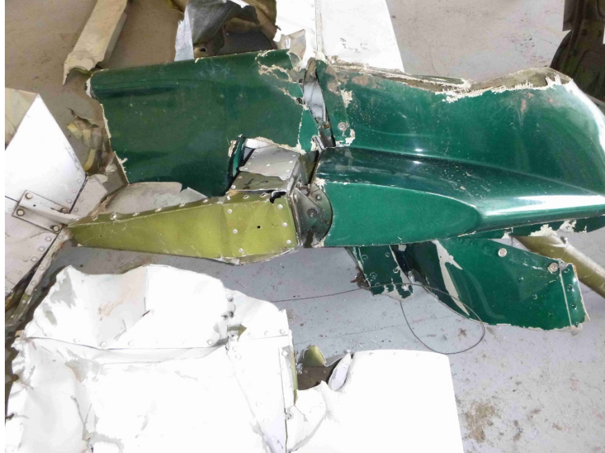
Photo 20 – Rudder Upper Hinge
