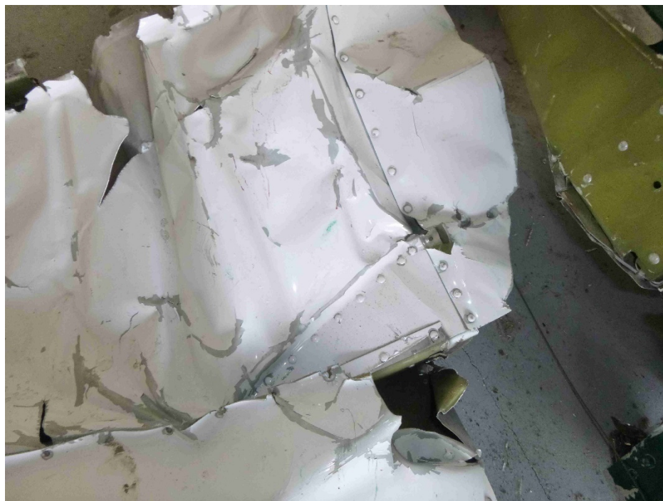
Photo 17 – Green Paint Transfer Marks Upper Inboard Right Stabilator Skin
