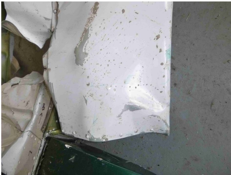
Photo 19 - Green Paint Transfer on Left Stabilator Upper Leading Edge
