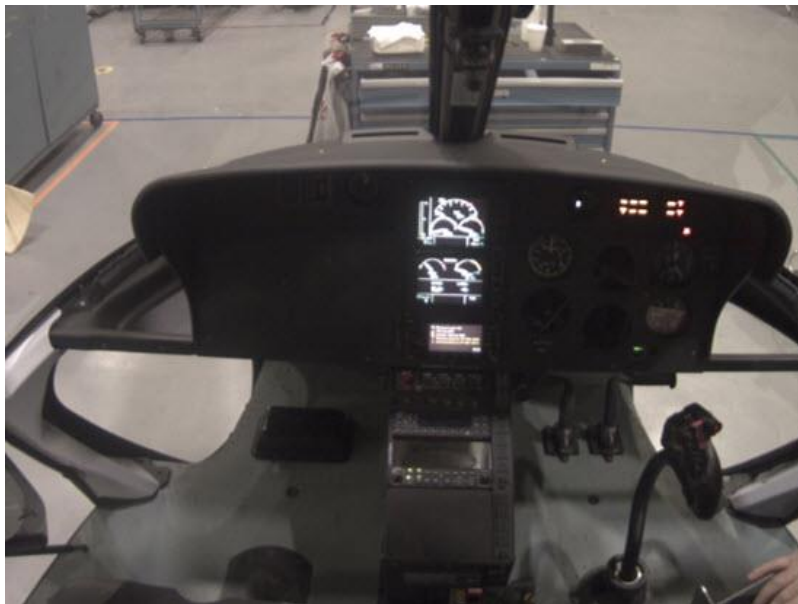
Figure 1. The Appareo Vision 1000's field of view as mounted on the accident rotorcraft during the accident flight.
