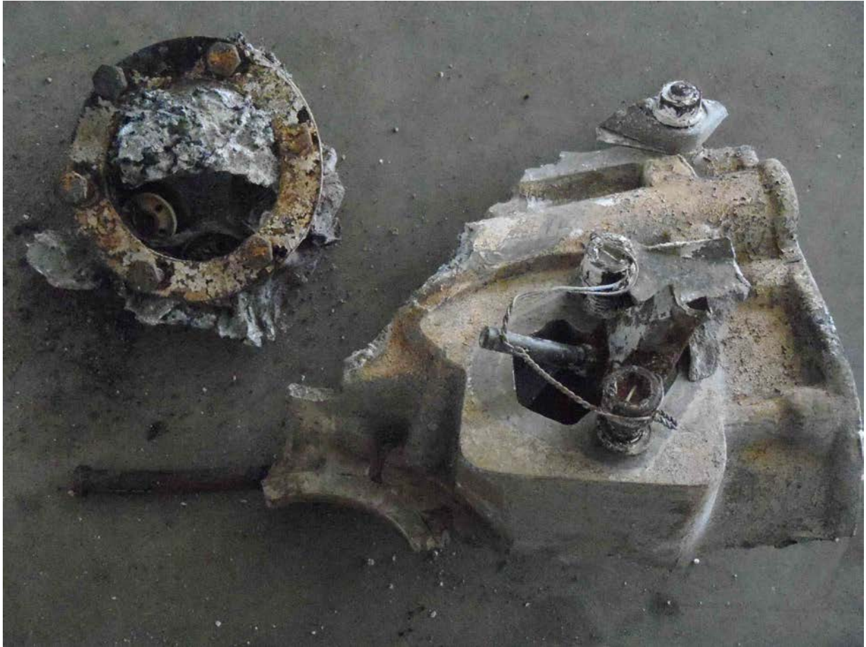
Photo 17 - Engine Driven Fuel Pump Remnants
