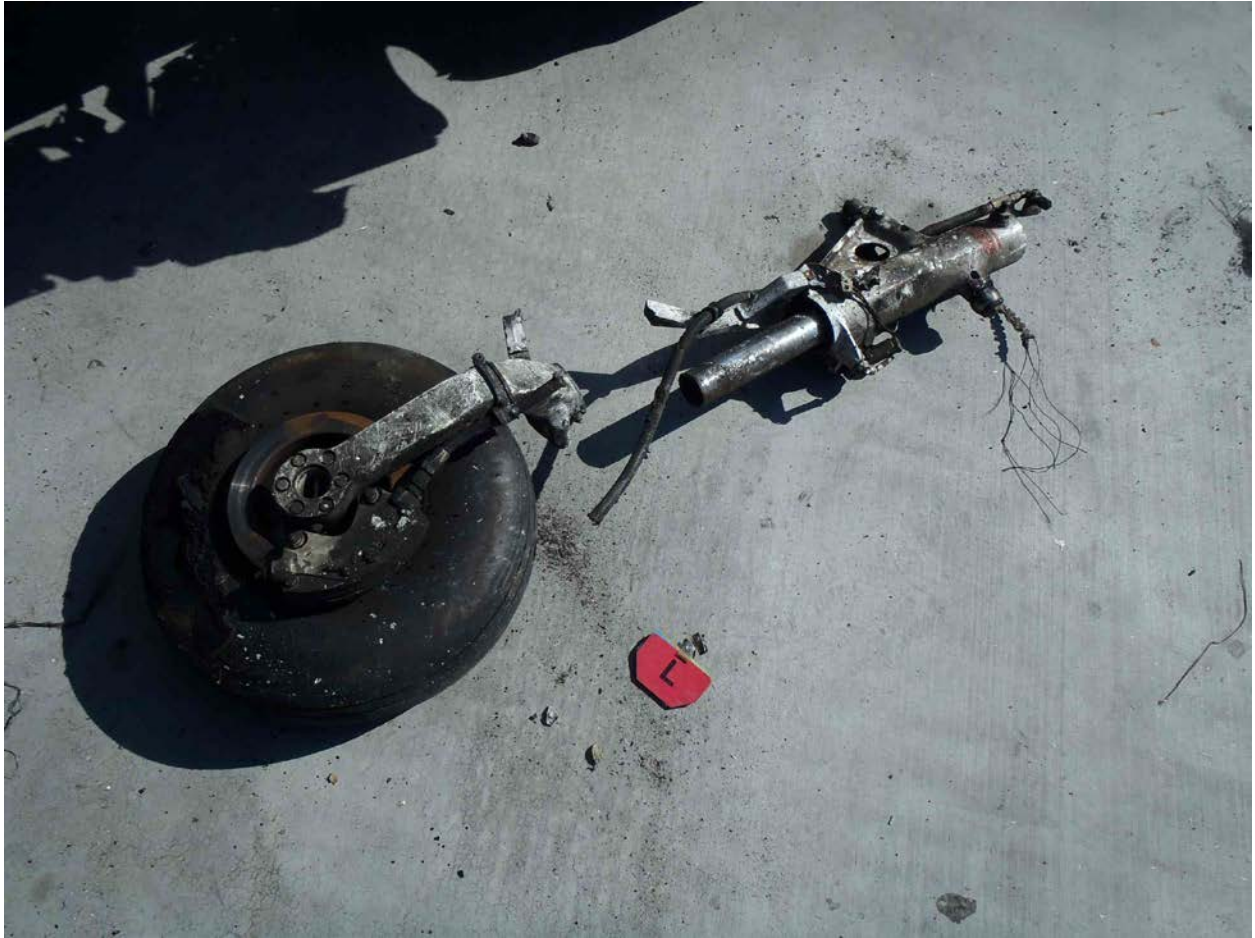
Photo 9 - Left Main Landing Gear
