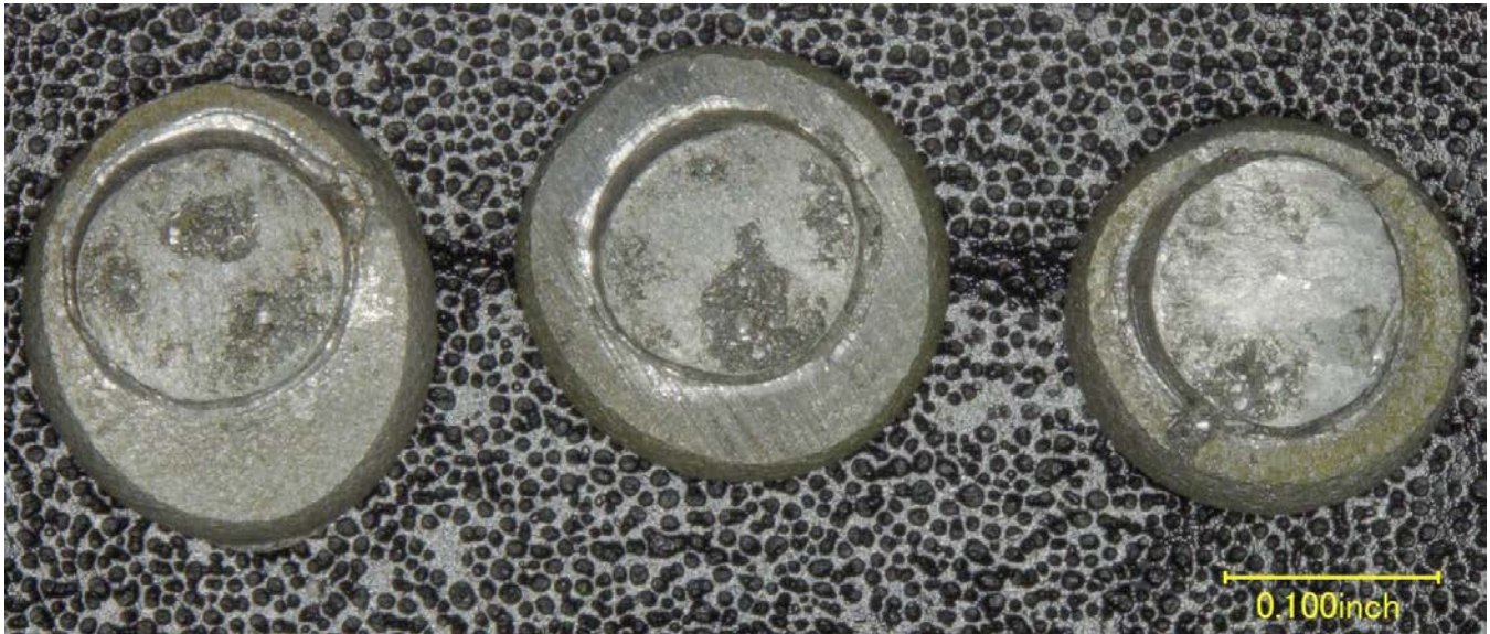
Figure 2 – The fracture surfaces of tails of rivets 1 through 3, as received.
