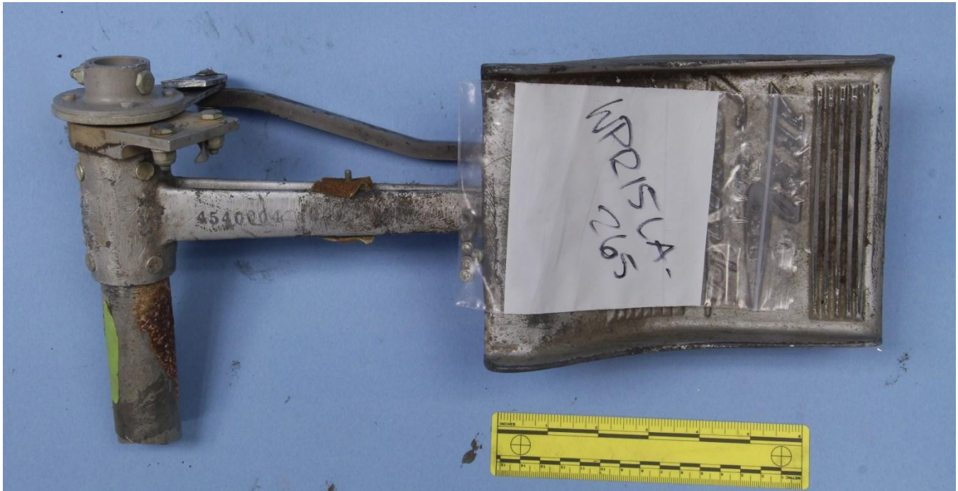
Figure 1 – The rudder control pedal and bagged rivet tails, as received.
