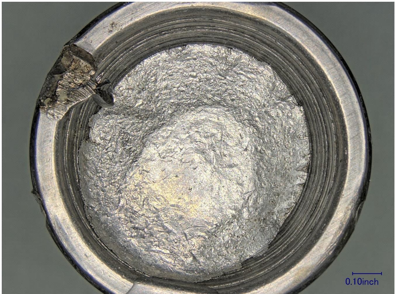
Figure 9 – Closer view of the pin fracture surface from Figure 8.
