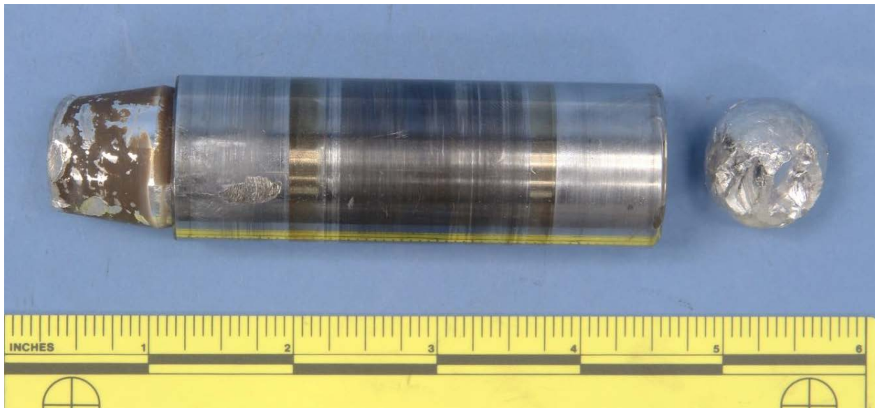
Figure 7 – The piston pin, as received. The left side of the pin exhibited batter on the plug, while the right side plug fragment had separated and been deformed into a spherical shape.
