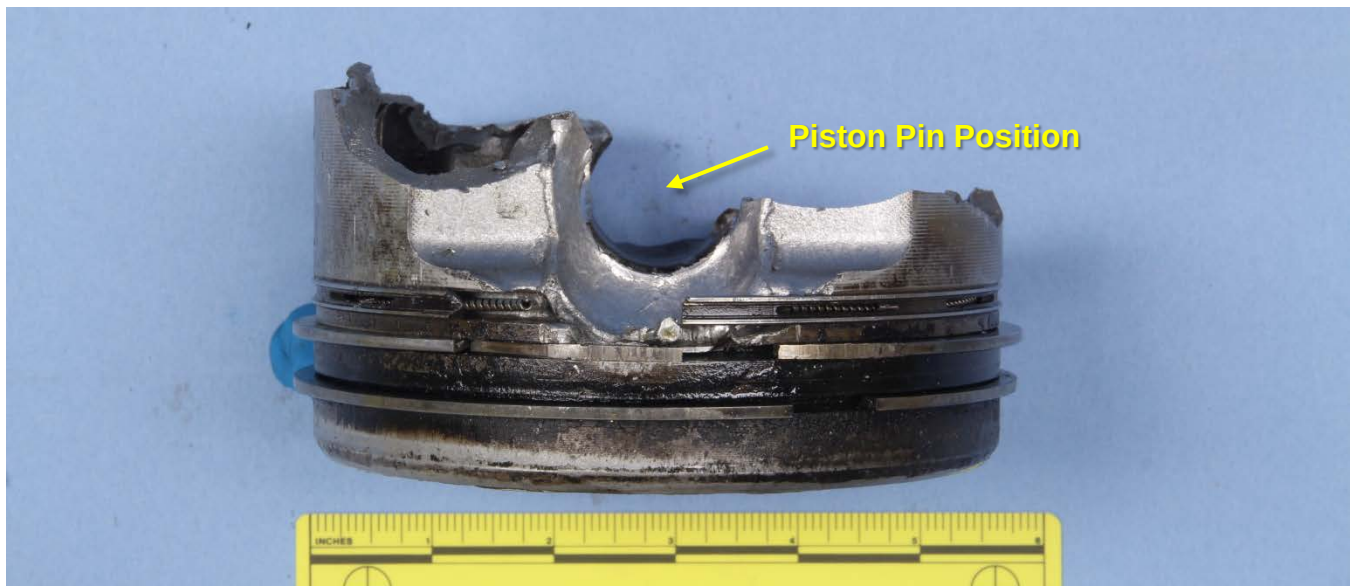
Figure 3 – The piston crown, as viewed from the side along the piston position, as received.
