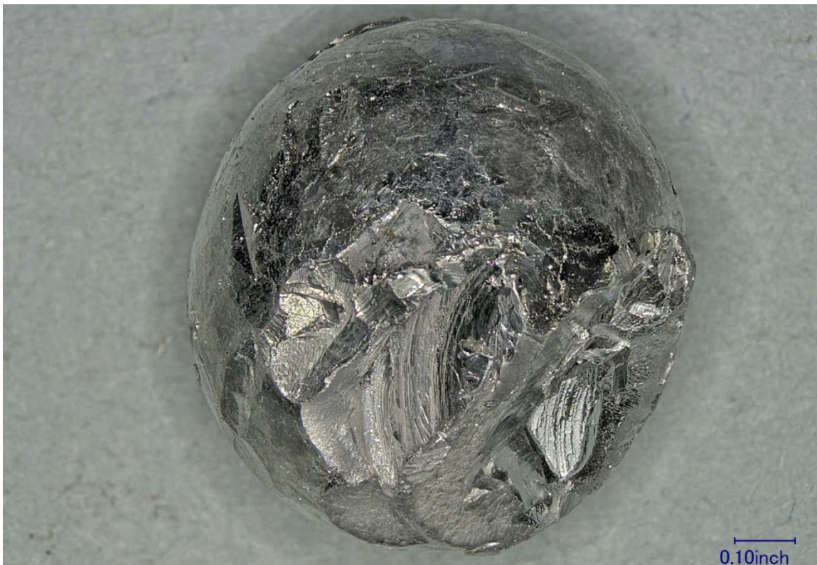
Figure 15 – The spherical separated pin piece, showing impressions from collisions.
