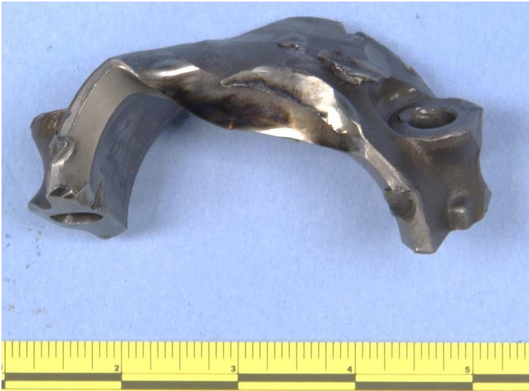
Figure 6 – The connecting rod cap, showing batter and impact damage.
