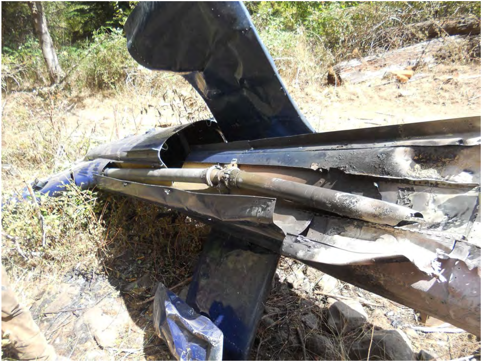
Photo 7 – Tail rotor drive shaft (photo provided by AvTech)
