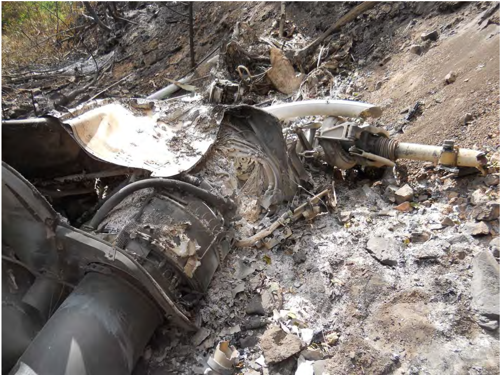
Photo 5 – Engine and main rotor mast (photo provided by AvTech)
