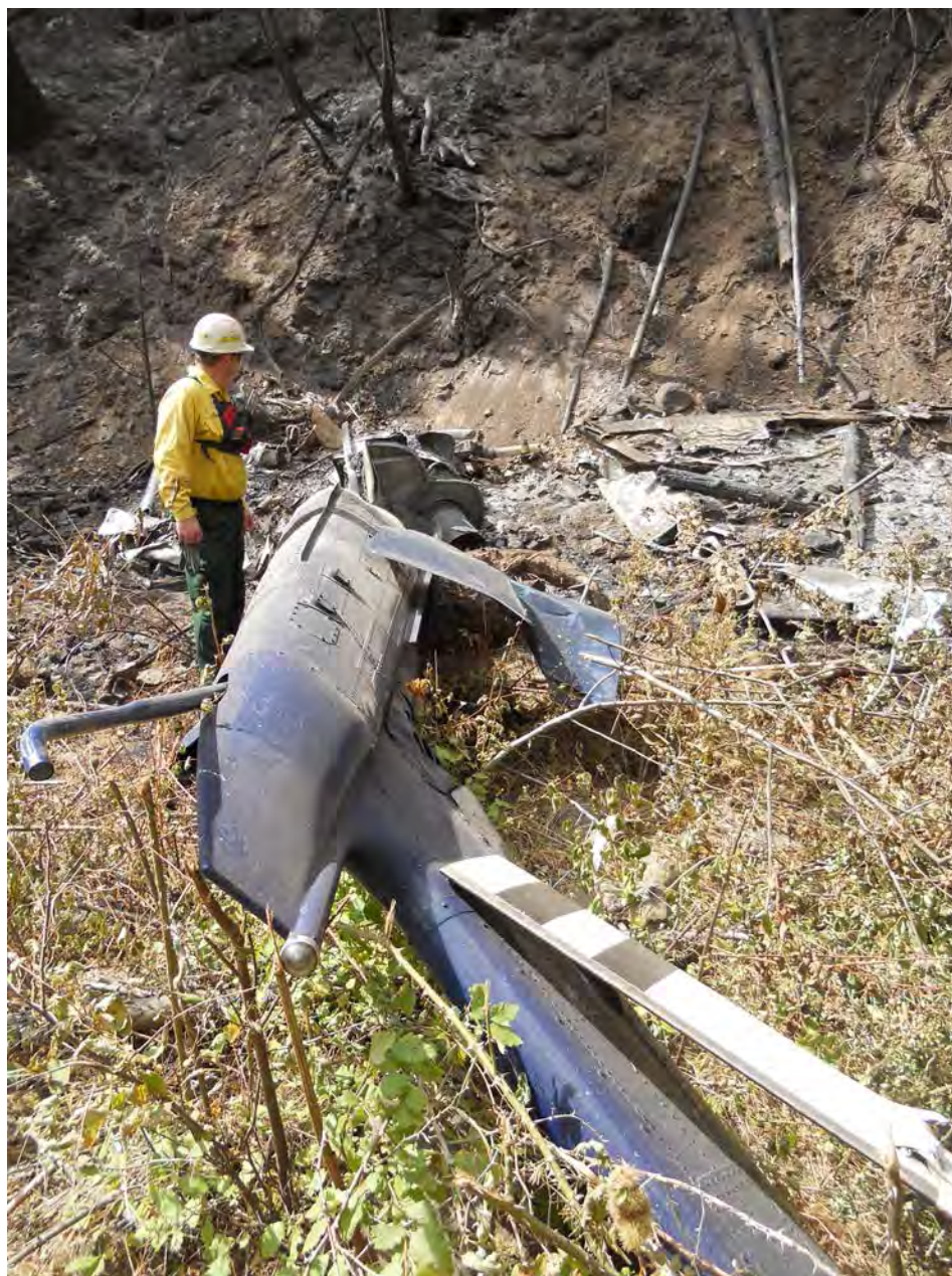
Photo 4 – Tail boom with tail rotor blade (photo provided by AvTech)
