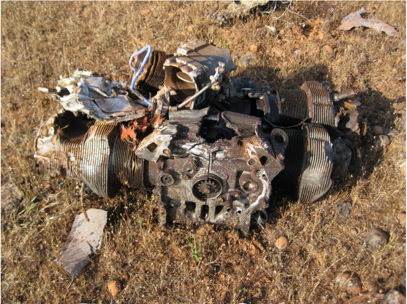
Photo 2 - View of Engine (Courtesy of the FAA)
