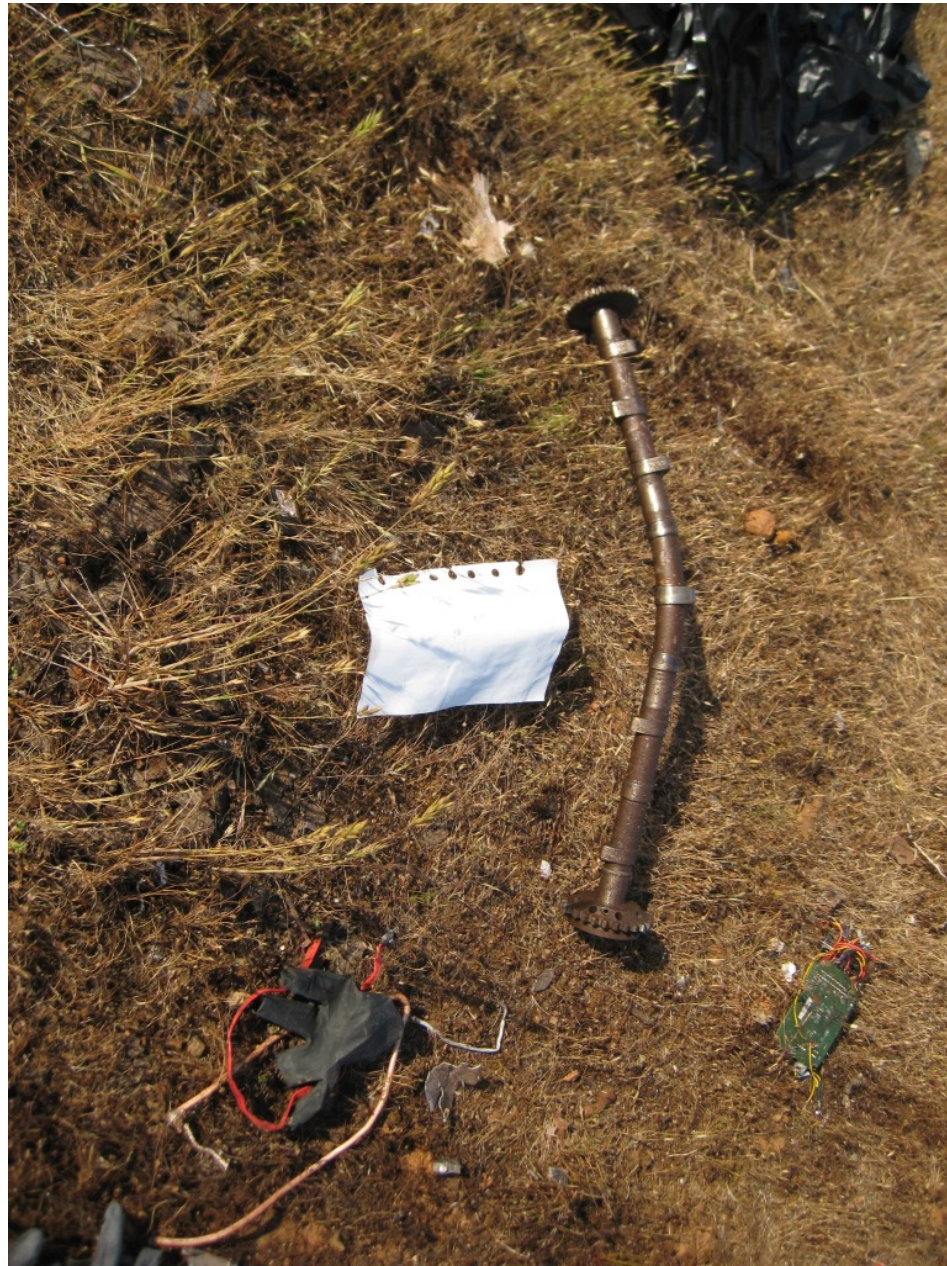
Photo 3 - Photo of the Camshaft (Courtesy of the FAA)
