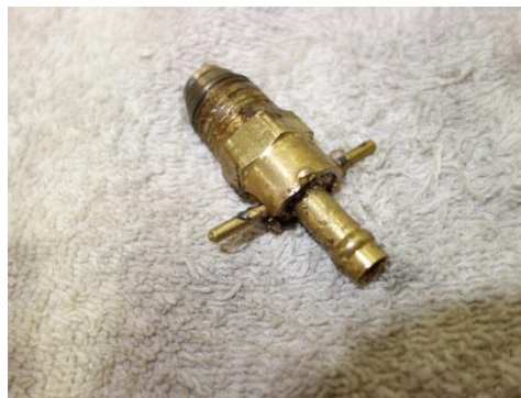
Figure 2: Installed oil quick drain valve
