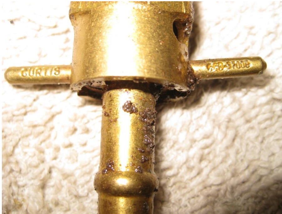
Figure 3: Installed Oil Quick Drain Valve with part number
