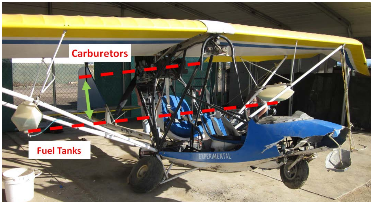
Photo 16 - Fuel Tank Position Relative to Carburetors
