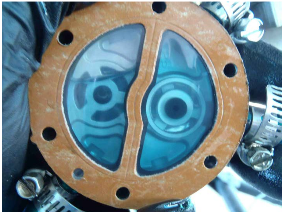
Photo 5 - Engine Driven Fuel Pump
