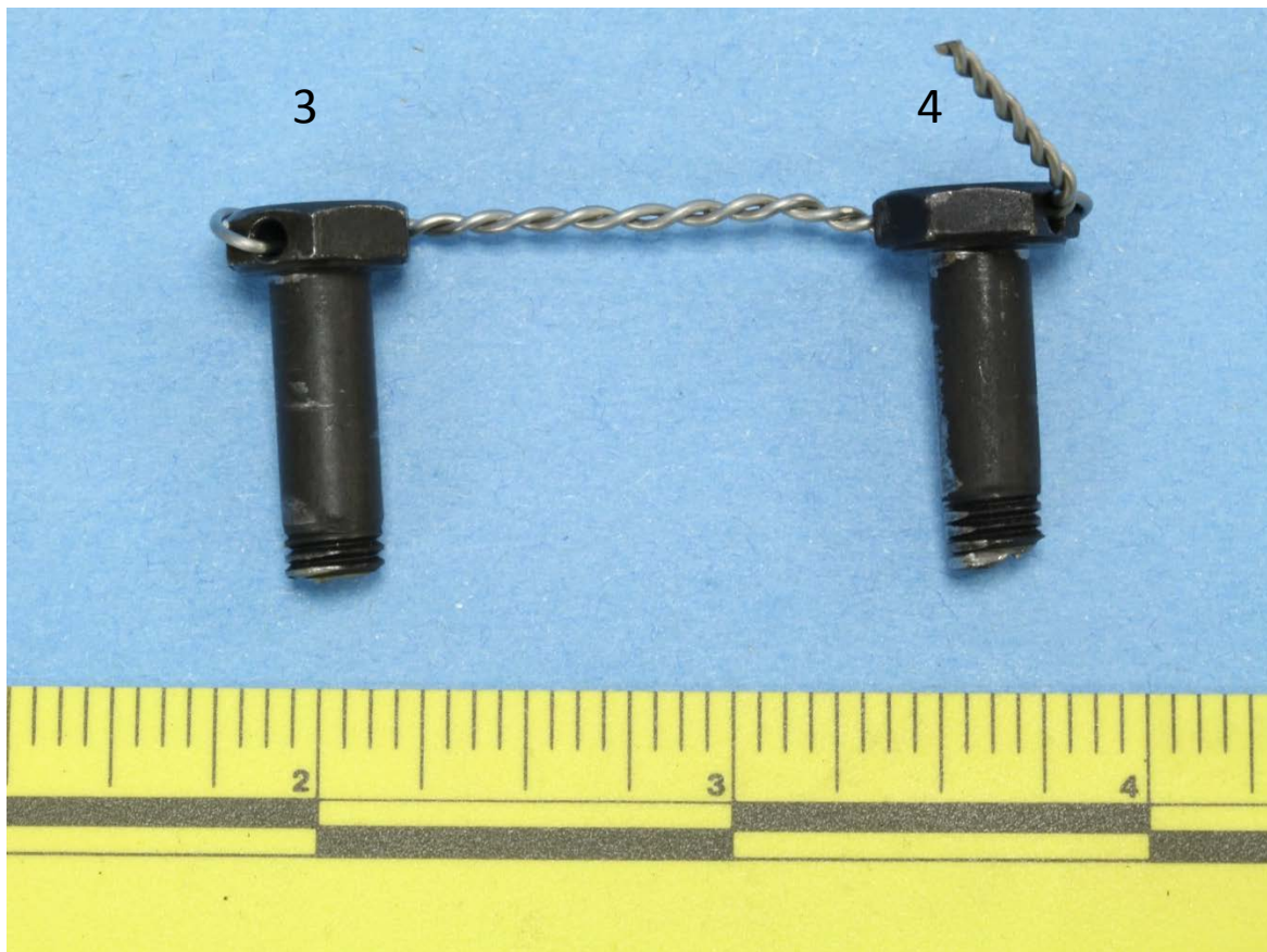
Figure 2: Two gear bolts without plastic deformation and exhibiting flat fracture surfaces.
