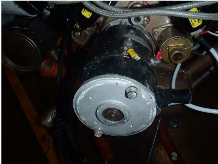
Figure 33 - photo of generator
